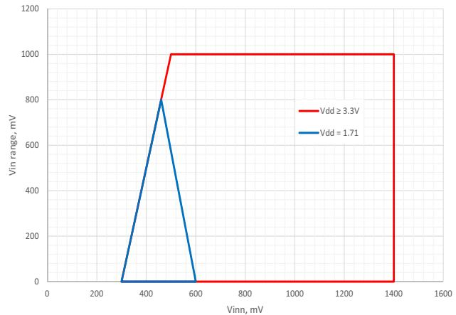
**Figure 32. PGA Input Vind Range Multiplied by Gain vs. Vinn, Pseudo-Differential Mode, G = 4**
