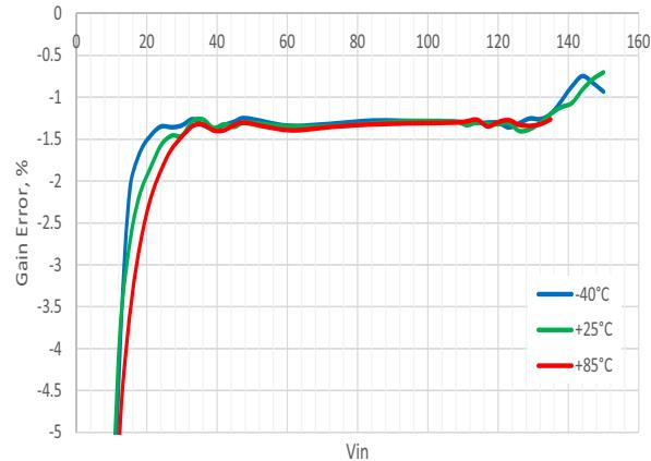
**Figure 24. Typical PGA Gain Error vs. Vin, Single-Ended Mode, G = 8, VDD = 5.5 V**
