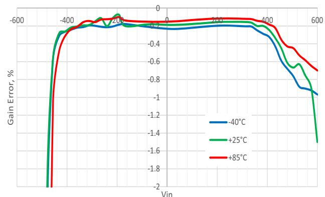
**Figure 26. Typical PGA Gain Error vs. Vin, Differential Mode, G = 1, VDD = 1.71 V**
