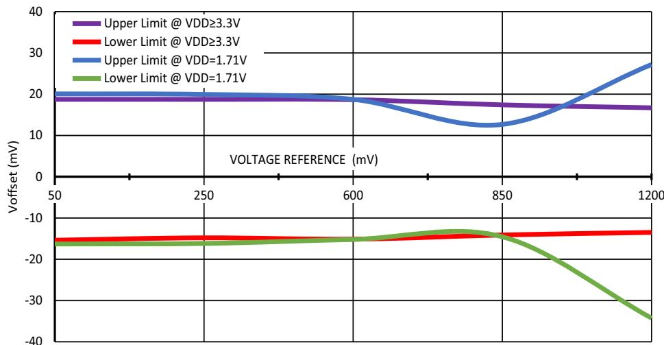
**Figure 51. Buffer Input Voltage Offset vs. Voltage Reference at  $T = (-40 \dots +85)^\circ\text{C}$ ,
