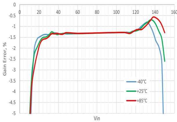
**Figure 23. Typical PGA Gain Error vs. Vin, Single-Ended Mode, G = 8, VDD = 1.71 V**
