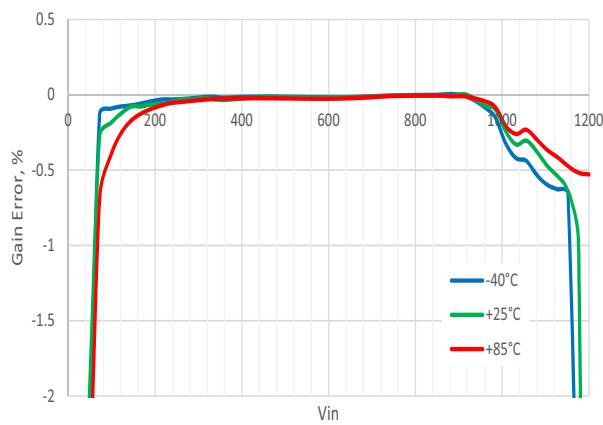
Figure 21. Typical PGA Gain Error vs. Vin, Single-Ended Mode, G = 1, VDD = 1.71 V
