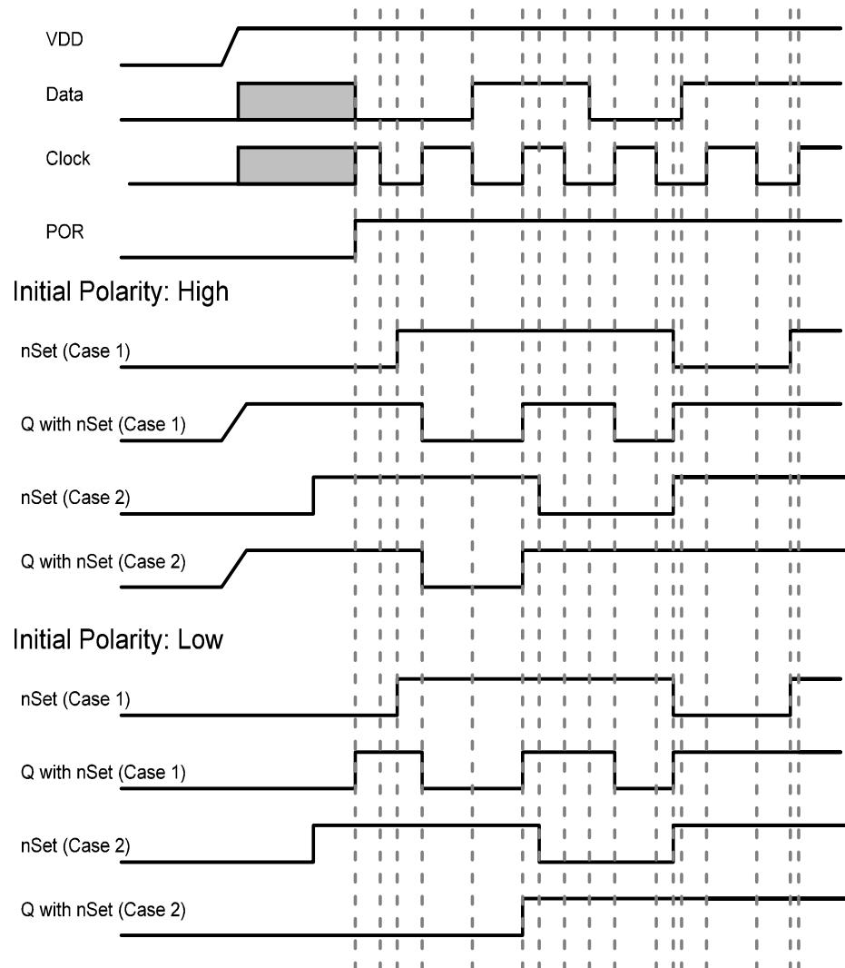
Figure 76. DFF Polarity Operations with nSet
