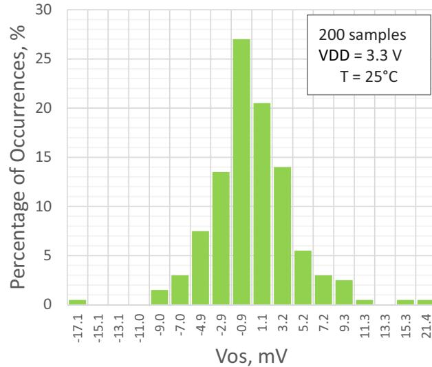
Figure 16. PGA Input Offset Distribution, Single-Ended Mode,  $G = 0.5$
