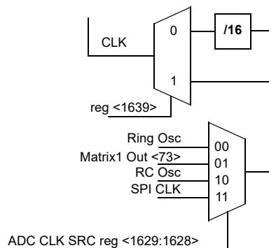
Figure 38. ADC Clock Source
