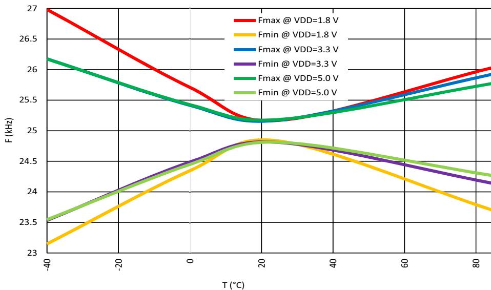
Figure 121. RC Oscillator Frequency vs. Temperature, RC OSC = 25 kHz
