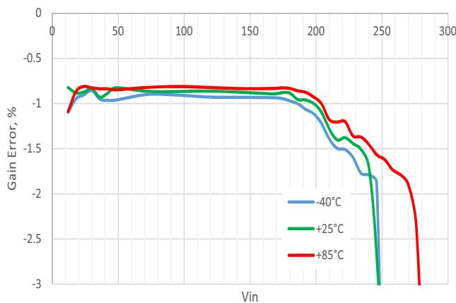
**Figure 35. Typical PGA Gain Error vs. Vin,
