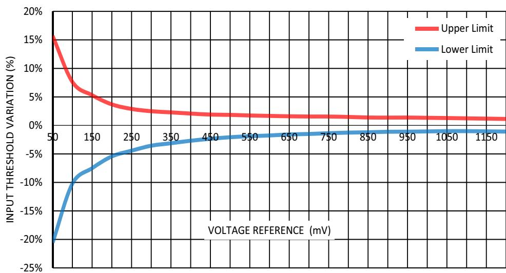
**Figure 54. Input Threshold Variation (including  $V_{\text{ref}}$  variation, ACMP offset) vs.
