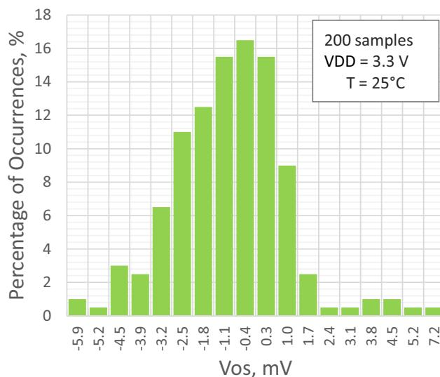
Figure 18. PGA Input Offset Distribution, Single-Ended Mode,  $G = 2$
