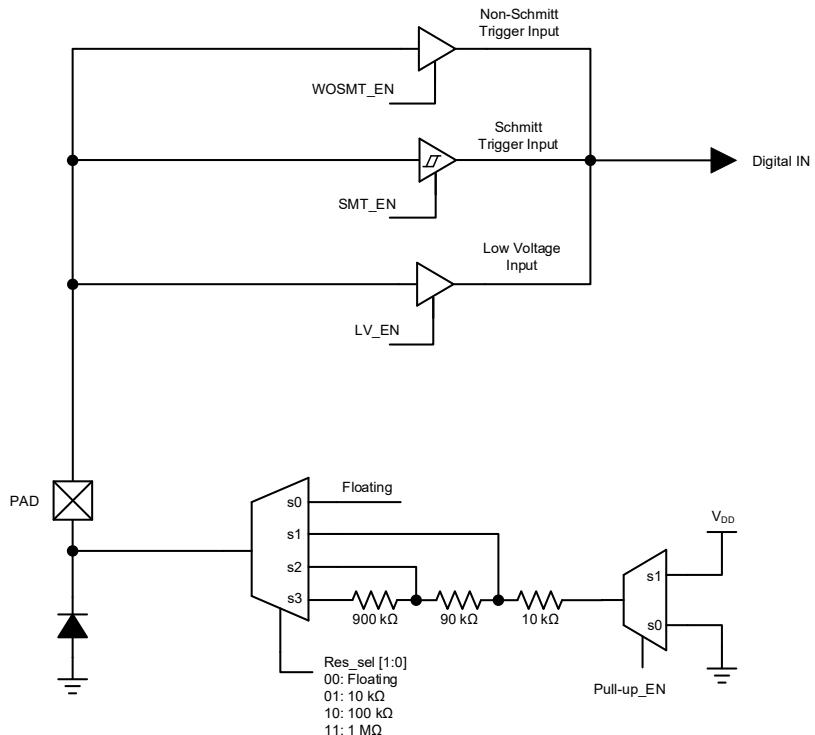
Figure 2. PIN 2 GPI IO Structure Diagram
