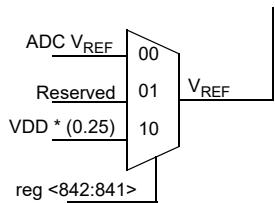
Figure 37. ADC Reference Voltage
