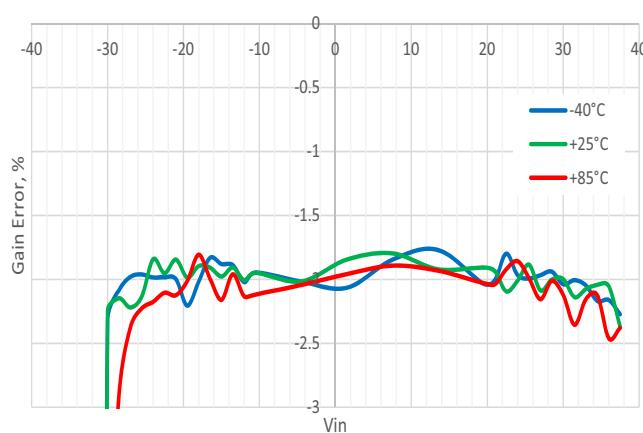
**Figure 29.** Typical PGA Gain Error vs. Vin, Differential Mode,  $G = 16$ ,  $VDD = 5.5$  V
