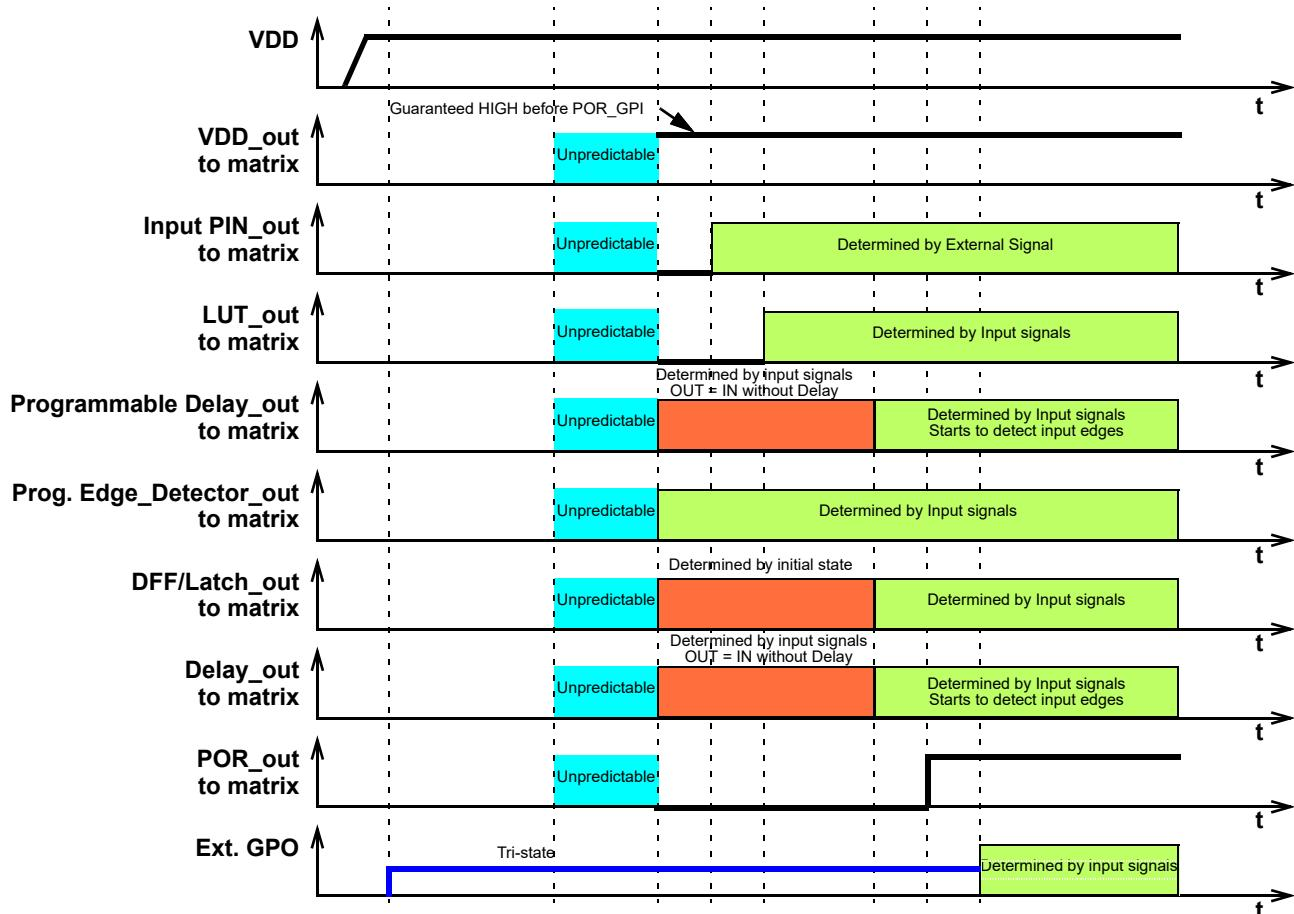
Figure 125. Internal Macrocell States during POR sequence
