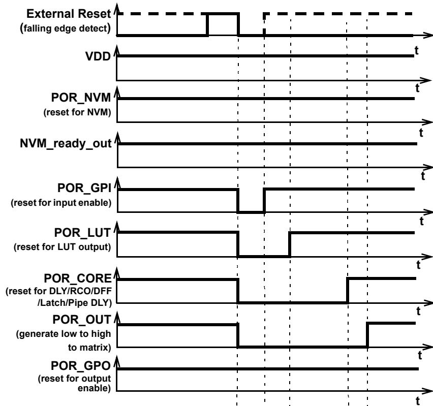
Figure 129. External reset sequence (Falling edge detect)
