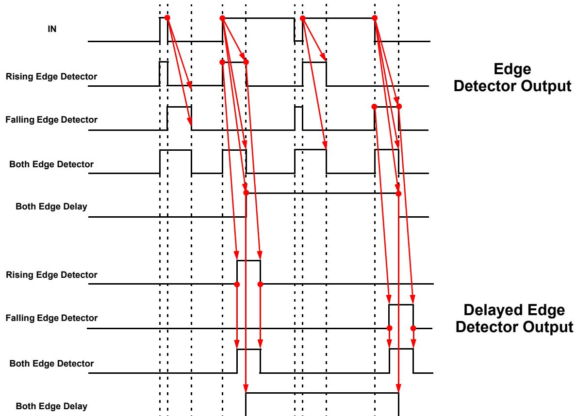
Figure 112. Glitch Filtering for Edge Detector Output
