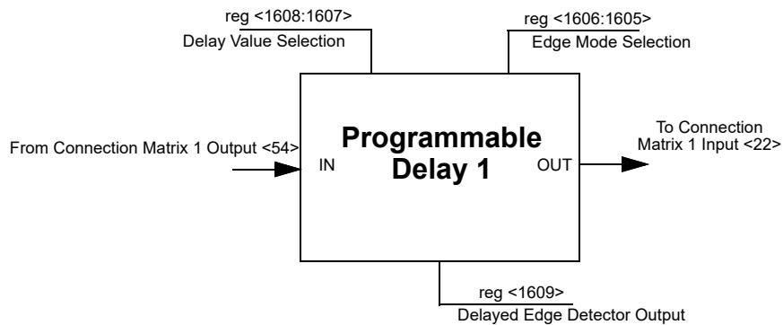
**Figure 109. Programmable Delay**
