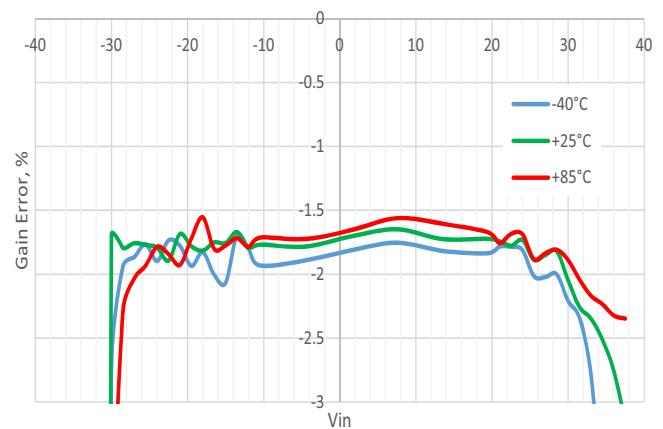
**Figure 28.** Typical PGA Gain Error vs. Vin, Differential Mode,  $G = 16$ ,  $VDD = 1.71$  V
