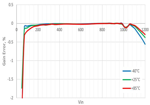
Figure 22. Typical PGA Gain Error vs. Vin, Single-Ended Mode, G = 1, VDD = 5.5 V
