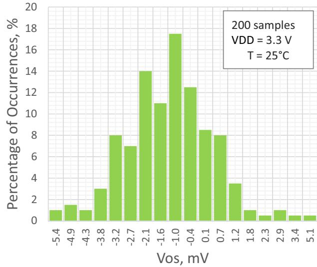
Figure 20. PGA Input Offset Distribution, Single-Ended Mode, G = 8
