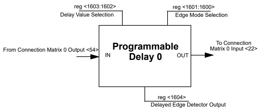
**Figure 108. Programmable Delay**
