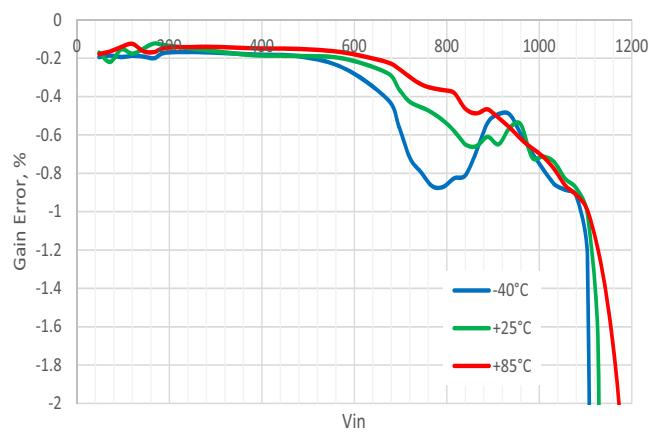
**Figure 33. Typical PGA Gain Error vs. Vin, Pseudo-Differential Mode, G = 1, VDD = 2.0 V**
