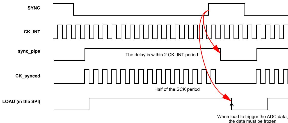
Figure 104. Timing Diagram showing SPI Clock synchronization
