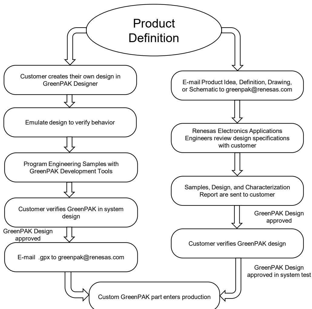
Figure 1. Steps to create a custom GreenPAK device
