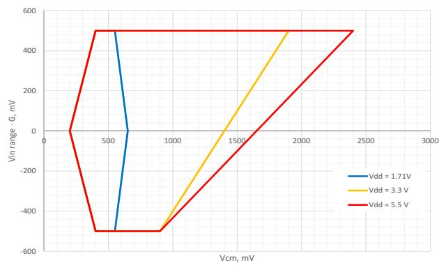
**Figure 25. PGA Input Vind Range Multiplied by Gain vs. Vcm, Differential Mode**
