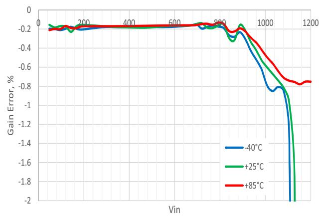
**Figure 34. Typical PGA Gain Error vs. Vin, Pseudo-Differential Mode, G = 1, VDD = 5.5 V**
