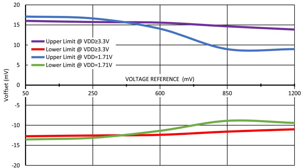
**Figure 53. Buffer Input Voltage Offset vs. Voltage Reference at  $T = (-40.... +85)^\circ\text{C}$ ,
