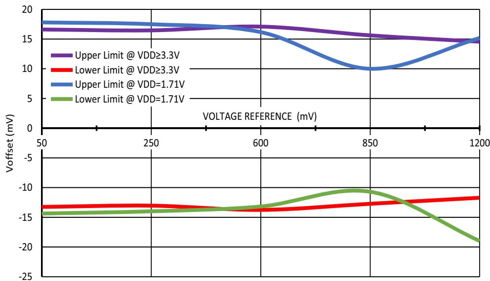
**Figure 52. Buffer Input Voltage Offset vs. Voltage Reference at  $T = (-40 \dots +85)^\circ\text{C}$ ,
