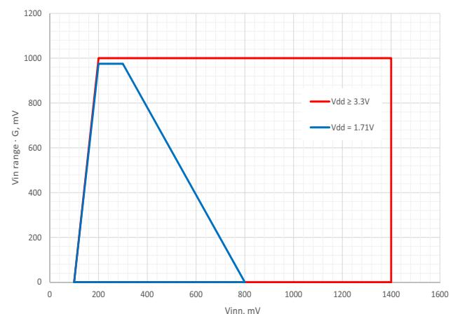
**Figure 30.** PGA Input Vin Range Multiplied by Gain vs. Vinn, Pseudo-Differential Mode,  $G = 1$
