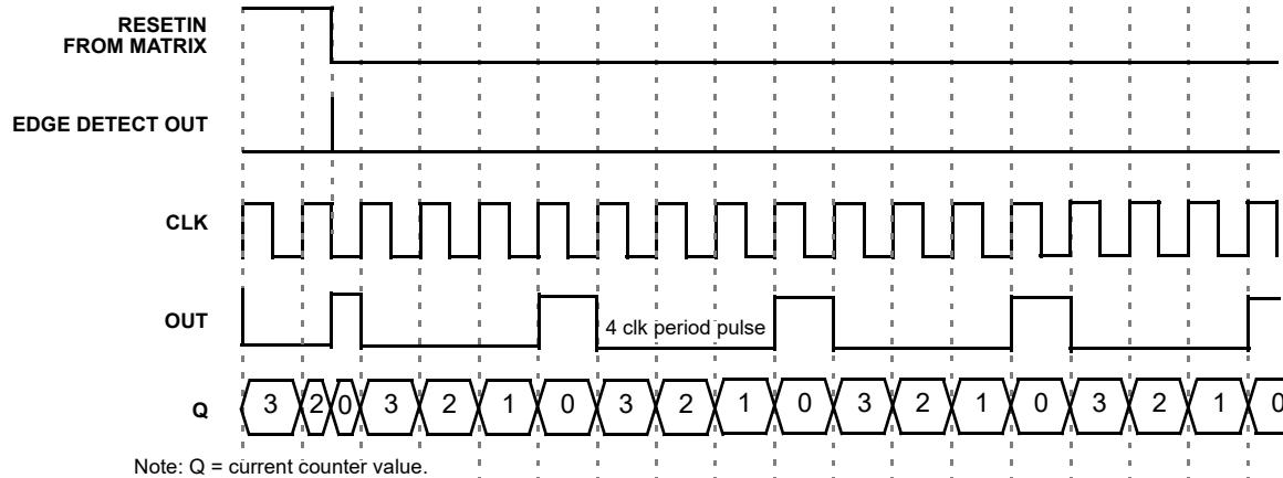
Figure 90. Timing (reset falling edge mode, oscillator is forced on) for count data = 3
