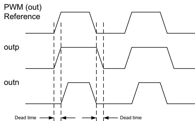
Figure 100. PWM Dead Band Control Timing Diagram
