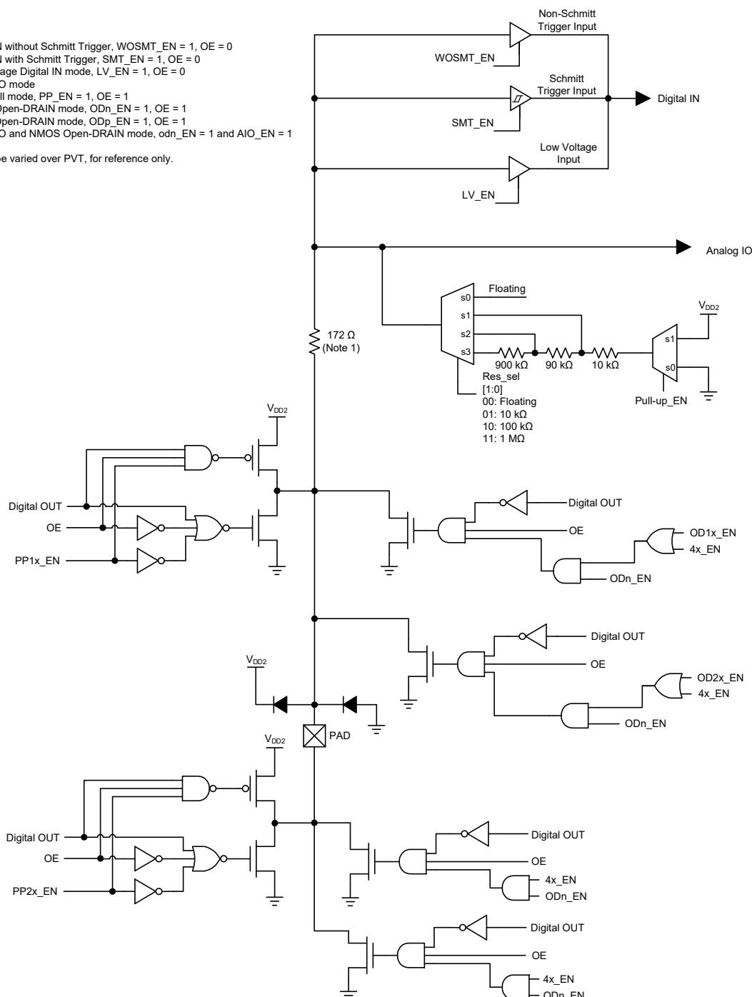
Figure 8. Matrix OE IO 4x Drive Structure Diagram
