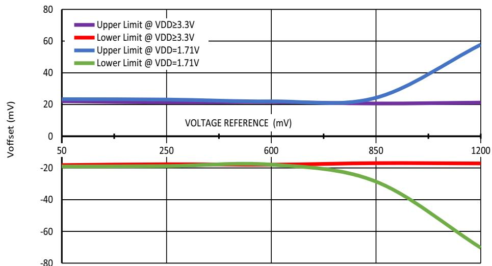
**Figure 50. Buffer Input Voltage Offset vs. Voltage Reference at T = (-40.... +85)°C,
