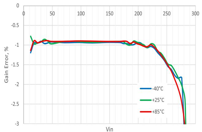
**Figure 36. Typical PGA Gain Error vs. Vin,
