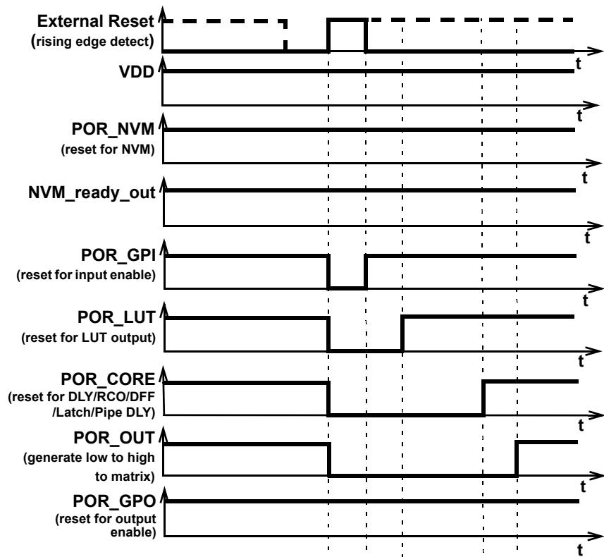
Figure 128. External reset sequence (Rising edge detect)
