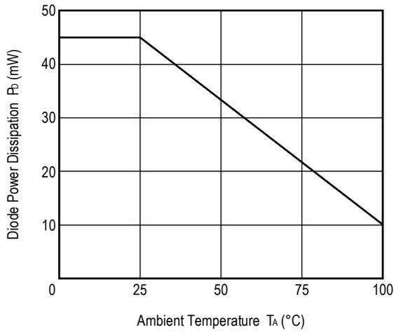
DETECTOR POWER DISSIPATION vs. AMBIENT TEMPERATURE
