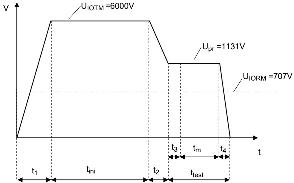
$t_1, t_2 = 1 \text{ to } 10 \text{ sec}$
