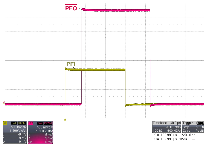
FIGURE 16. ISL7x6xRH PFI TO PFO RESPONSE
