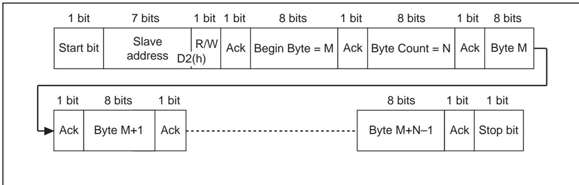
**Renasas clock generator I<sup>2</sup>C Serial Interface Operation (cont.)**
