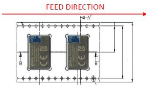
Figure 15: Component Direction
