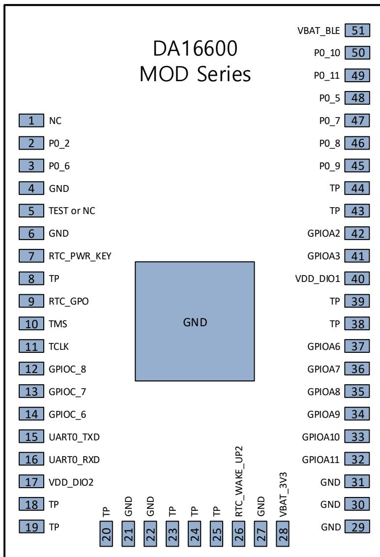
Figure 2: DA16600MOD 51 Pinout Diagram (Top View)
