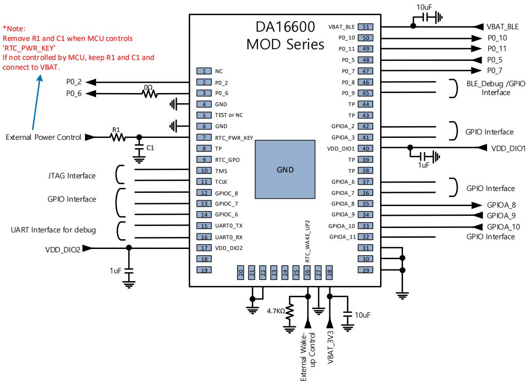
Figure 6: Application Schematic
