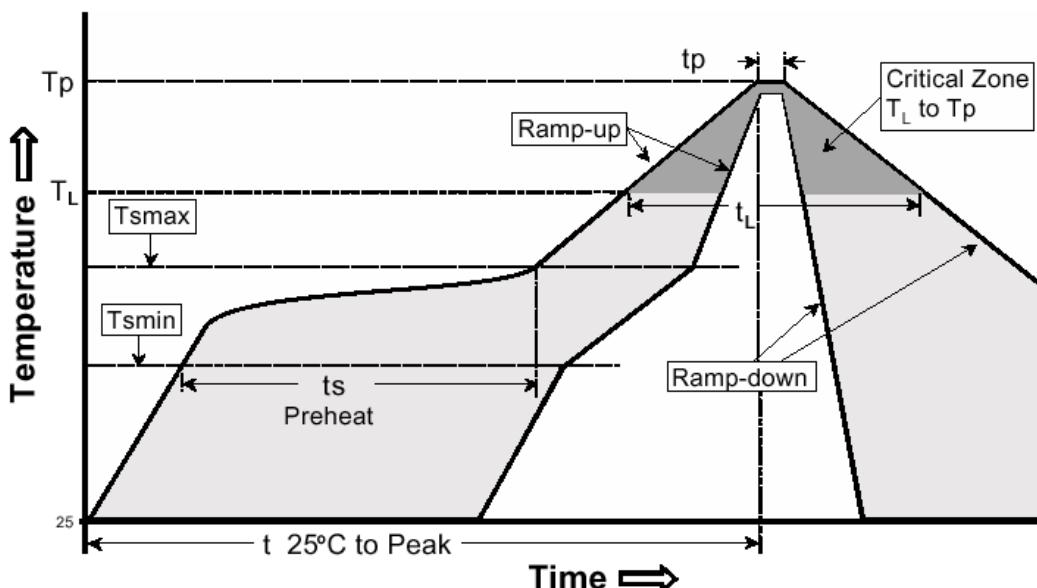
Figure 13: Reflow Condition
