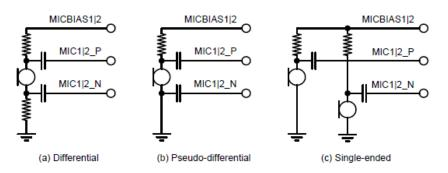
Figure 7: Connection of Analog Microphones
