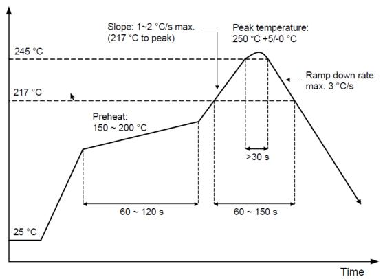
Figure 5: Reflow Profile (Lead-Free)
