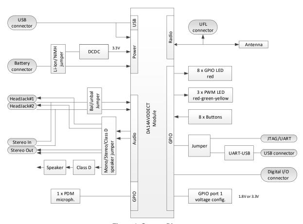
Figure 1: System Diagram
