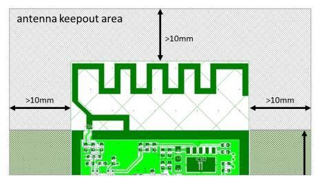
NB: application PCB should not extend beneath antenna area
