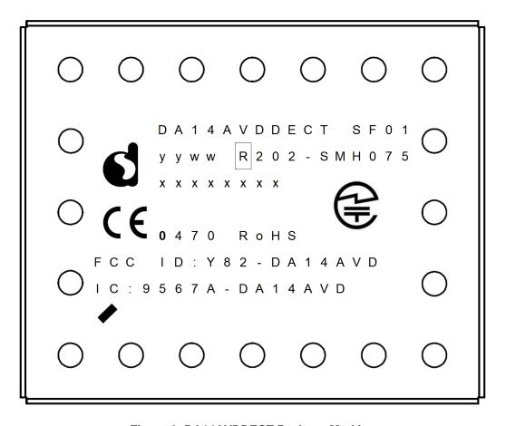
Figure 6: DA14AVDDECT Package Marking
