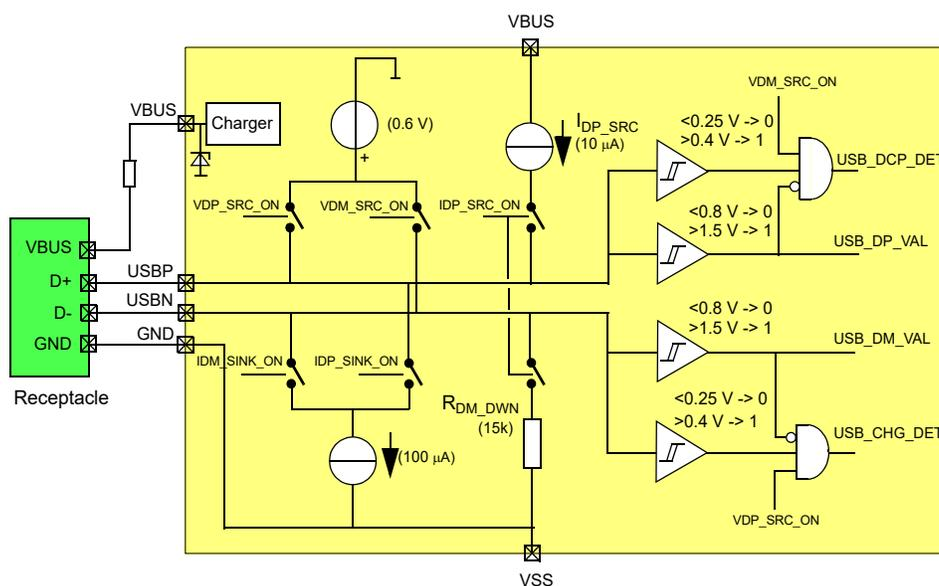
Figure 29: USB charger detection block diagram (BC1.2)
