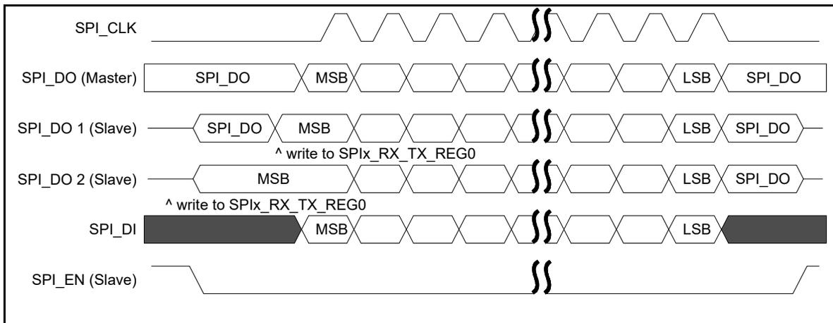
Figure 80: SPI Master/slave, mode 0: SPI\_POL=0 and SPI\_PHA=0
