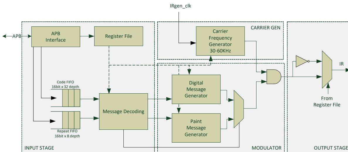
Figure 96: InfraRed Generator Block Diagram
