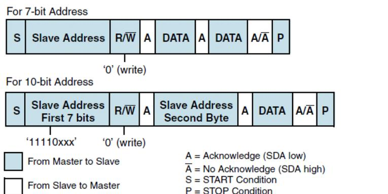
Figure 91: Master-Transmitter Protocol
