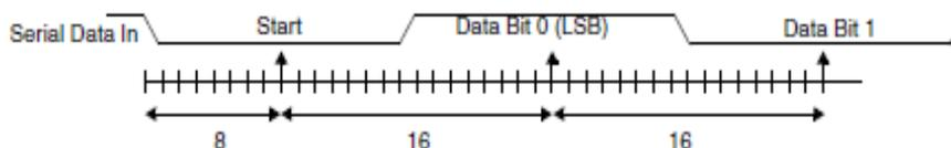
Figure 75: Receiver Serial Data Sample Points
