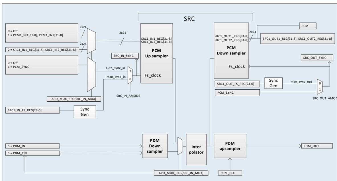
Figure 62: Sample rate Converter block diagram
