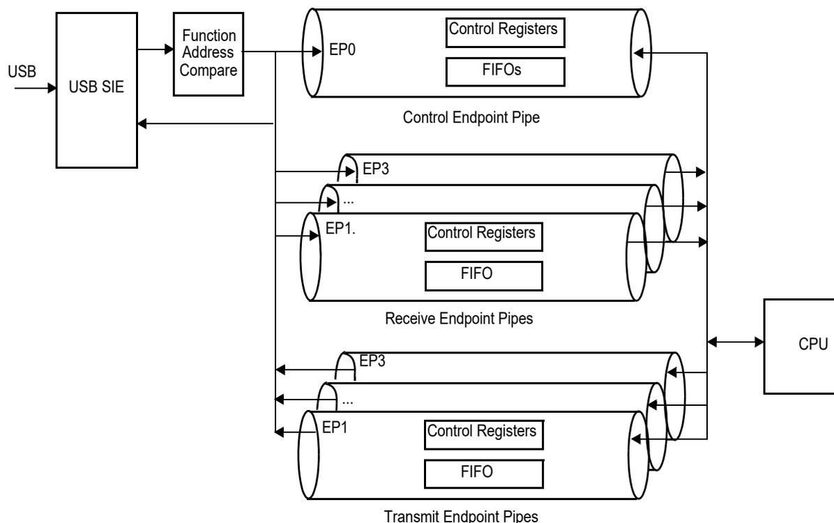
Figure 111: Endpoint Operation
