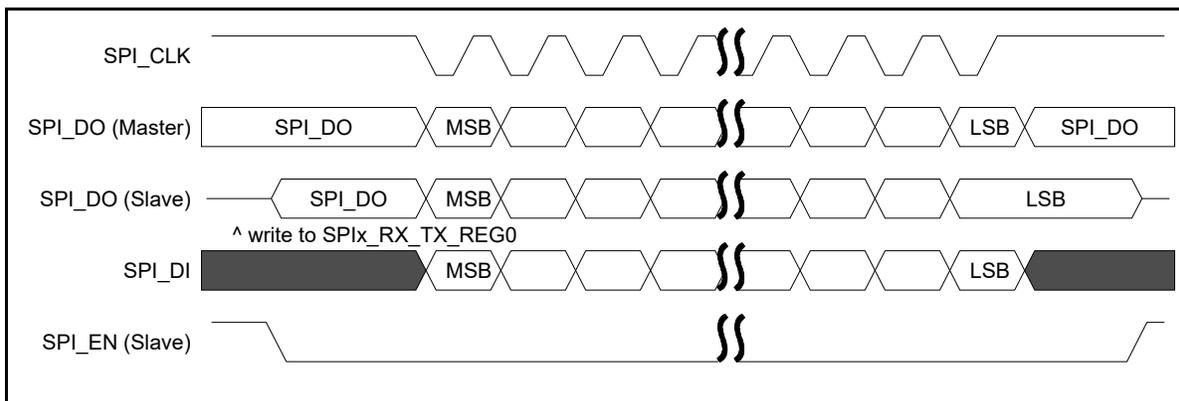
Figure 83: SPI Master/slave, mode 3: SPI\_POL=1 and SPI\_PHA=1
