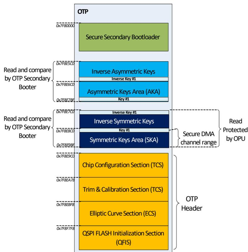
**Figure 9: OTP layout with security features enabled**
