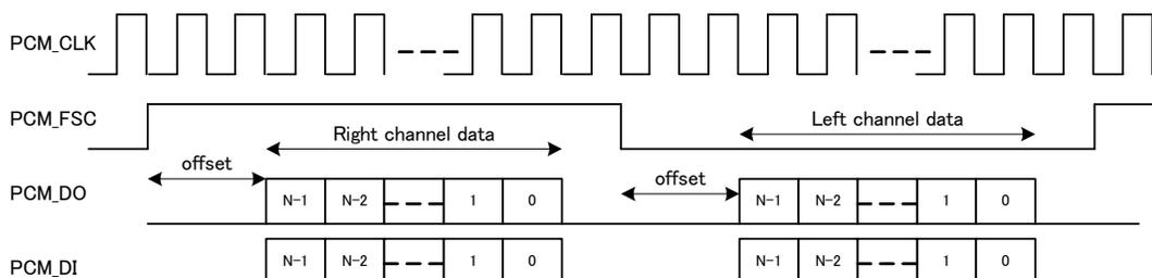
Figure 71: I2S TDM mode (left justified mode)
