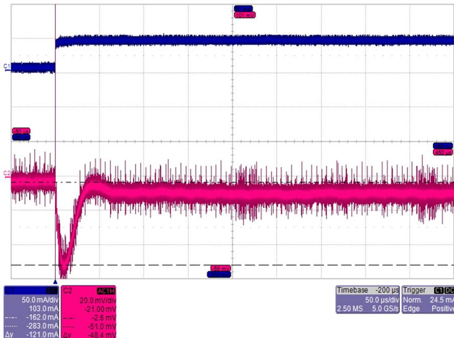
Figure 19: LDO\_RADIO loadstep 0 to 35mA (Cload=4.7uF, Vout=1.45V)
