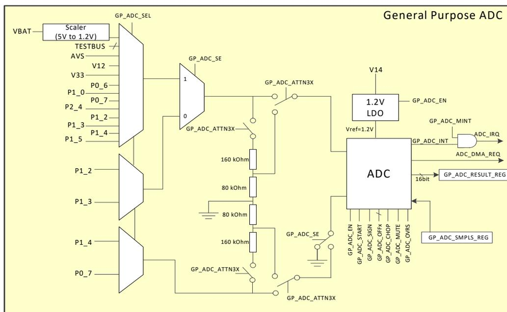
**Figure 60: Block diagram of the General Purpose ADC**
