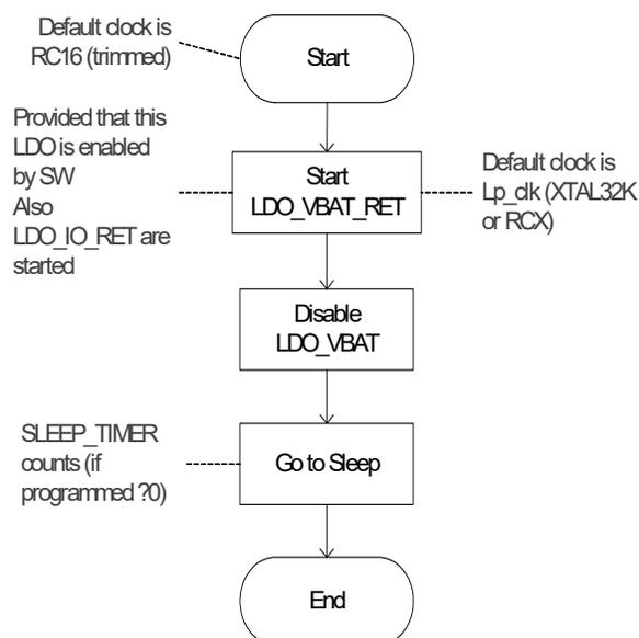
**Figure 5: Go to Sleep FSM flow diagram**
