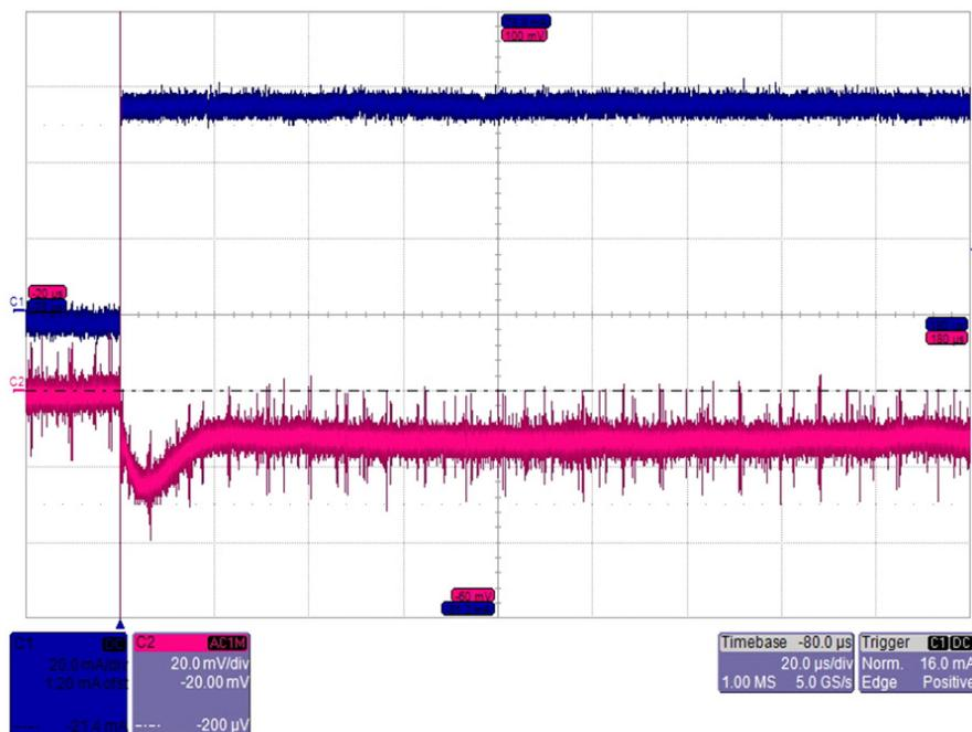
Figure 20: LDO\_IO loadstep 0 to 60mA (Cload=10uF)
