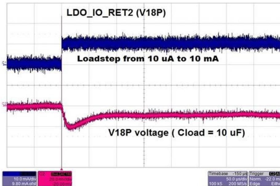
Figure 21: LDO\_VBAT\_RET loadstep 0 to 10mA (Cload=10uF)
