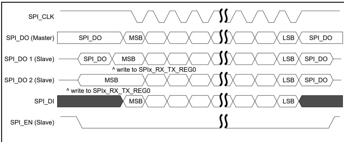
Figure 82: SPI Master/Slave, mode 2: SPI\_POL=1 and SPI\_PHA=0
