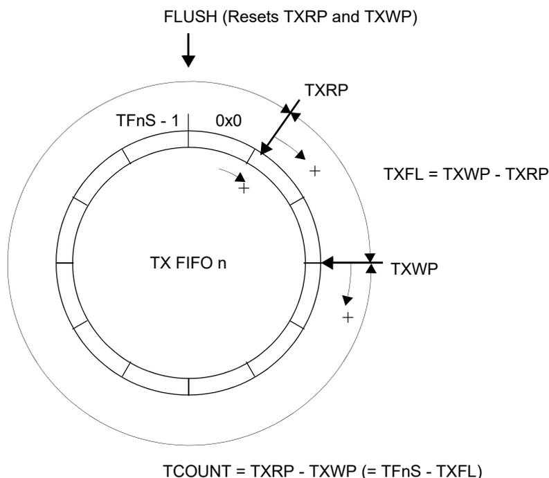
Figure 115: Tx FIFO operation
