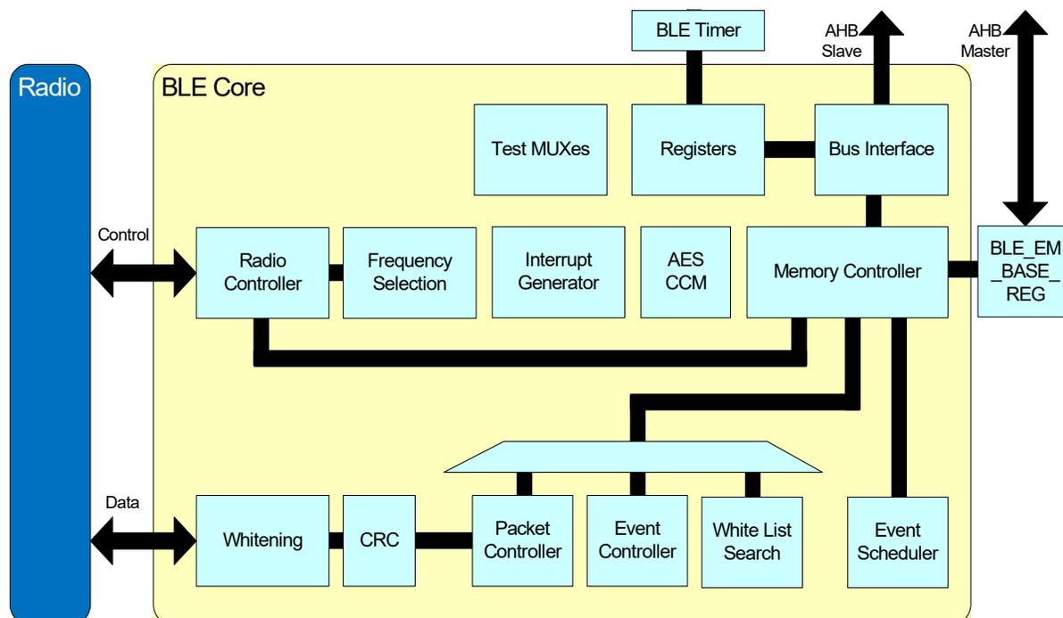
Figure 121: BLE Core Block Diagram
