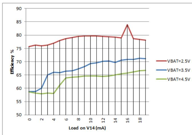
**Figure 16: 1.4V rail DCDC efficiency vs load**
