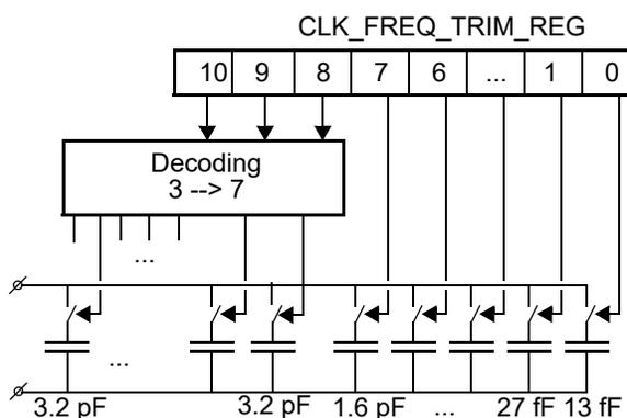
Figure 36: Frequency trimming
