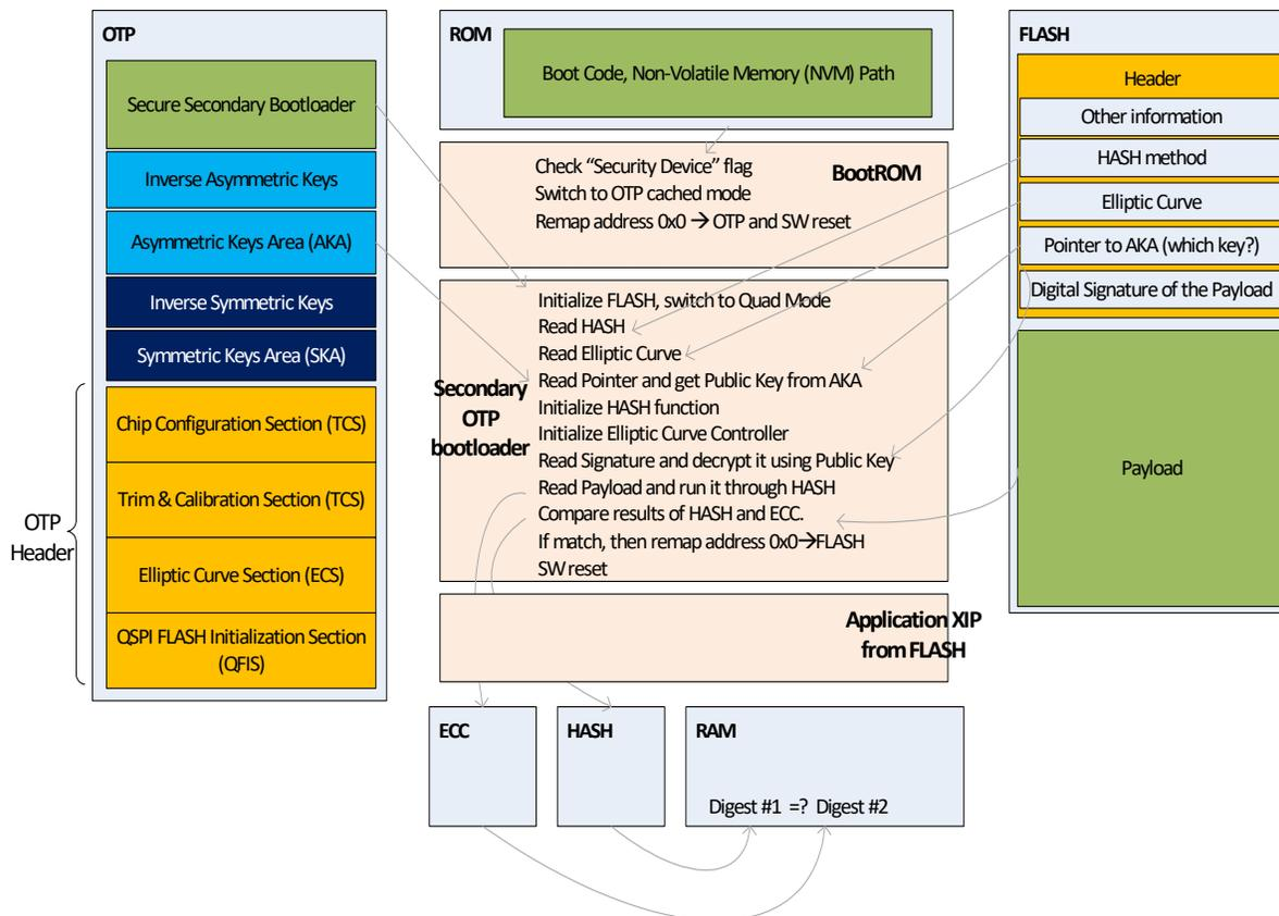
Figure 11: CPU steps for a Secure Boot process
