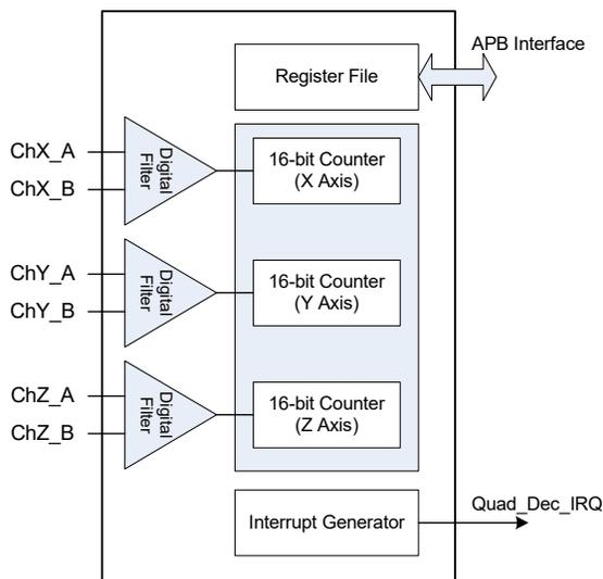
**Figure 98: Block diagram of the Quadrature Decoder**
