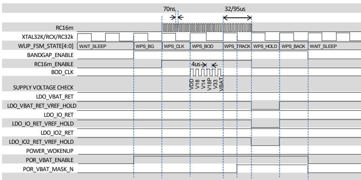
Figure 33: SLEEP\_TIMER based wake up timing for BOD
