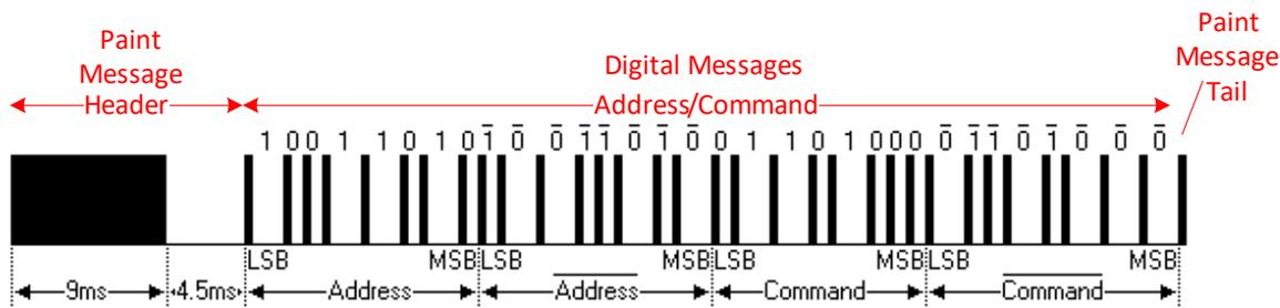
Figure 97: Paint/Digital messages on a NEC based example
