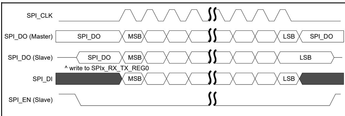
Figure 81: SPI Master/Slave, mode 1: SPI\_POL=0 and SPI\_PHA=1
