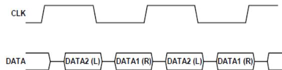
Figure 10. Stereo PDM Format
