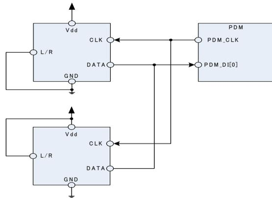
Figure 63: PDM with dual mic interface
