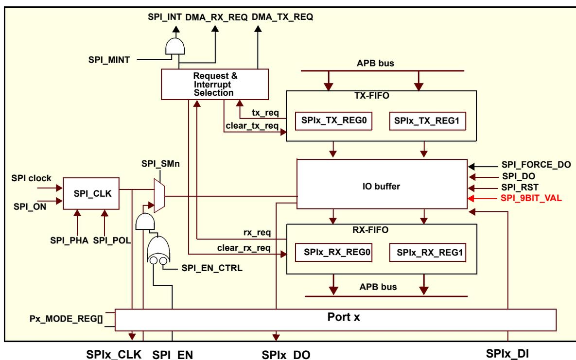
Figure 79: SPI block diagram
