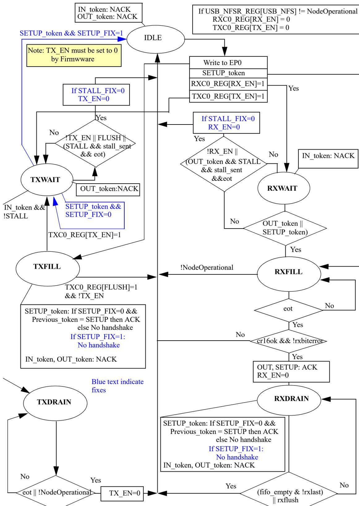
Figure 114: Endpoint 0 Operation
