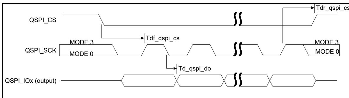
Figure 49: QSPI output Timing
