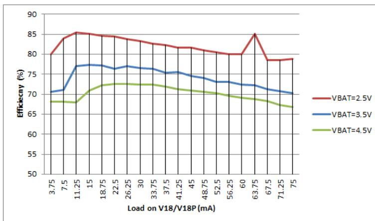
Figure 14: 1.8V rails DCDC efficiency vs load
