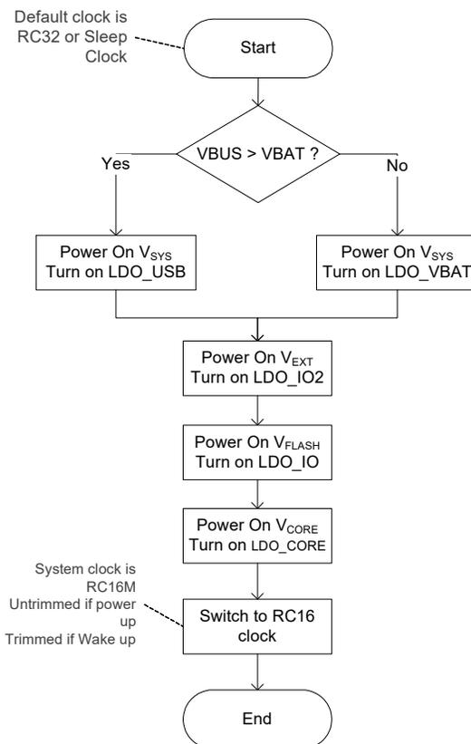
Figure 4: Power Up / Wake Up FSM
