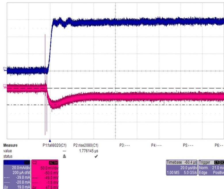
Figure 18: LDO\_CORE loadstep 0 to 58mA (Cload=4.7uF)
