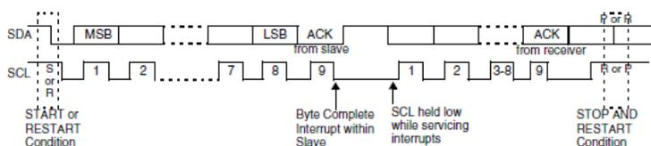
**Figure 87: Data transfer on the I2C Bus**
