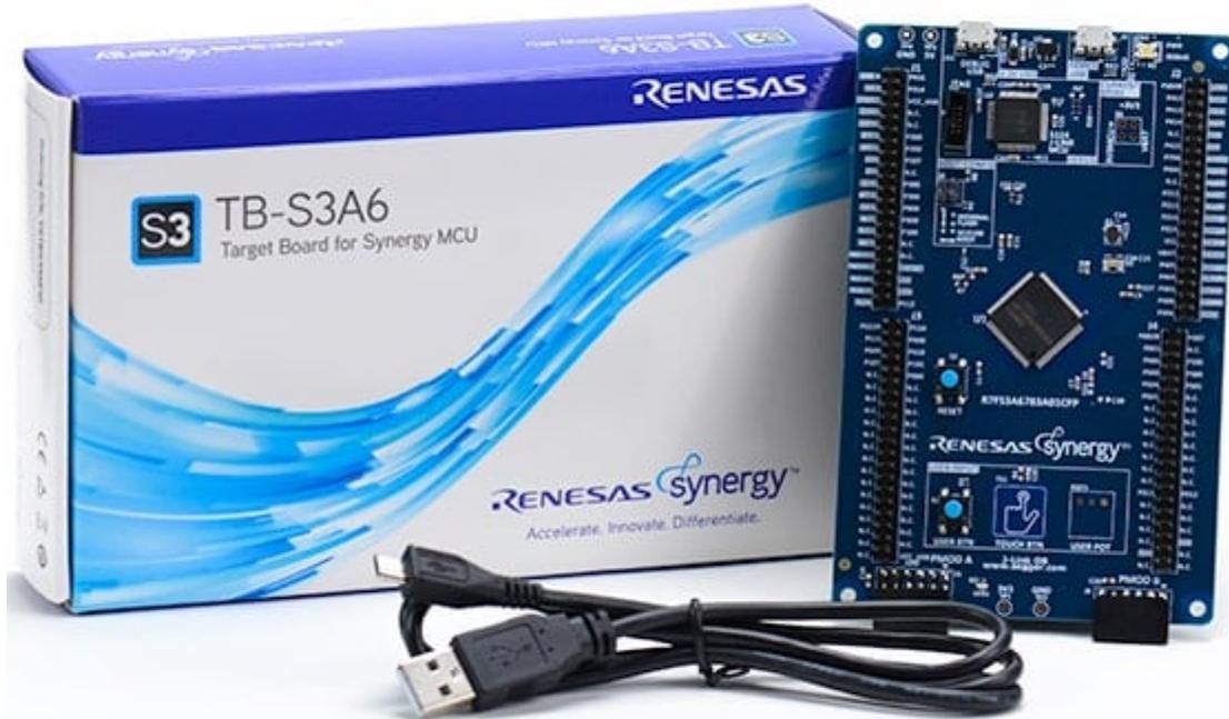
**Figure 14:** Synergy Target Board TB-S3A6
