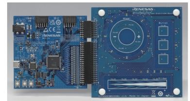
Capacitive Touch Evaluation System for RA4L1
