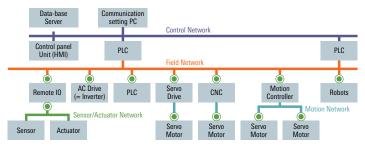
Target products: PLC, remote IO, CNC, AC drive (inverter), robot, servo drive, servo motor
