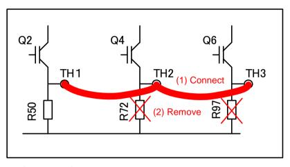
Figure 1-3 Change 3-shunt to 1-shunt
