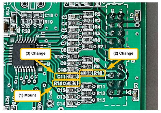
Figure 1-6 Modification example on the CPU card.
