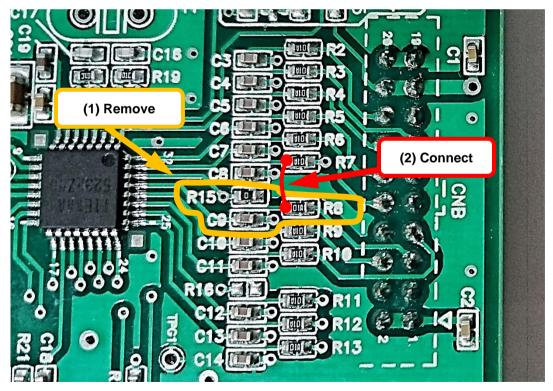
Figure 1-2 Modification example on the CPU card.
