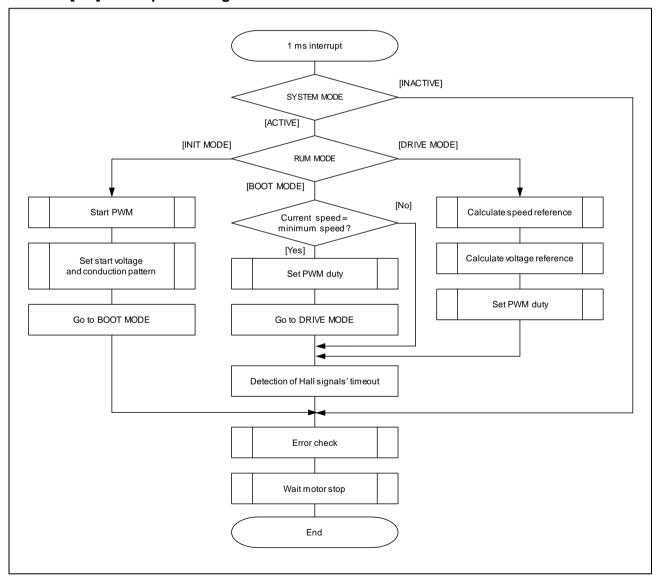
Figure 3-9 1 [ms] Interrupt Handling
