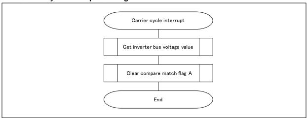
Figure 3-8 50[μs] Cycle Interrupt Handling (120-degree Control using Hall sensors)
