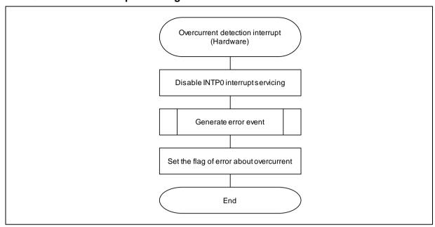
Figure 3-10 Over Current Detection Interrupt Handling (INTP0)
