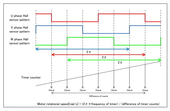
Figure 3-1 Method of Calculation for the Rotational Speed
