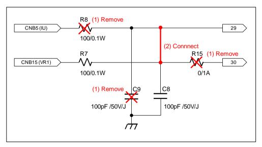
Figure 1-1 Modification of the CPU Card
