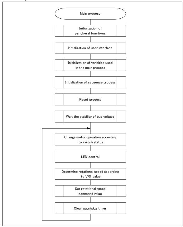
Figure 3-7 Main Process Flowchart
