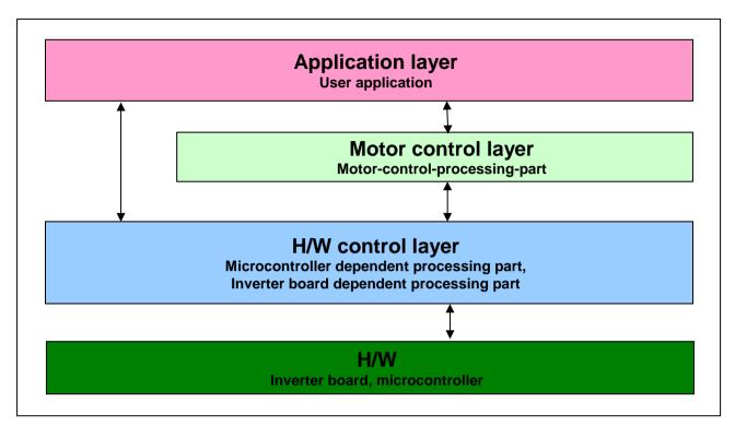
**Figure 2-2 Module Configuration**
