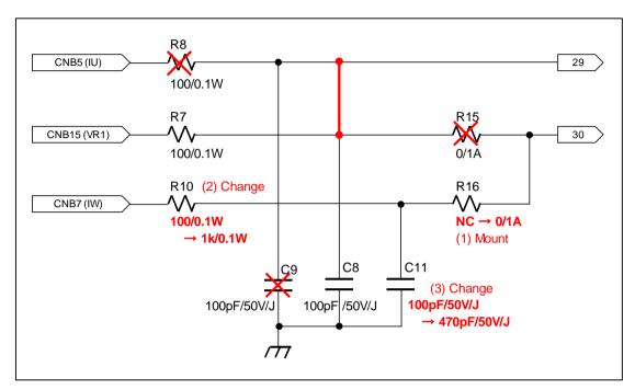
Figure 1-5 Modification of the CPU Card
