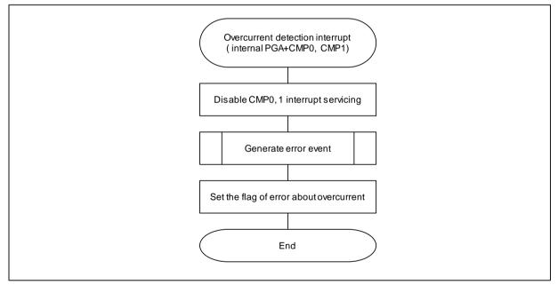
Figure 3-11 Over Current Detection Interrupt Handling (PGA+CMP0, CMP1)
