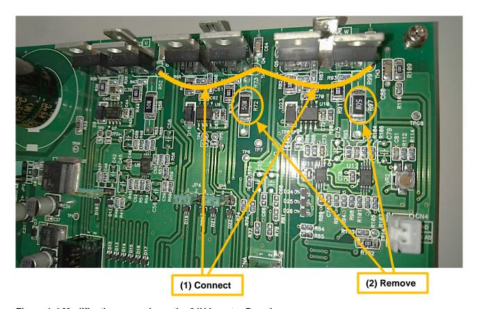
Figure 1-4 Modification example on the 24V Inverter Board
