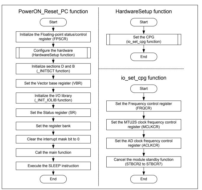
Figure 1 Flow Charts of Functions (PowerON\_Reset\_PC, HardwareSetup, and io\_set\_cpg)
