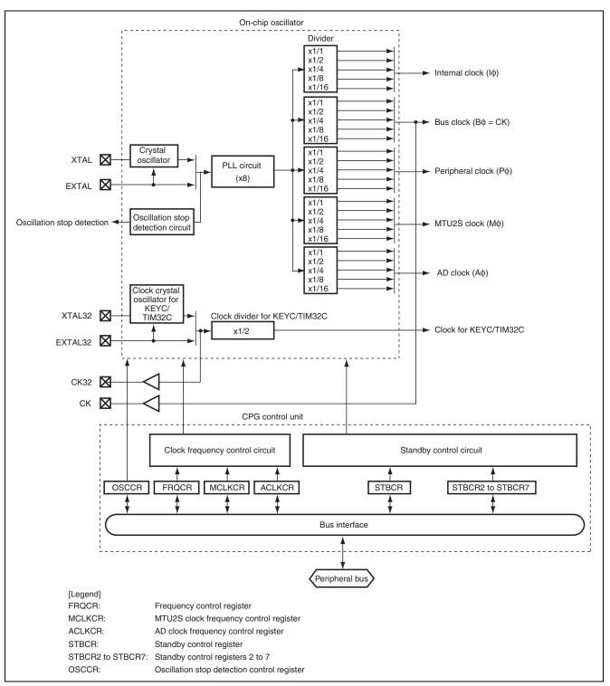
Figure 2 CPG Block Diagram
