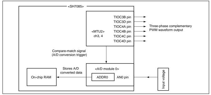
Figure 1 Block Diagram of A/D Conversion Using MTU2
