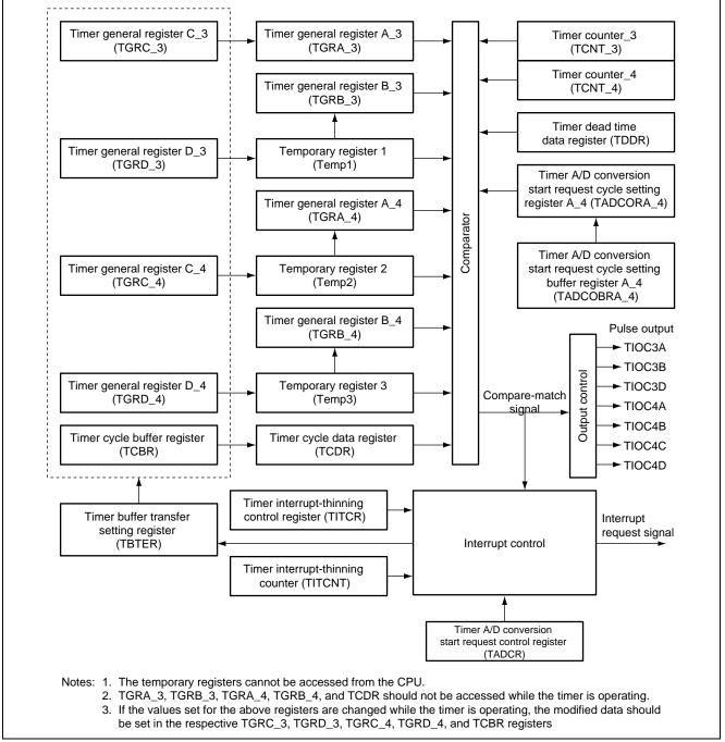
Figure 3 Block Diagram of MTU2 (ch3 and ch4) When Interrupt Skipping is Used
