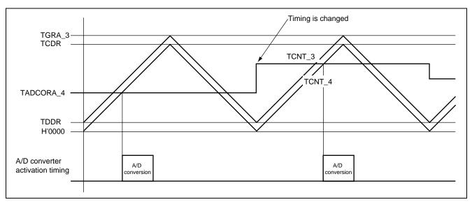
Figure 2 A/D Converter Activation Timing
