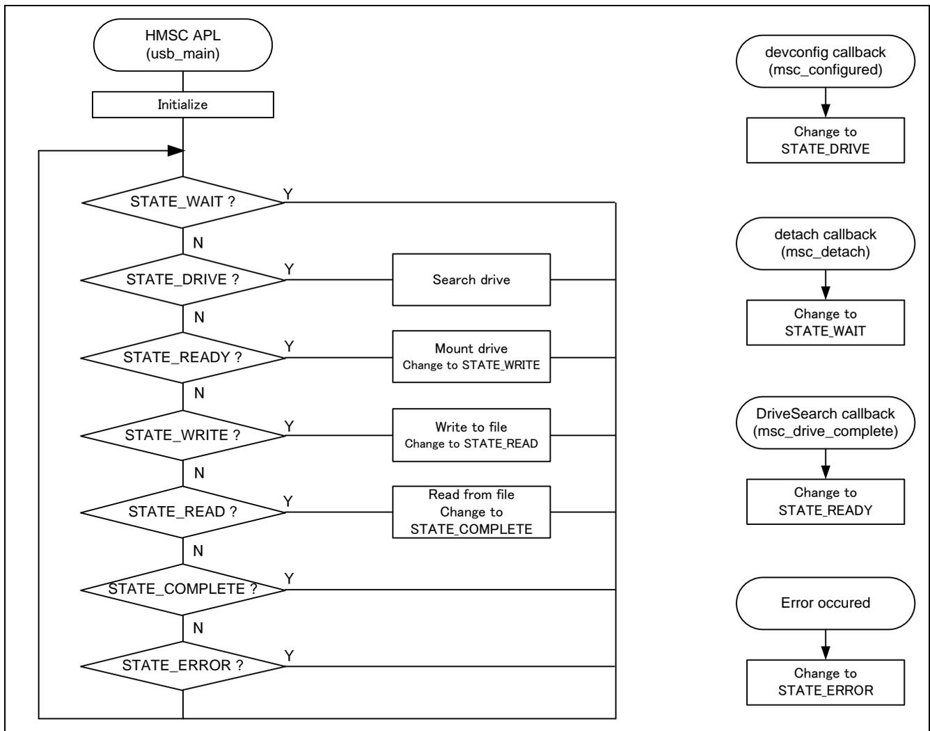
Figure 4-2 Main Loop flowchart
