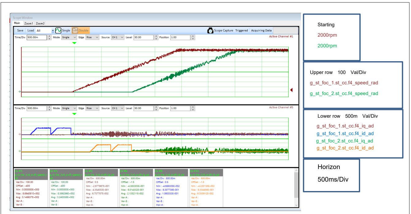
Figure 5-2 Driving Waveforms When Motors 1 and 2 are Starting up (2/3)
