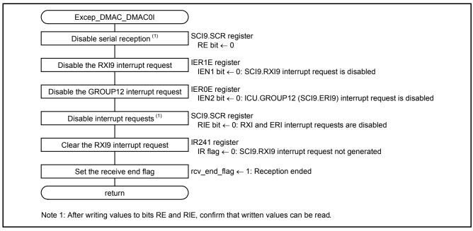
Figure 5.10 DMAC0 Transfer End Interrupt Handling
