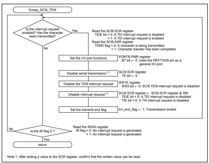
Figure 5.12 SCI9 Transmit End Interrupt Handling
