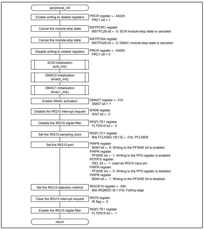
Figure 5.5 Peripheral Function Initialization
