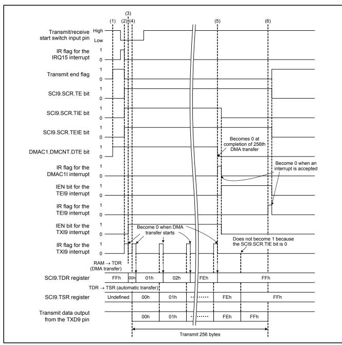
Figure 5.1 Timing Diagram When Transmitting Data
