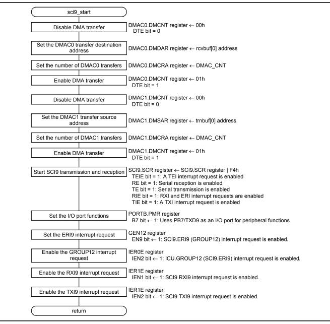
Figure 5.9 SCI9 Transmission/Reception Start
