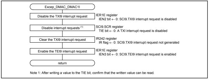
Figure 5.11 DMAC1 Transfer End Interrupt Handling
