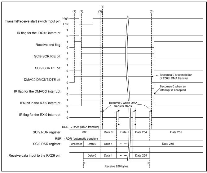
Figure 5.2 Timing Diagram When Receiving Data
