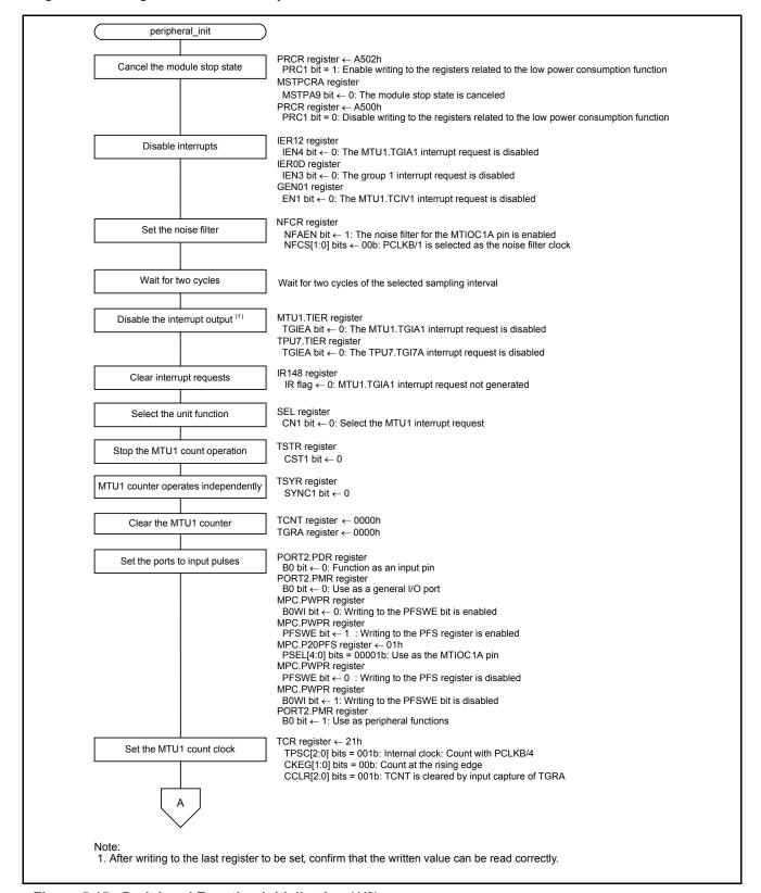
Figure 5.15 Peripheral Function Initialization (1/2)
