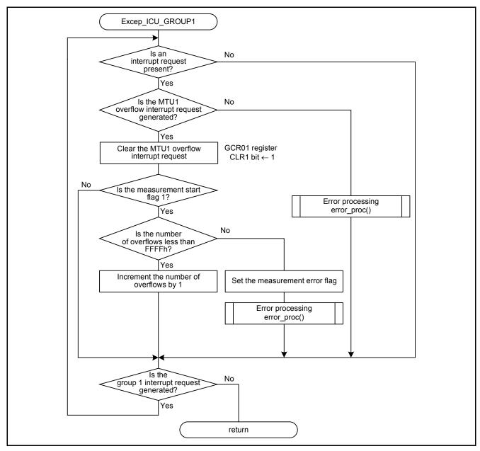
Figure 5.10 MTU1 Overflow Interrupt Handler
