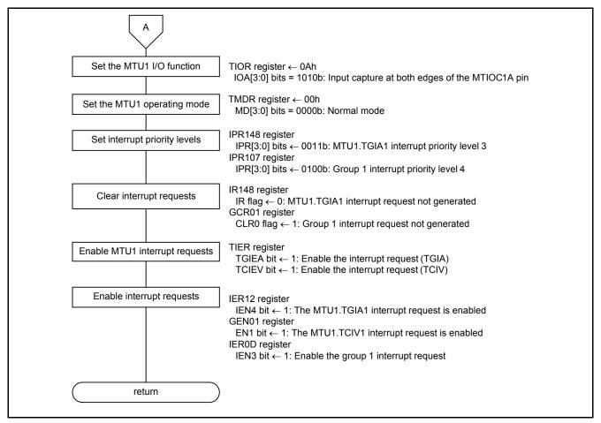
Figure 5.16 Peripheral Function Initialization (2/2)
