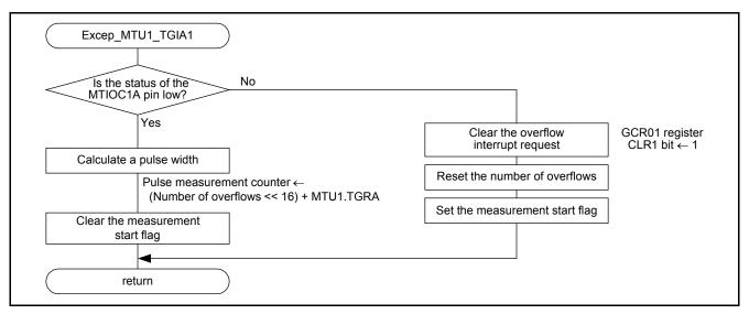
Figure 5.18 MTU1 Input Capture A Interrupt Handler
