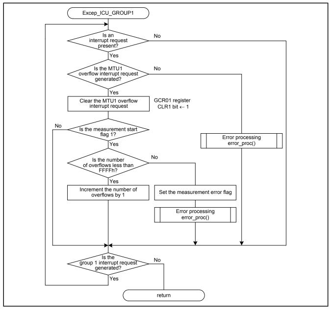
Figure 5.19 MTU1 Overflow Interrupt Handler
