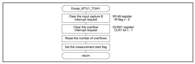
Figure 5.8 MTU1 Input Capture A Interrupt Handler
