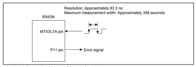
Figure 1.2 Connection Diagram of Sample Code 2
