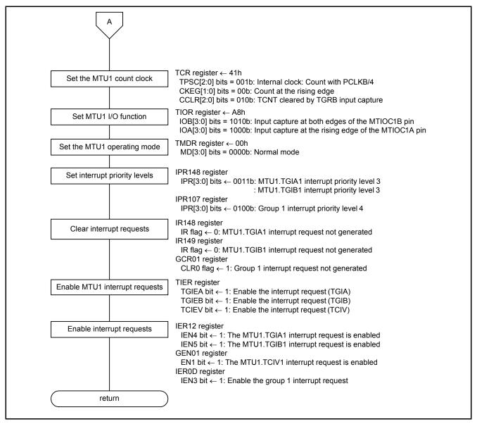
Figure 5.6 Peripheral Function Initialization (2/2)
