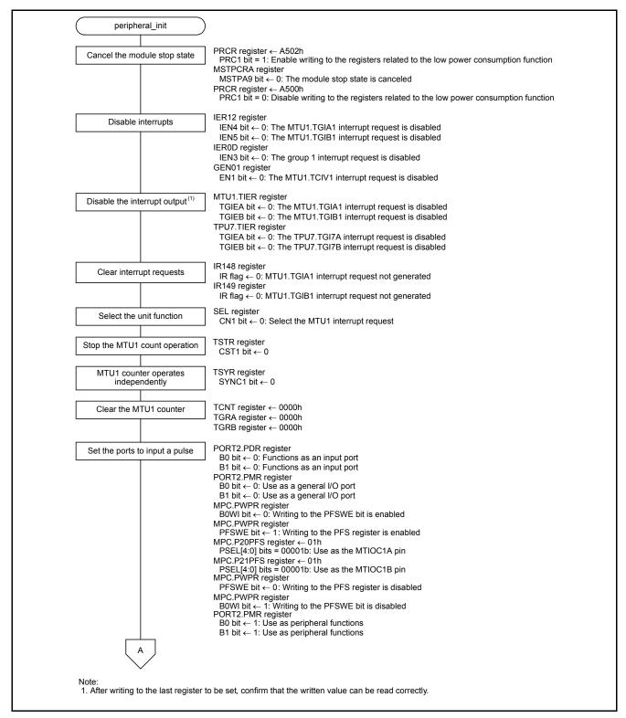
Figure 5.5 Peripheral Function Initialization (1/2)
