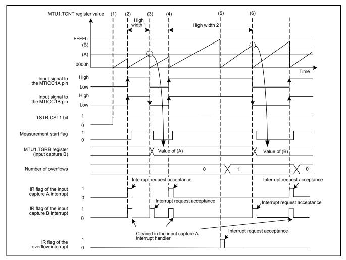
Figure 5.1 Timing Diagram of the Pulse Width Measurement
