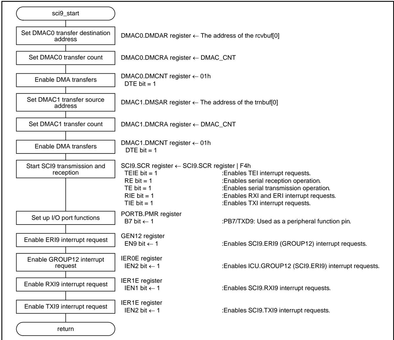
Figure 5.9 SCI9 Transmission and Reception Start
