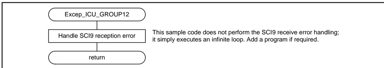
Figure 5.13 Group 12 Interrupt Handler (SCI9 Reception Error Interrupt)
