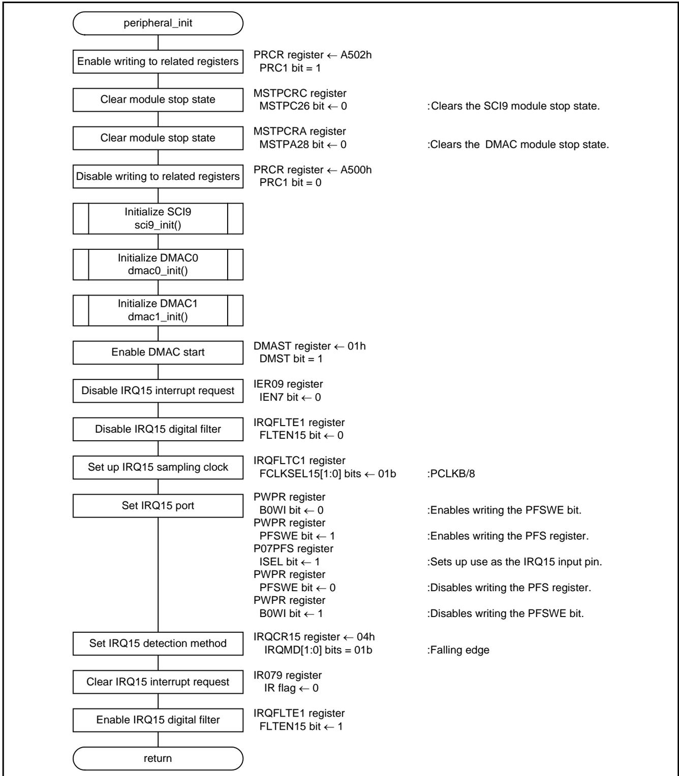
Figure 5.5 Peripheral Function Initialization
