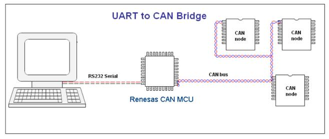
Figure 1 The RX MCU as a UART-CAN gateway between a PC and a CAN bus. Data can travel to and from the CAN bus and will all be shown on the PC terminal.
