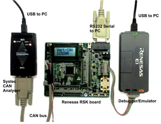
Figure 4 RSK RX630 in CAN UART Bridge test setup
