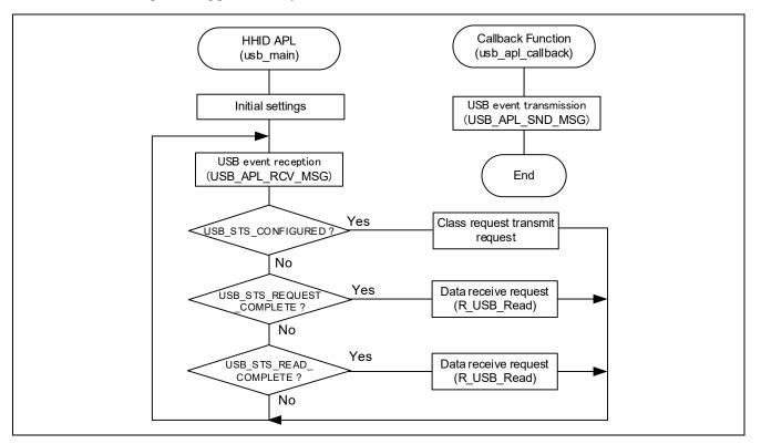
Figure 4-3 Main Loop (Normal mode)
