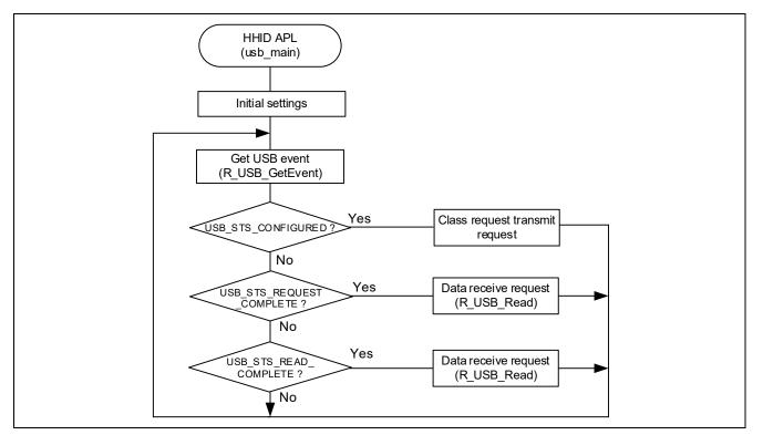
Figure 4-1 Main Loop (Normal mode)
