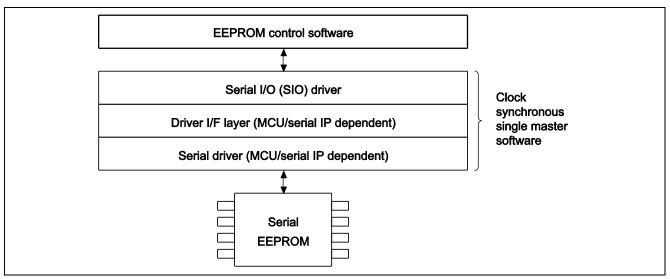
Figure 5.4 Software Configuration
