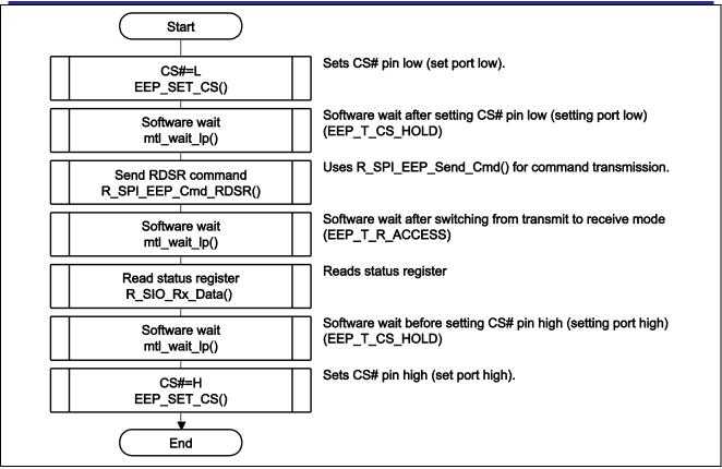
Figure 5.17 Read Status Register Command Processing Outline
