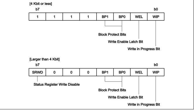
Figure 5.3 Status Register Configuration
