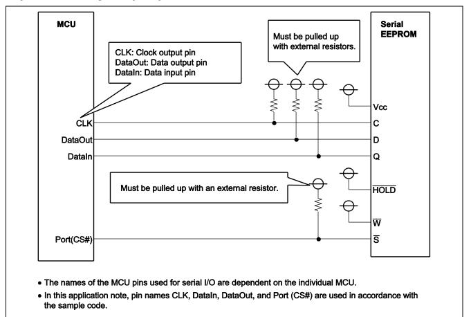
Figure 4.1 Sample Wiring Diagram for an MCU and an SPI Slave Device
