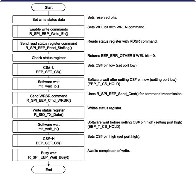
Figure 5.18 Write Status Register Command Processing Outline
