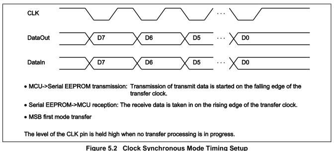
For available serial clock frequencies, see the datasheets for the individual MCUs and SPI devices.
