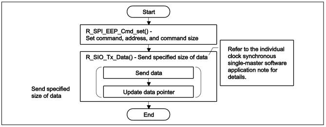
Figure 5.5 Outline of Command Transmission Processing (R\_SPI\_EEP\_Send\_Cmd())
