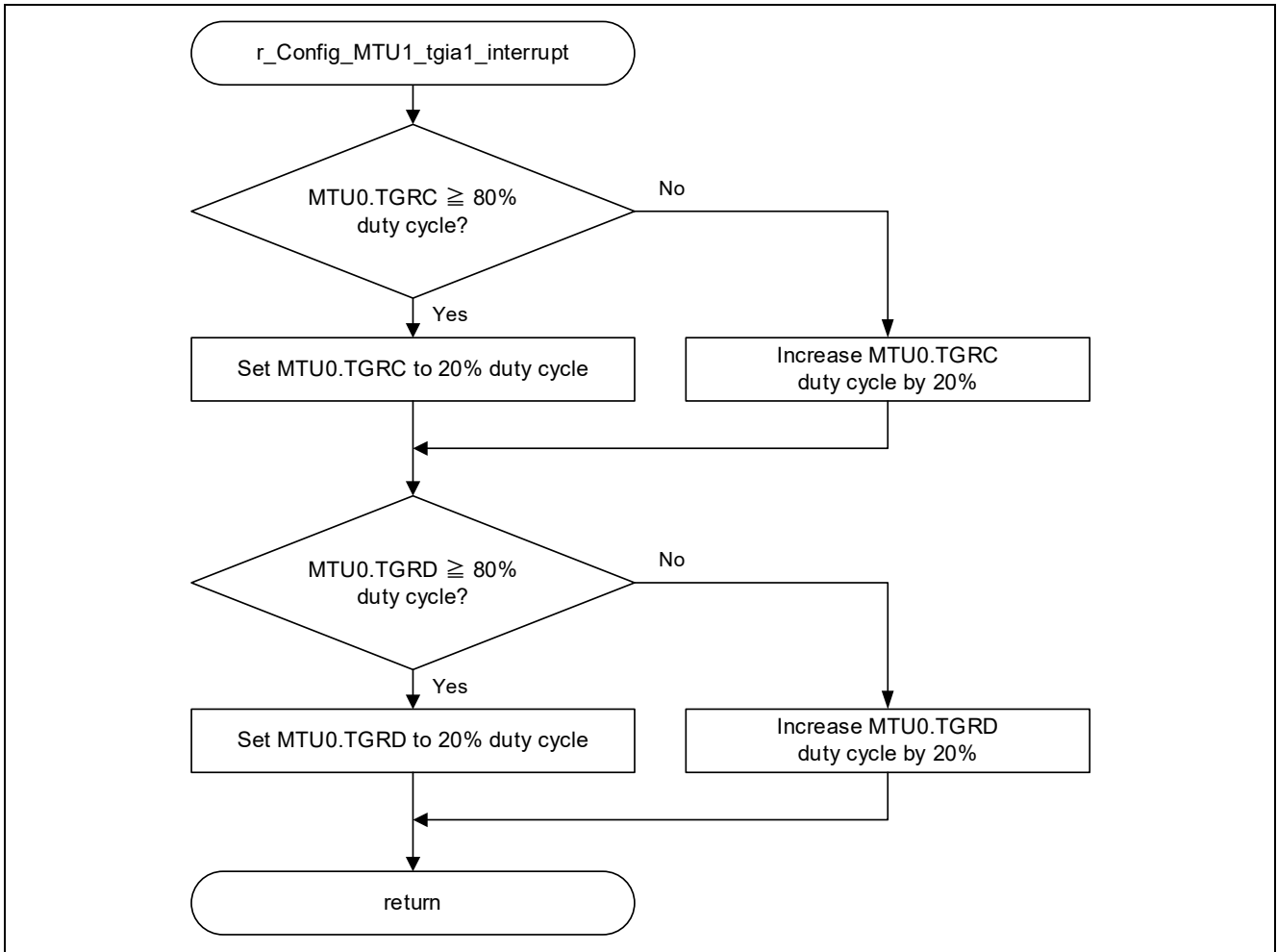
Figure 3.35 TGIA1 Interrupt Handler Function
