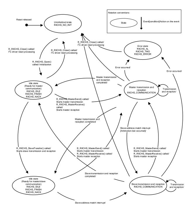
Figure 1.13 RIICHS FIT Module State Transition Diagram
