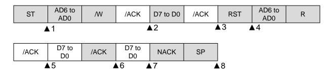
▲ 1: EEI (START) interrupt: Start condition detected
