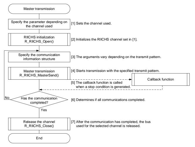
Figure 1.5 Example of Master Transmission
