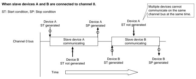
Figure 1.1 Example of Controlling Multiple Slave Devices
