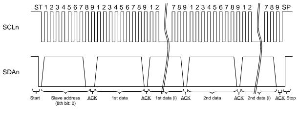
n: Channel number ST: Start condition generation SP: Stop condition generation ACK: Acknowledge: 0 \* A signal with an underline indicates data transmission from the slave to the master.
