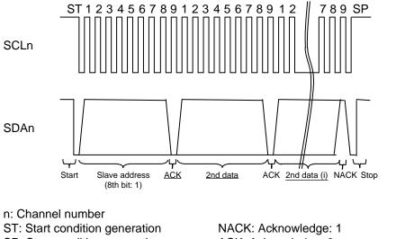
SP: Stop condition generation ACK: Acknowledge: 0 \* A signal with an underline indicates data transmission from the slave to the master.
