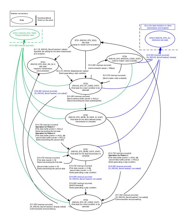
Figure 6.2 State Transition on Master Transmission (R\_RIICHS\_MasterSend() Called)
