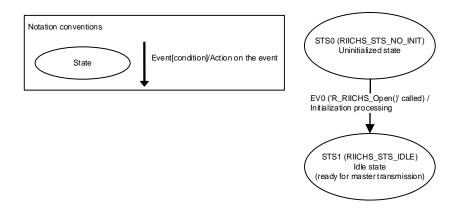
Figure 6.1 State Transition on Initialization ('R\_RIICHS\_Open()' Called)
