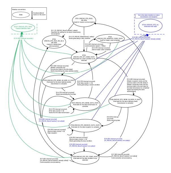
Figure 6.3 State Transition on Master Reception (R\_RIICHS\_MasterReceive() Called)
