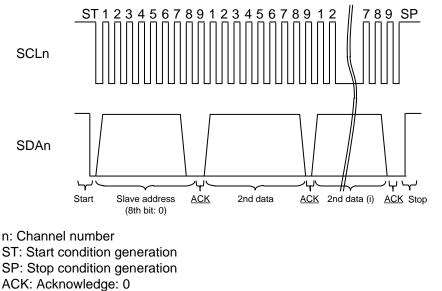
\* A signal with an underline indicates data transmission from the slave to the master.
