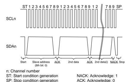
\* A signal with an underline indicates data transmission from the slave to the master.
