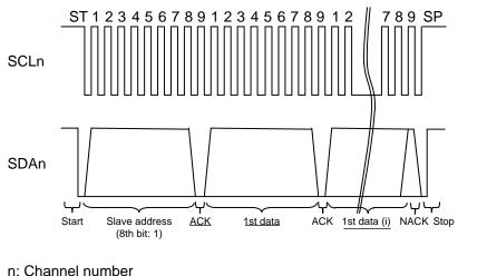
ST: Start condition generationNACK: Acknowledge: 1SP: Stop condition generationACK: Acknowledge: 0\* A signal with an underline indicates data transmission from the slave to the master.
