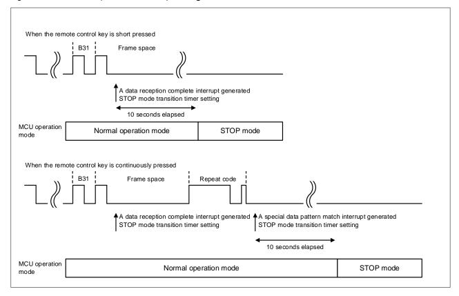
Figure 1-4 Remote Control Signal Reception State Transition Diagram
