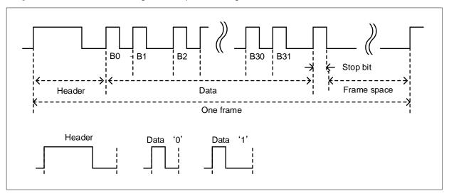
Table 1-3 shows the correspondence between remote control input signals and remote control signal data. When the third byte (B16 to B23 in Figure 1-2) of the received remote control signal data matches the signal data in Table 1-3, the application recognizes that the relevant channel button was pressed.
