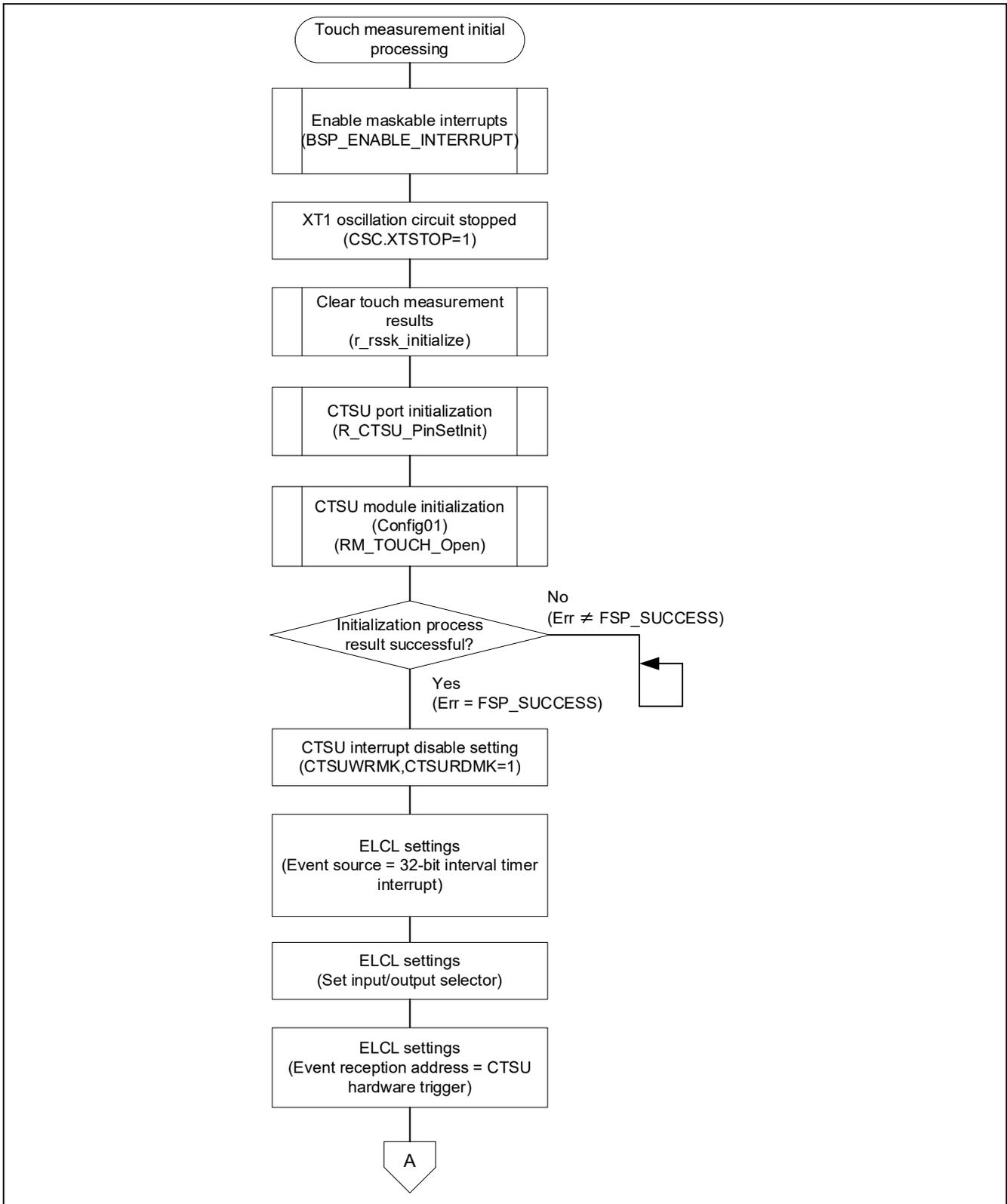
Figure 8.3 Flowchart of Touch measurement initial processing (1/3)
