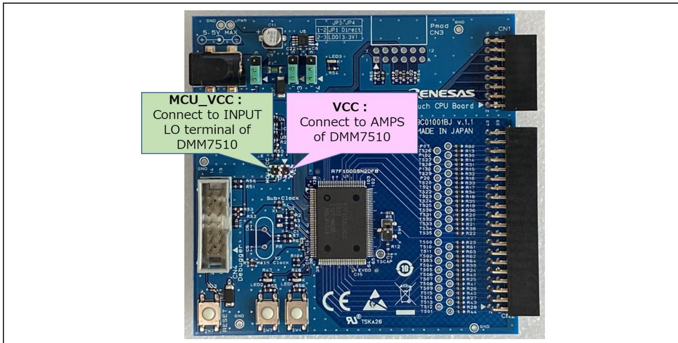
Figure 9.4 Pins of CPU board connected to the digital multimeter
