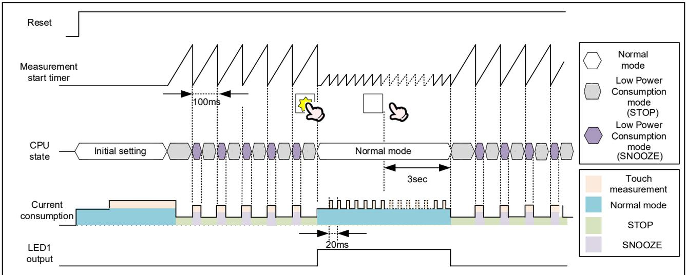
Figure 7.1 Operation image during touch measurement using SMS
