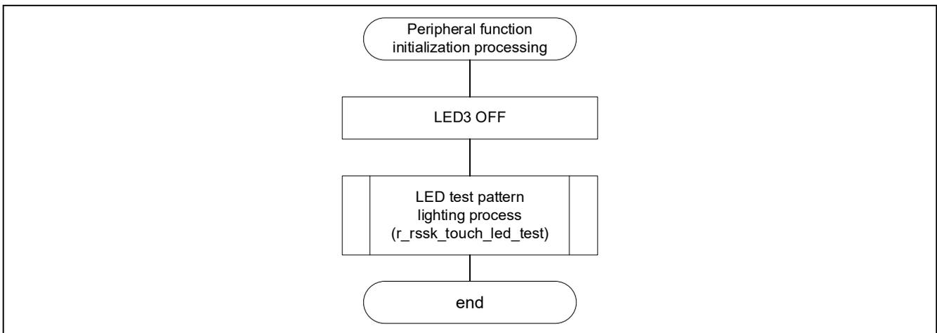
Figure 8.6 Flowchart of peripheral function initialization processing
