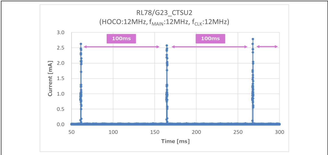
Figure 10.1 Current waveform in intermittent operation with touch measurement every 100ms
