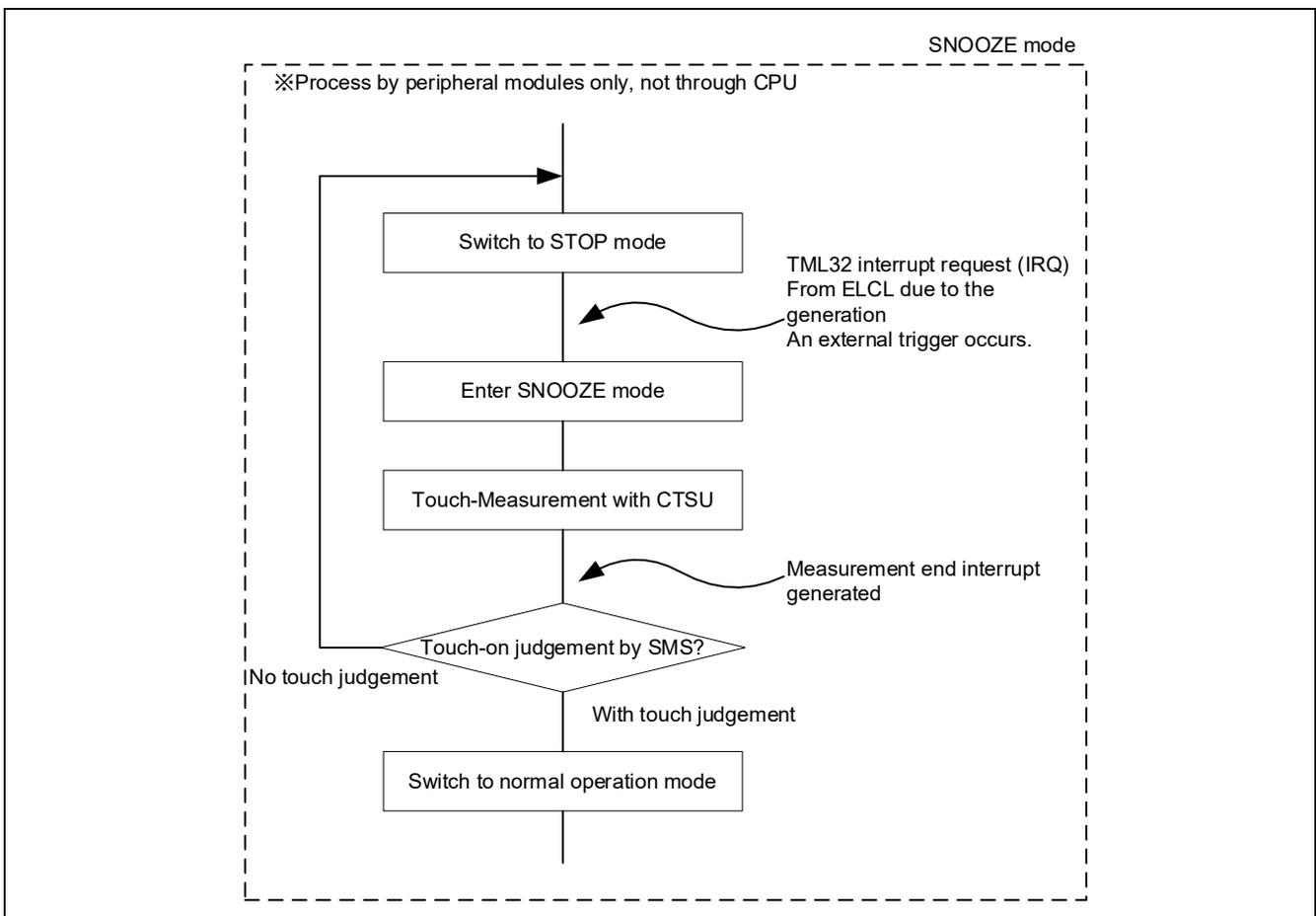
Figure 8.10 Flowchart of SMS processing in SNOOZE mode
