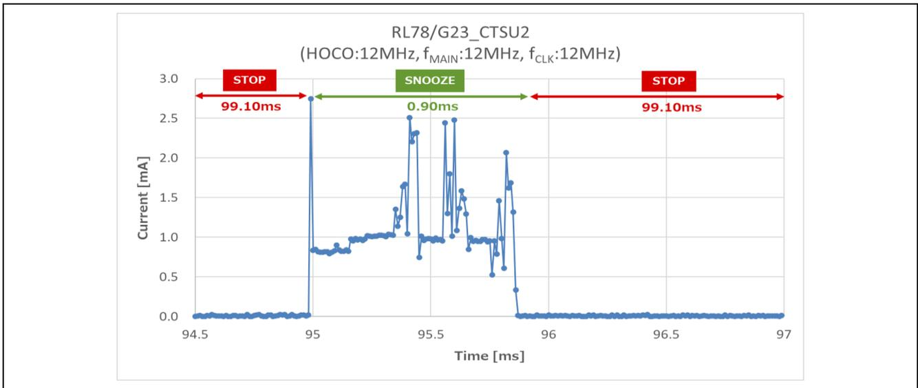
Figure 10.2 Current consumption waveform 1ch measurement (Touch measurement using SMS)
