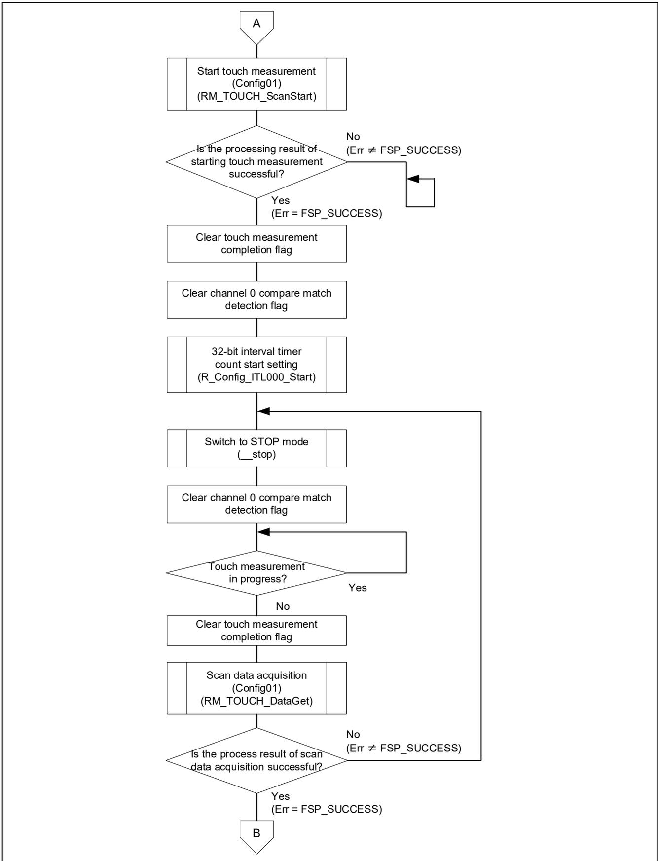
Figure 8.4 Flowchart of Touch measurement initial processing (2/3)
