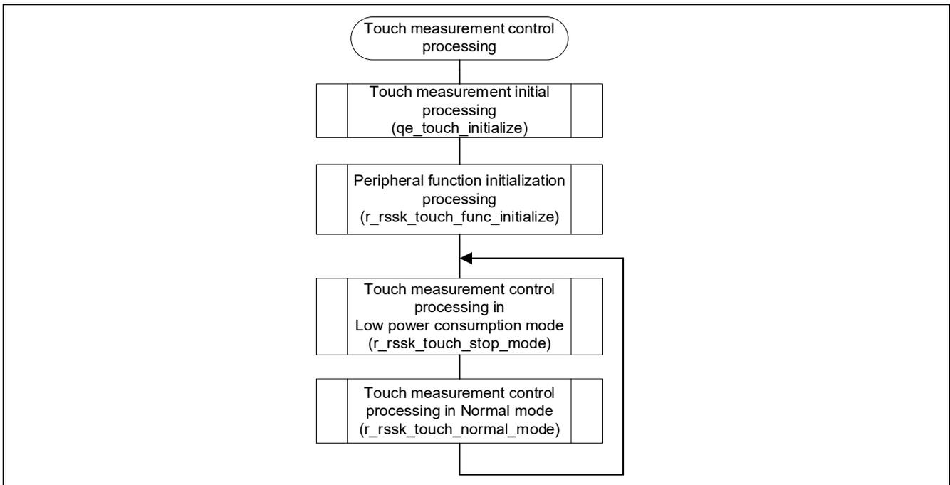
Figure 8.2 Flowchart of Touch measurement control processing
