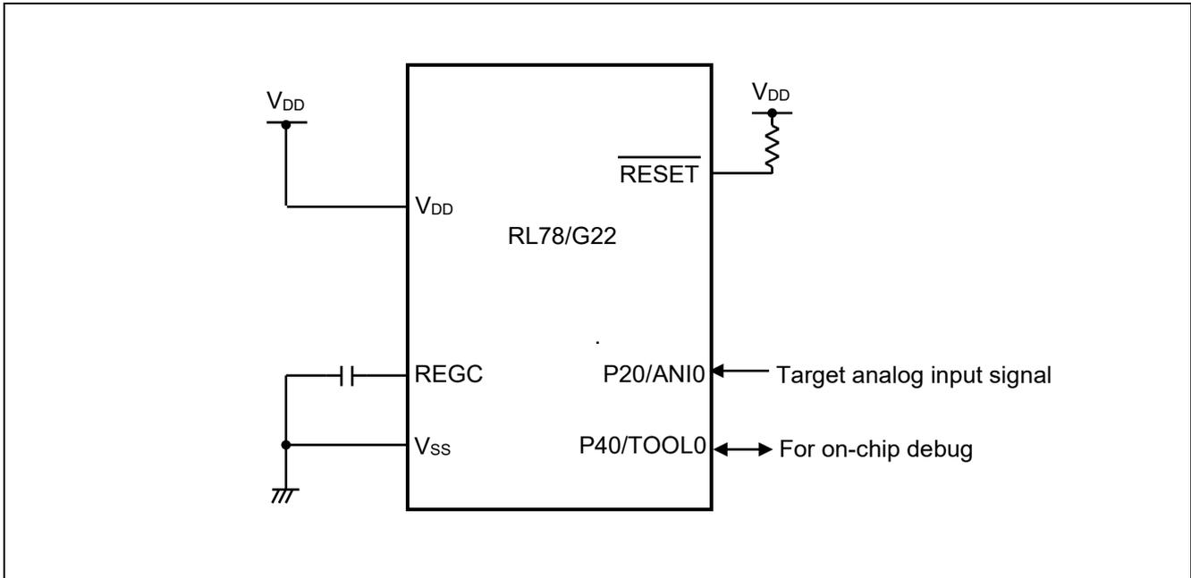
Note 1. This simplified circuit diagram was created to show an overview of connections only. When actually designing your circuit, make sure the design includes appropriate pin handling and meets electrical characteristic requirements (connect each input-only port to  $V_{DD}$  or  $V_{SS}$  through a resistor).
