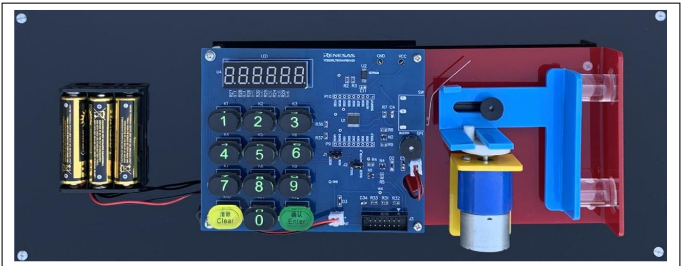
Figure 1.2 Photo of Circuit Board of Electronic Safe Box
