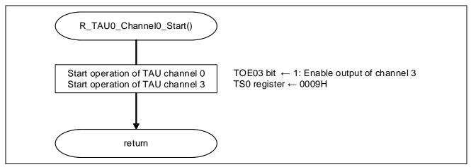
Figure 5.12 Timer Array Unit Operation Start
