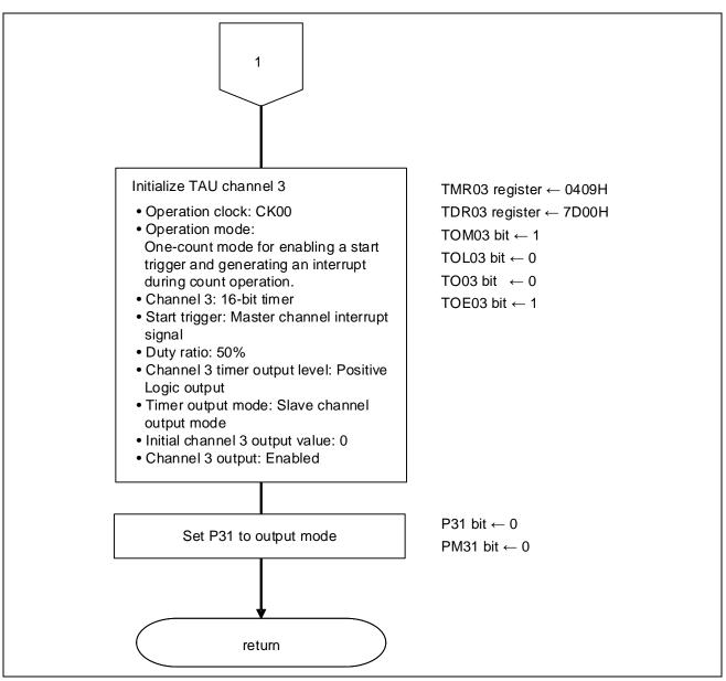
Figure 5.10 Timer Array Unit Setup (2/2)
