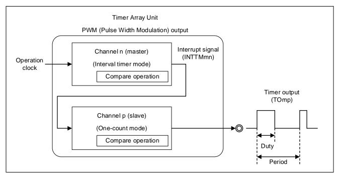
Figure 5.1 Operation Overview (example of migration from timer mode (output compare function) or PWM mode)
