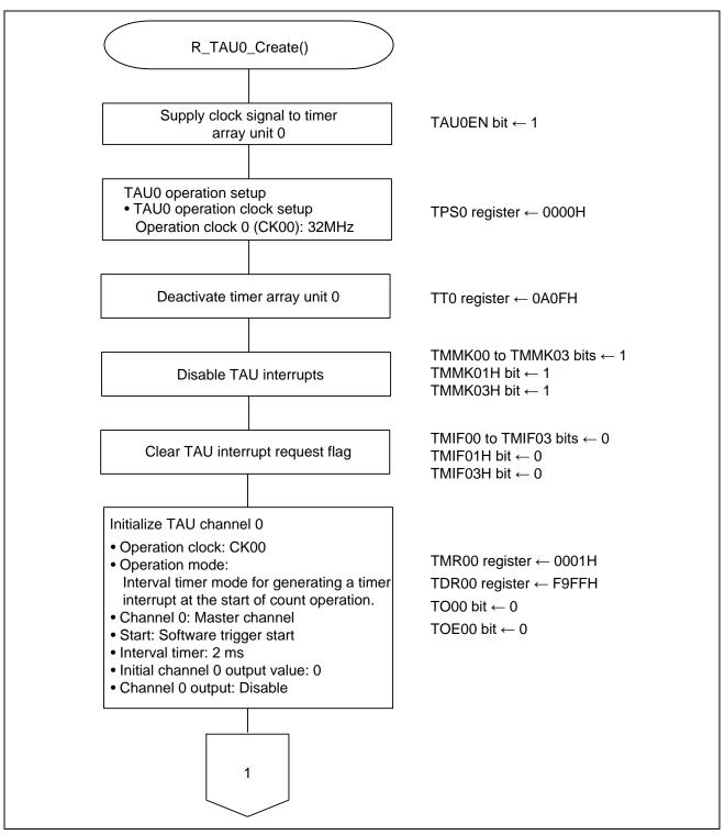
Figure 5.9 Timer Array Unit Setup (1/2)
