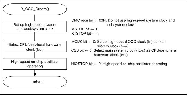
Figure 4.7 CPU Clock Setup
