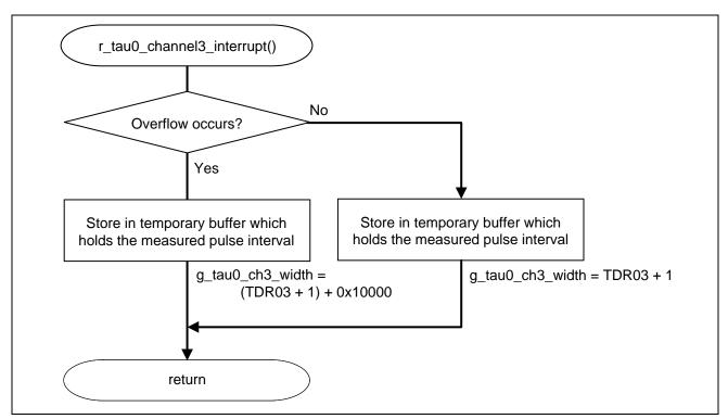
Figure 4.12 INTTM03 Interrupt Processing
