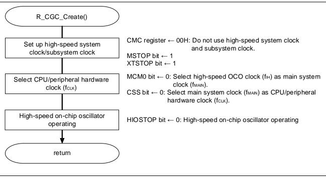
Figure 5.7 CPU Clock Setup
