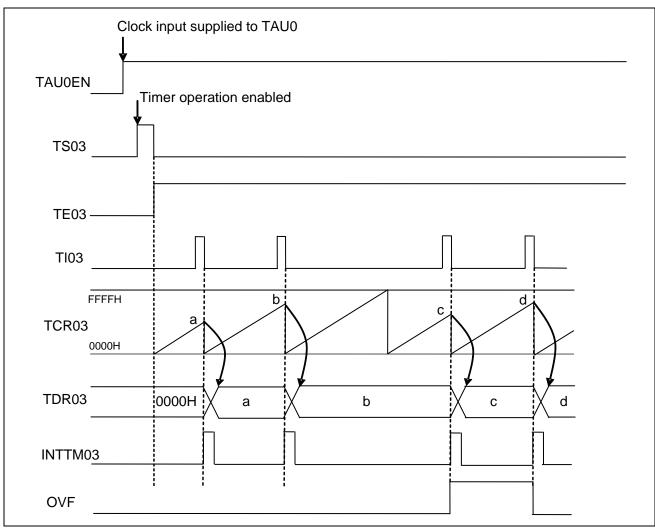
Figure 4.3 Overview of Timer Operation and Interrupts
