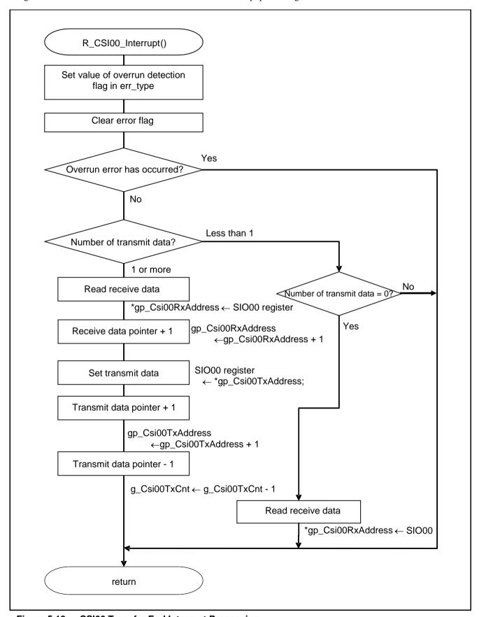
Figure 5.12 CSI00 Transfer End Interrupt Processing
