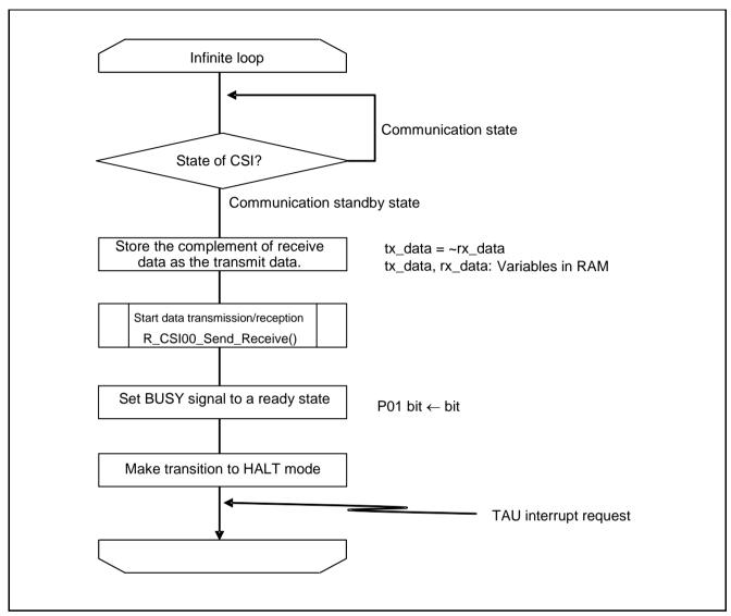
Figure 5.10 Infinite Loop in Main Processing
