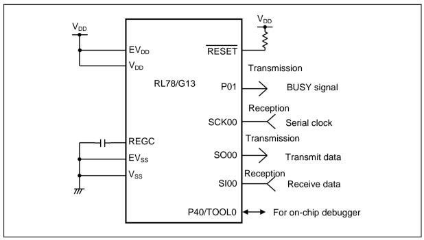
Figure 4.1 Hardware Configuration
