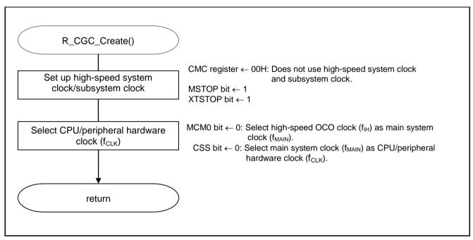
Figure 5.5 **CPU Clock Setup**
