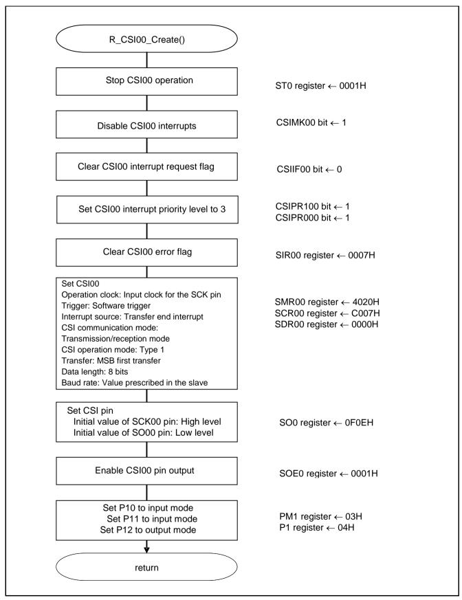
Figure 5.7 SAU0 Channel 0 (CSI00) Operation Setup
