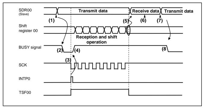
Figure 1.3 Example of BUSY Signal Control by SCK Detection in the Slave
