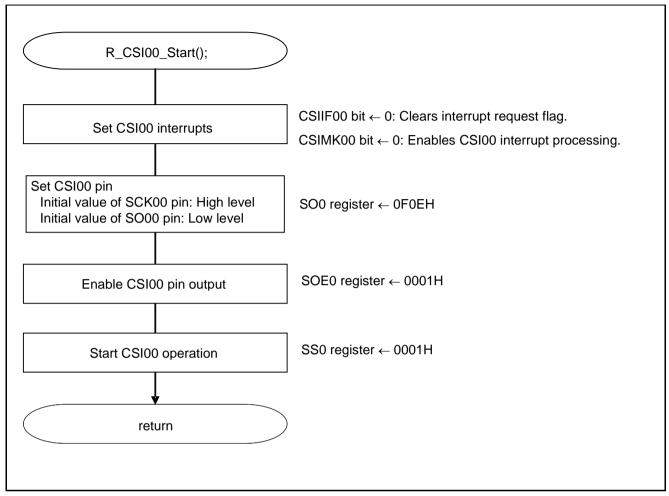
Figure 5.9 SAU0 Channel 0 (CSI00) Operation Start Processing
