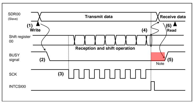
Figure 1.2 Handshake Operation and Communication
