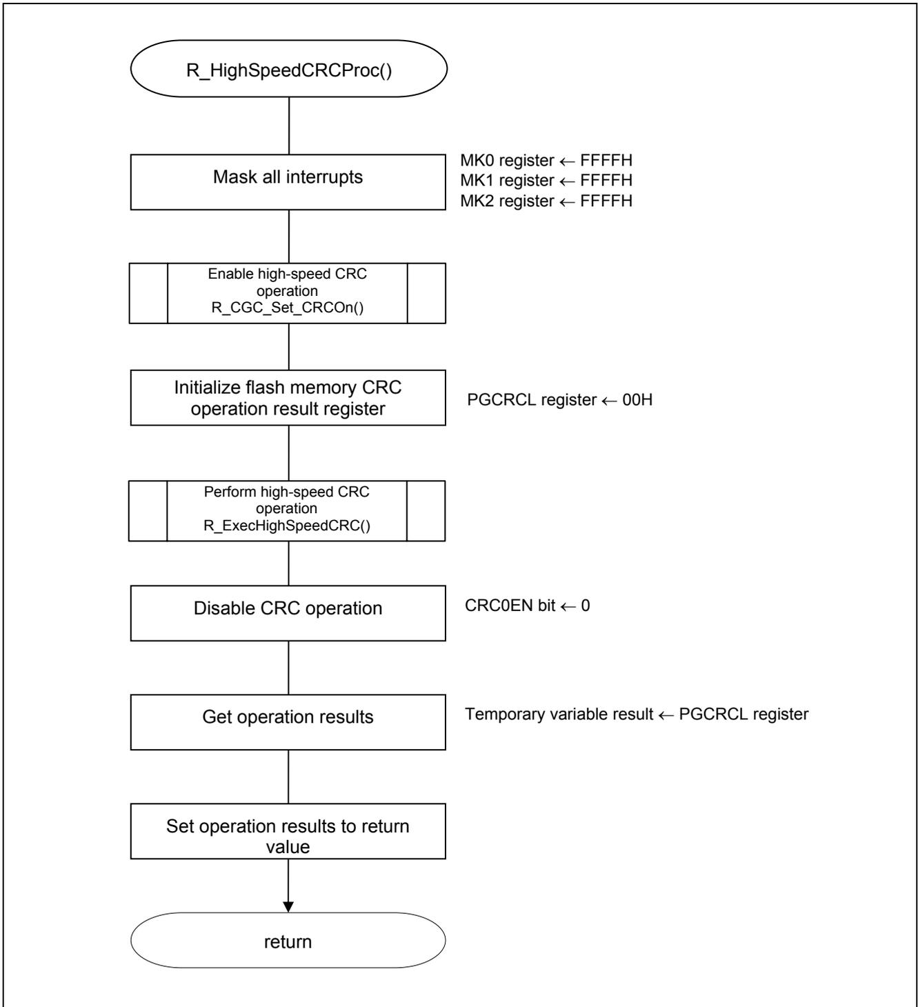
Figure 5.9 High-speed CRC Operation Processing
