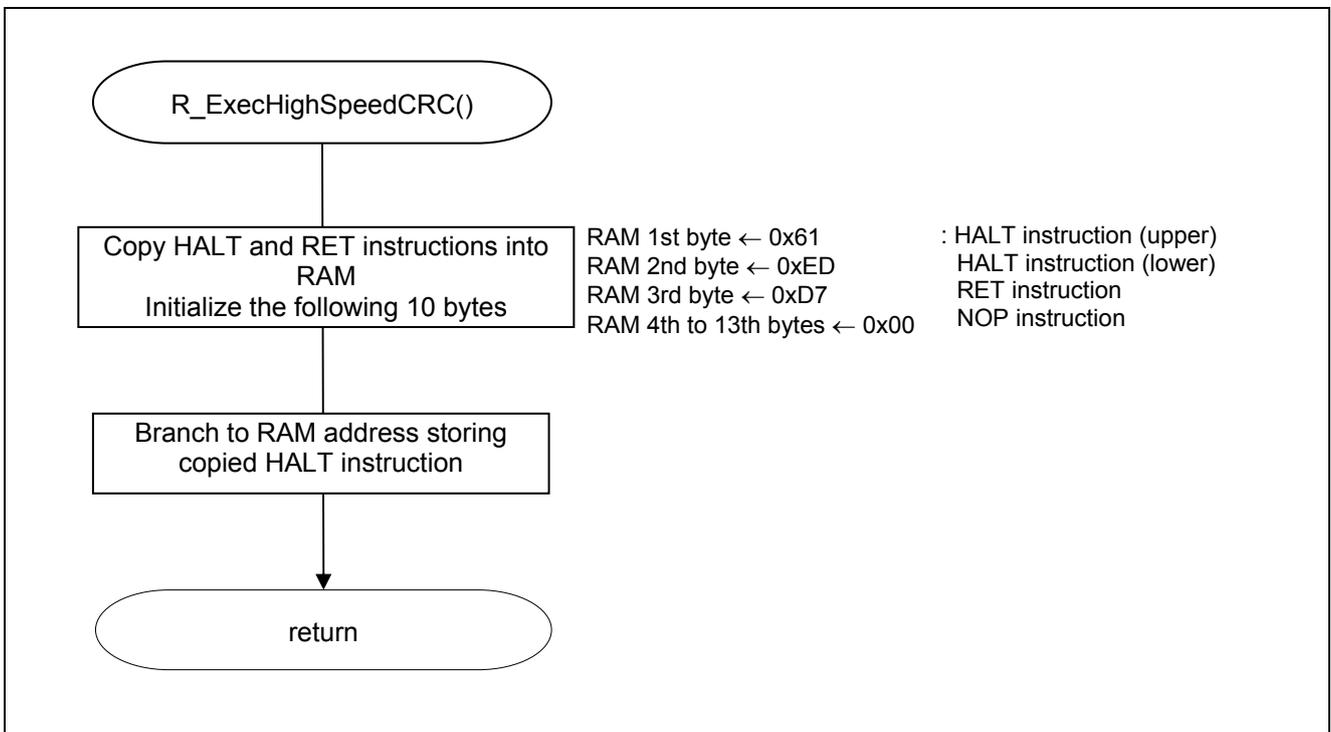
Figure 5.11 Performing High-speed CRC Operation
