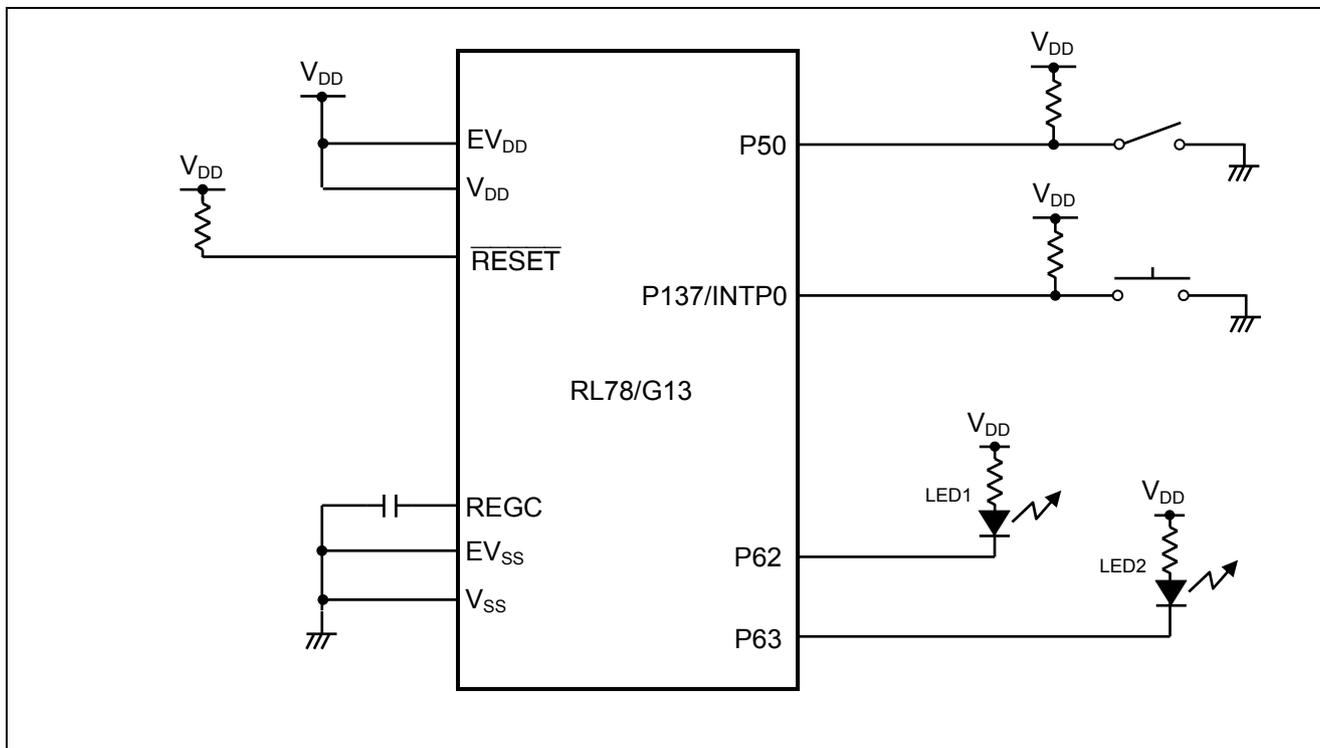
**Figure 4.1 Hardware Configuration**
