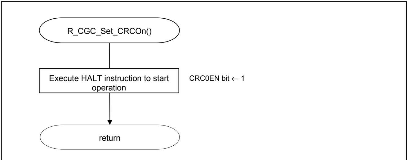
Figure 5.10 Enabling High-speed CRC Operation
