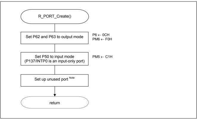
Figure 5.4 I/O Port Setup
