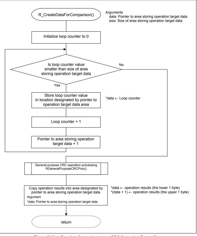
Figure 5.12 Creating General-purpose CRC Operation Target Data
