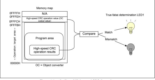
Figure 1.1 Outline of High-speed CRC Operation
