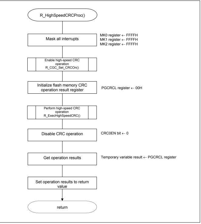
Figure 5.9 High-speed CRC Operation Processing
