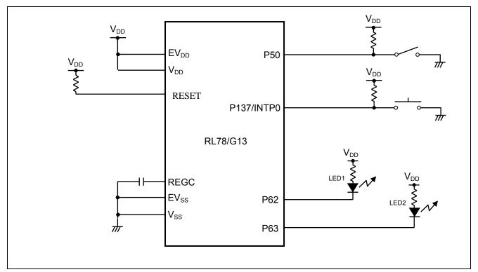
Figure 4.1 Hardware Configuration
