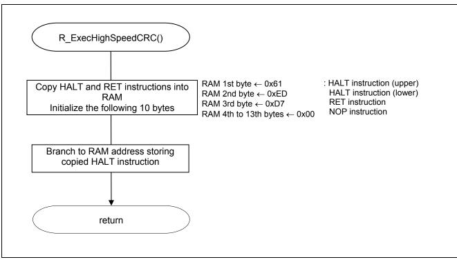
Figure 5.11 Performing High-speed CRC Operation
