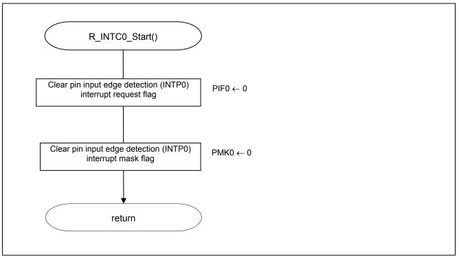
Figure 5.14 Starting INTP0 Operation
