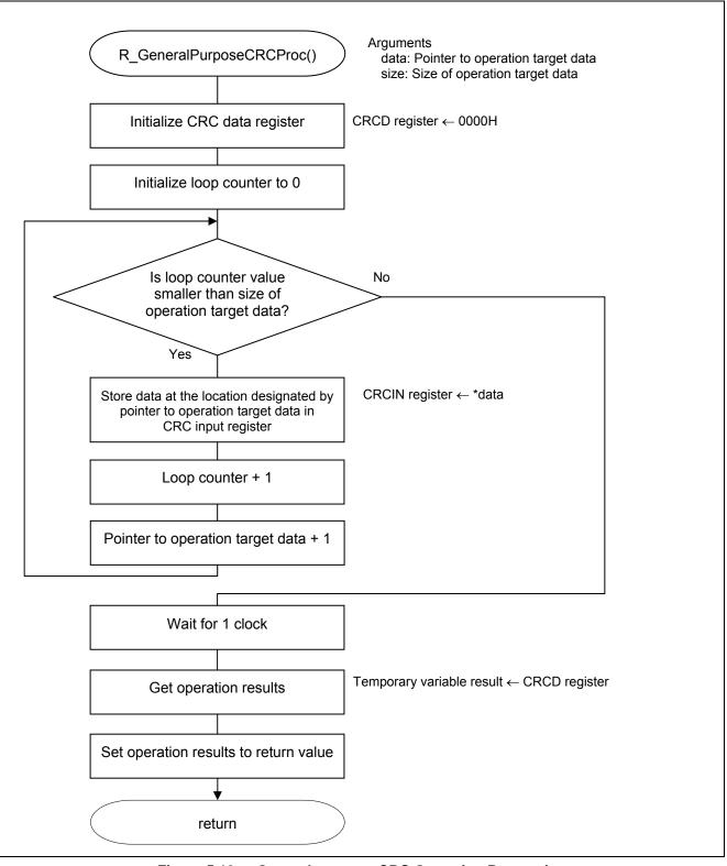
Figure 5.13 General-purpose CRC Operation Processing
