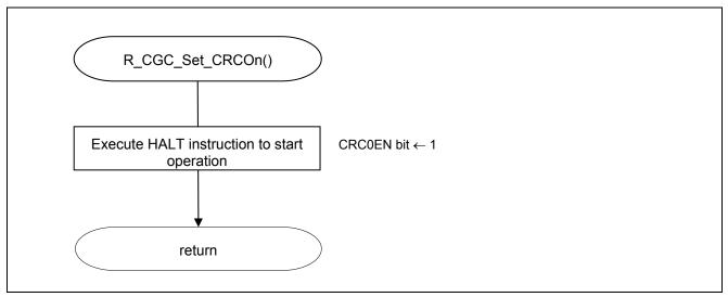
Figure 5.10 Enabling High-speed CRC Operation
