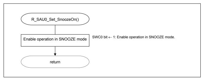
Figure 5.12 Enabling CSI00 in SNOOZE Mode
