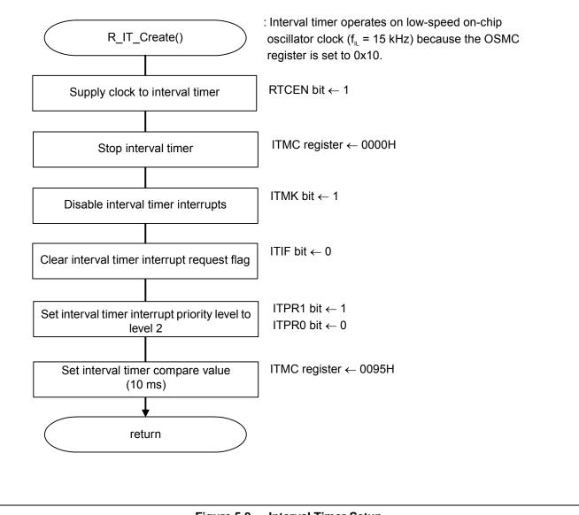
Figure 5.8 Interval Timer Setup
