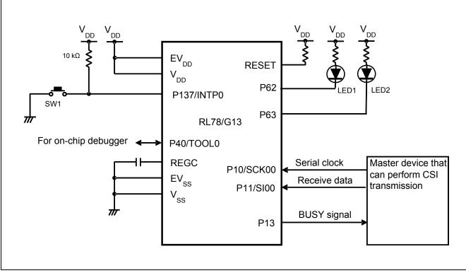
Figure 4.1 Hardware Configuration
