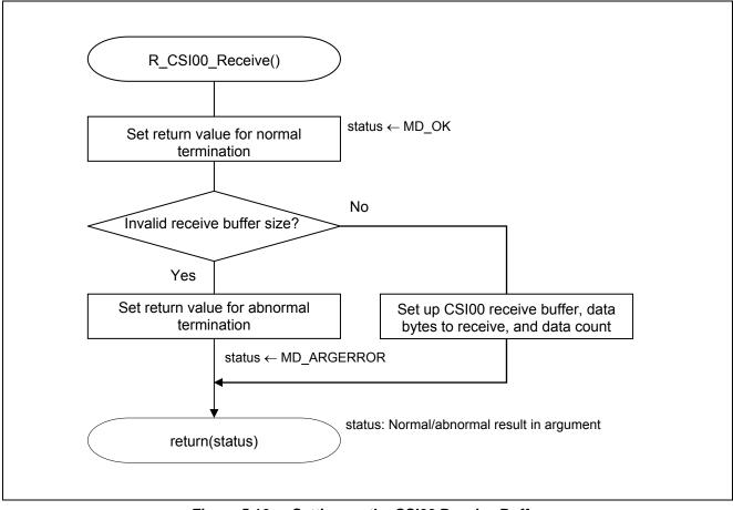
Figure 5.16 Setting up the CSI00 Receive Buffer
