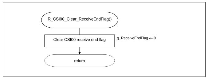
Figure 5.20 Clearing the Receive End Flag
