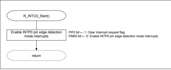
Figure 5.21 Starting INTP0 Operation
