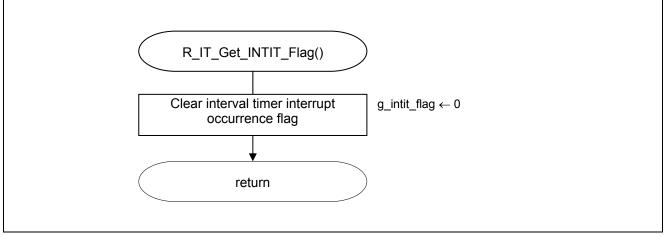
Figure 5.30 Clearing the Interval Timer Interrupt Occurrence Flag
