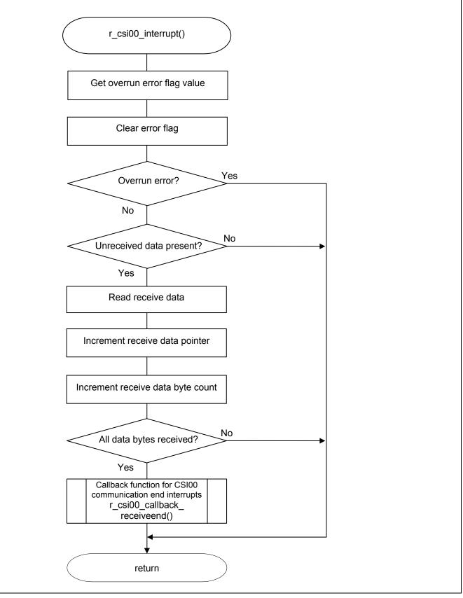
Figure 5.17 CSI00 Communication End Interrupt
