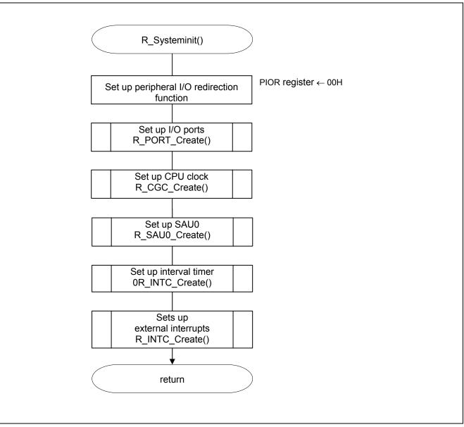
Figure 5.3 System Initialization Function
