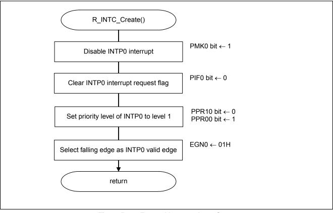
Figure 5.9 External Interrupt Input Setup
