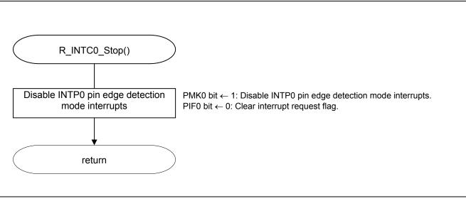
Figure 5.22 Stopping INTP0 Operation
