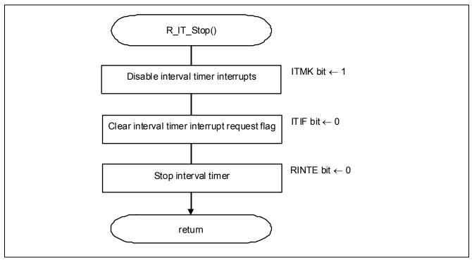
Figure 5.25 Stopping Interval Timer
