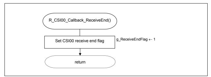
Figure 5.18 Callback Function for SI00 Communication End Interrupts
