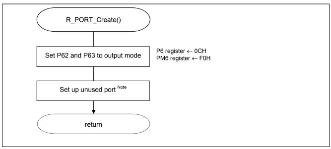
Figure 5.4 I/O Port Setup
