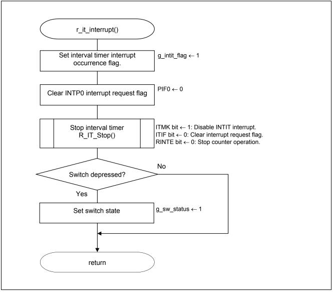
Figure 5.26 Interval Timer Interrupt
