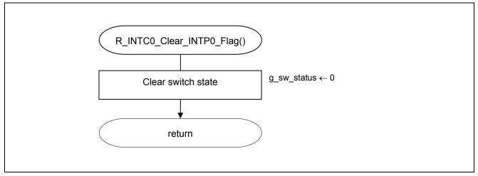
Figure 5.28 Clearing the Switch State
