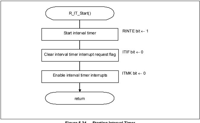
Figure 5.24 **Starting Interval Timer**
