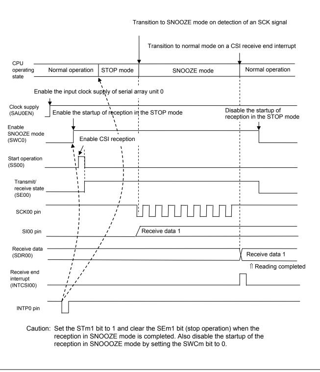
Figure 1.3 Timing Chart of SNOOZE Mode
