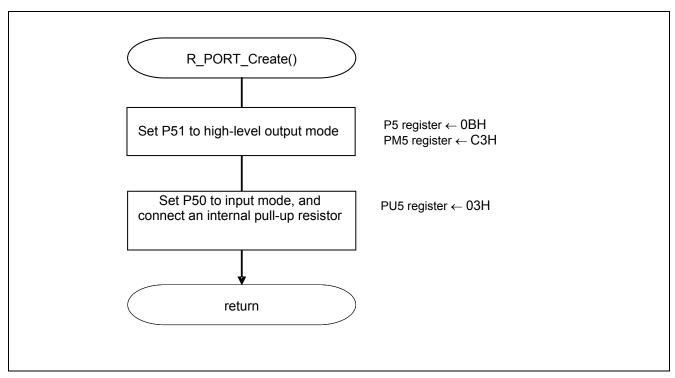
Figure 5.4 I/O Port Setup
