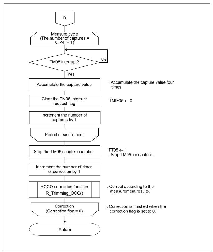
Figure 5.13 Calibration with XT1 Oscillation (2/2)
