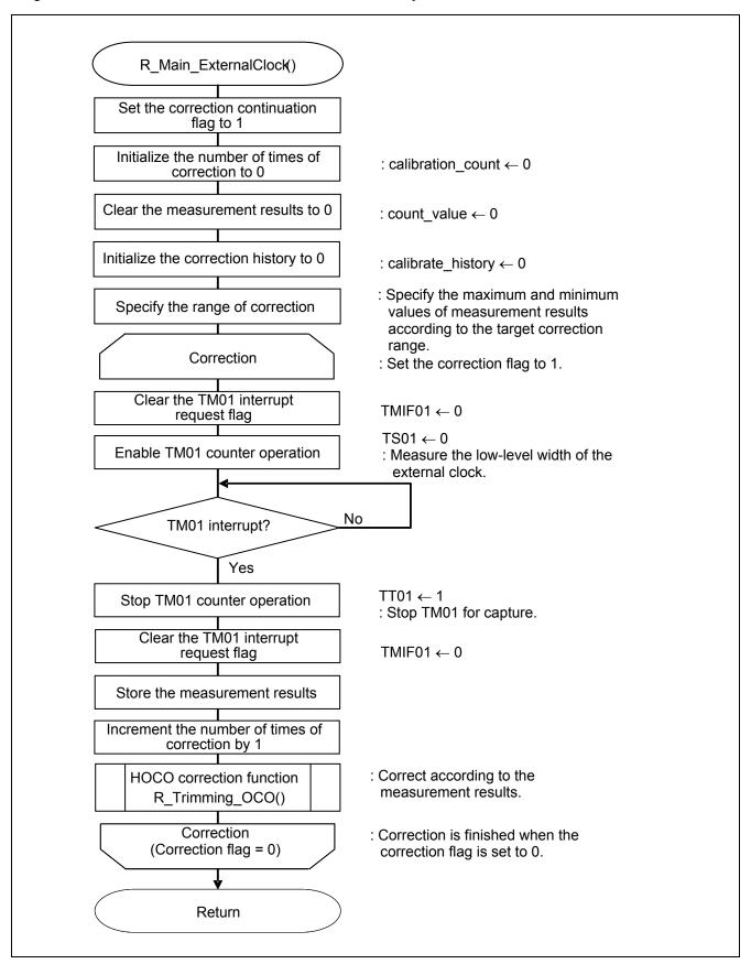
Figure 5.14 Calibration with External Input Clock
