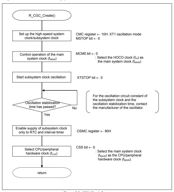
Figure 5.5 CPU Clock Setup
