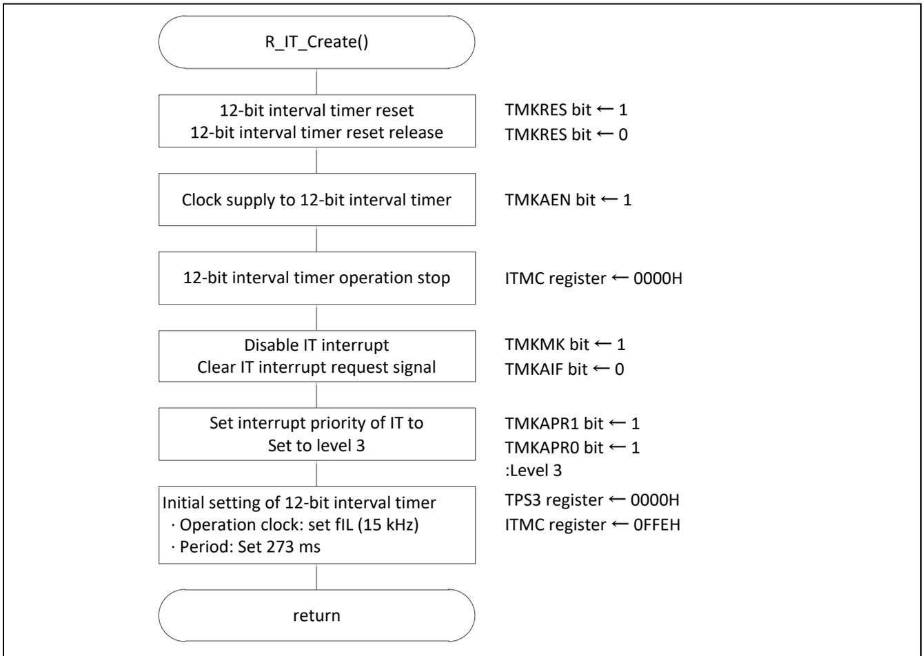
Figure 5.11 Setting 12-Bit Interval Timer
