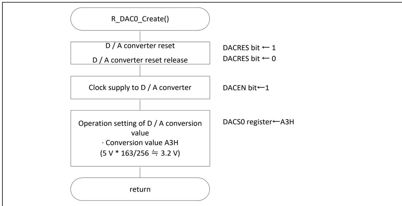
Figure 5.7 Setting D/A Converter
