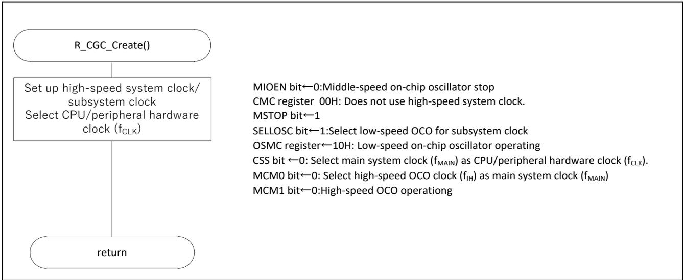
Figure 5.5 Setting CPU Clock
