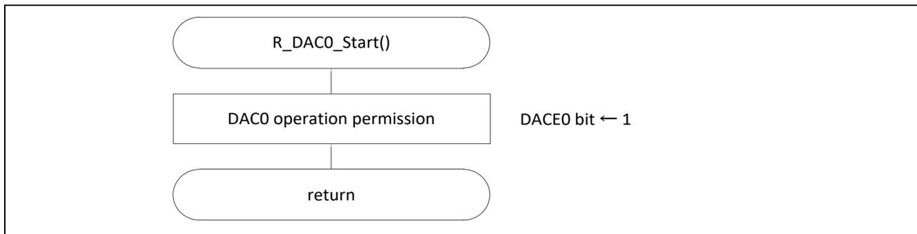
Figure 5.15 Starting D/A Converter Operation
