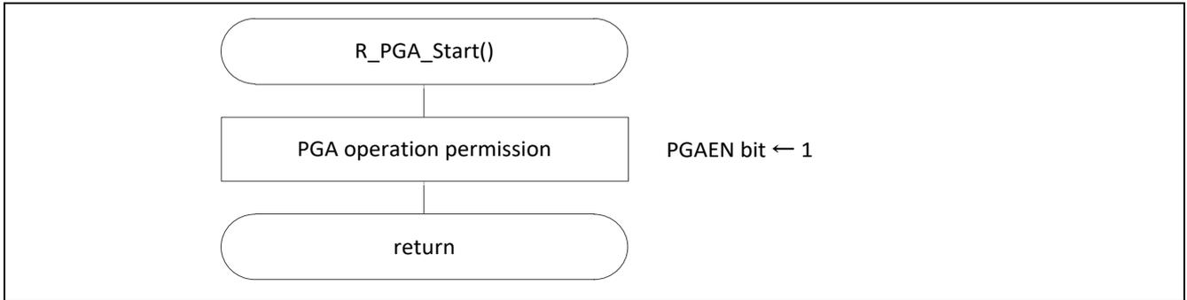
Figure 5.16 Starting PGA Operation
