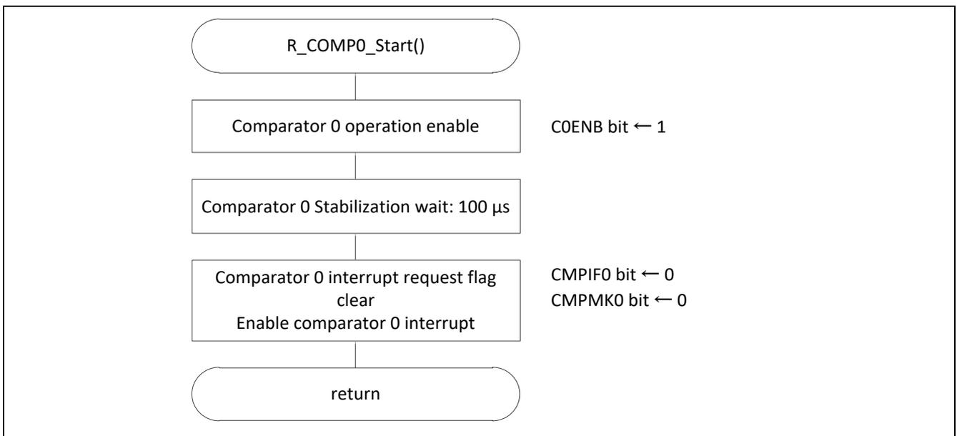
Figure 5.17 Starting Comparator 0 Operation
