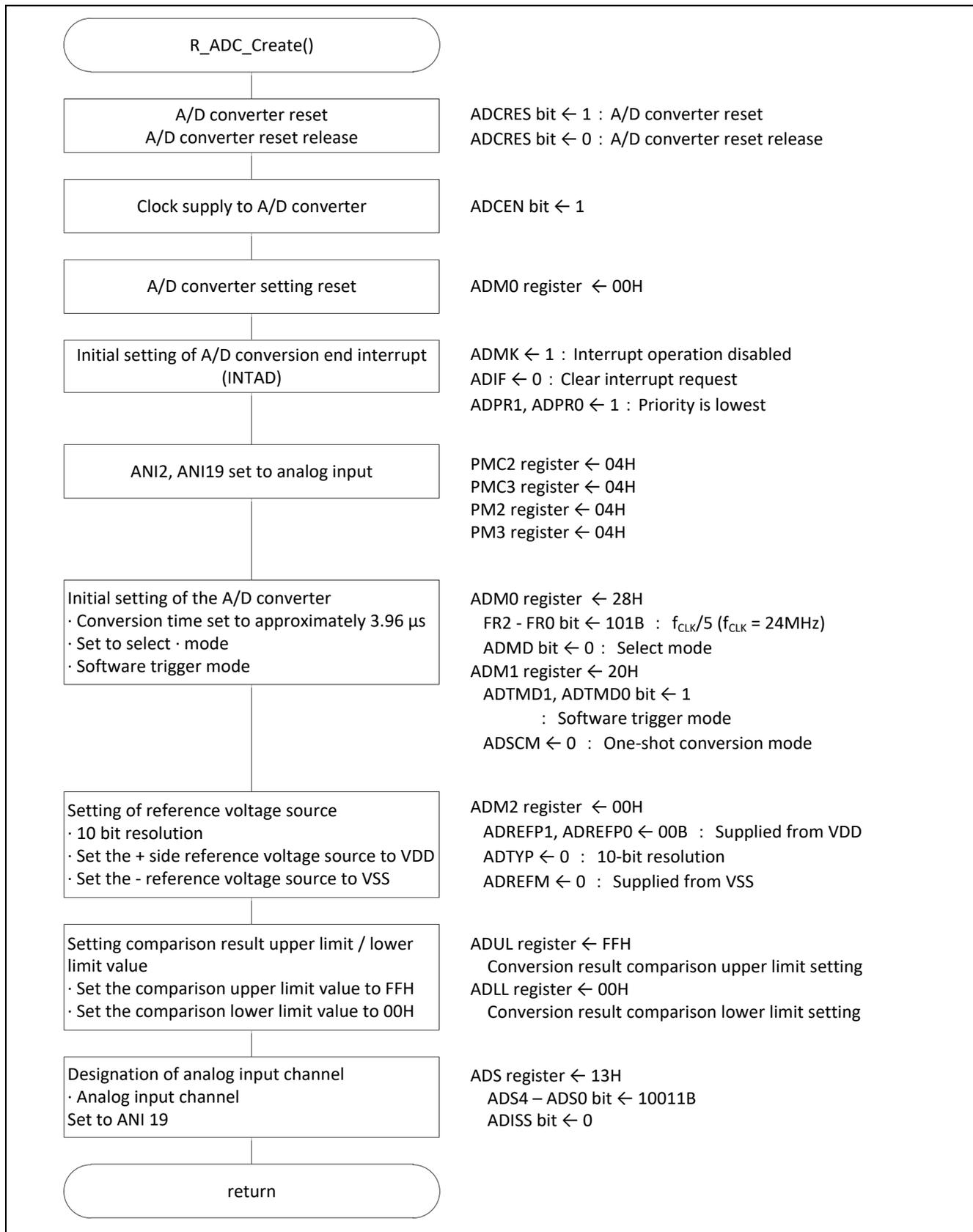
Figure 5.12 A/D Converter Setup
