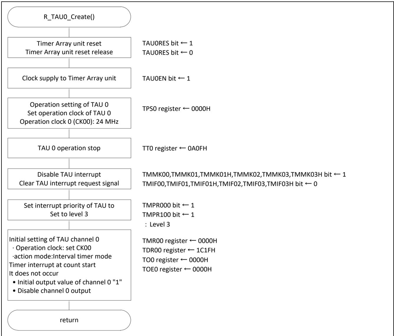
Figure 5.10 Setting Timer Array Unit
