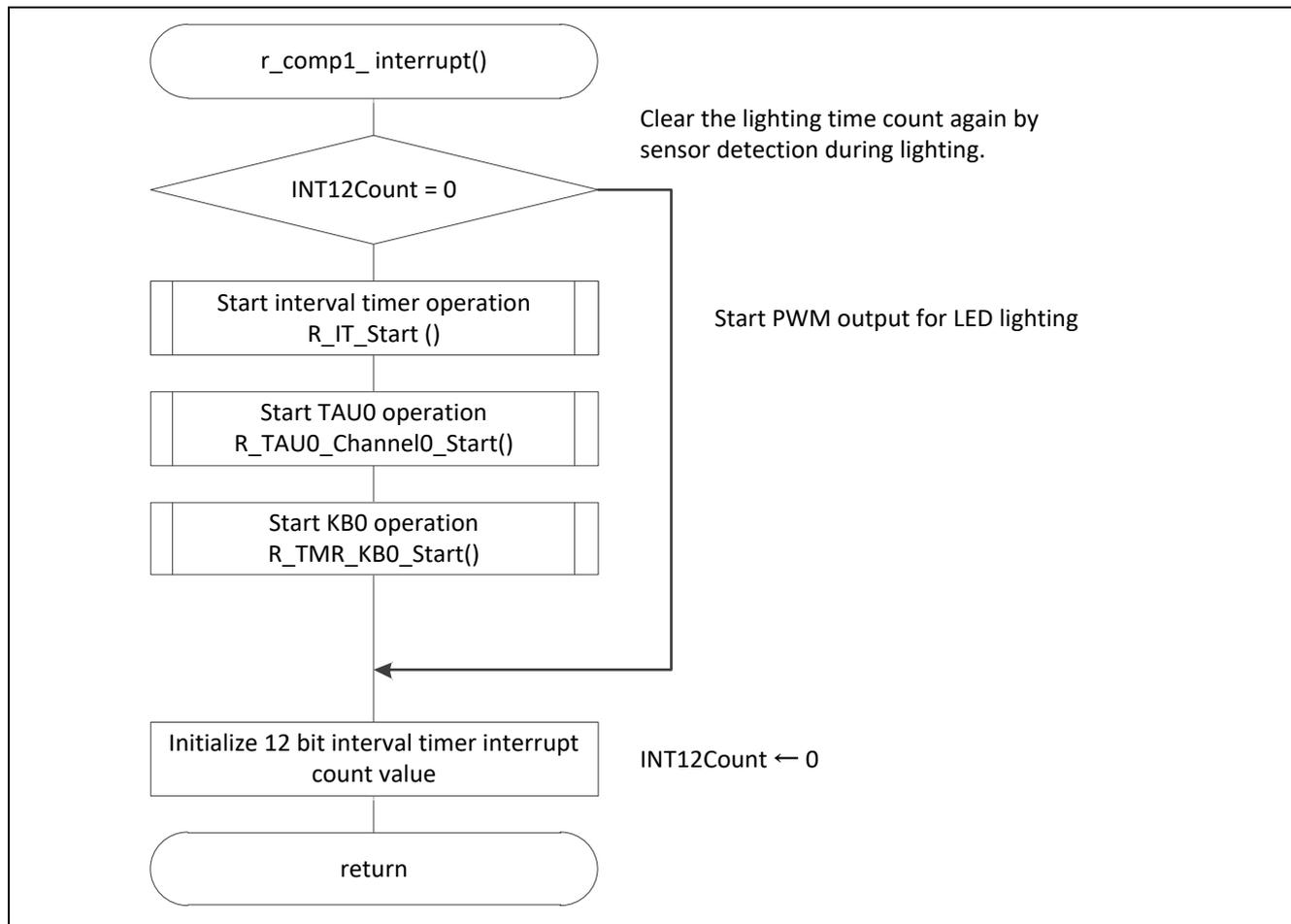
Figure 5.20 Comparator 1 Interrupt Operation
