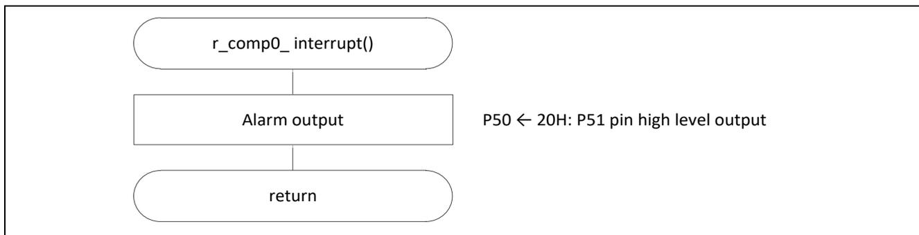
Figure 5.19 Comparator 0 Interrupt Operation
