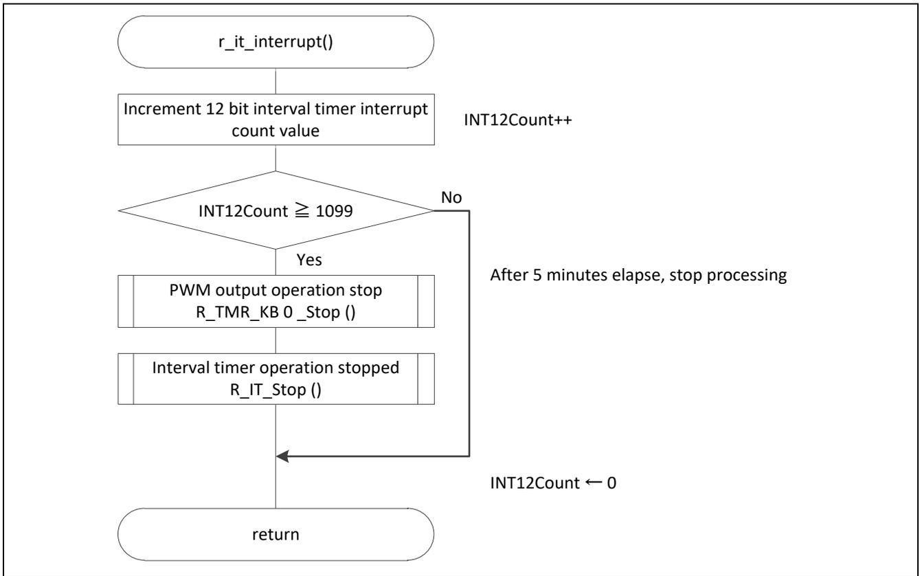
Figure 5.24 Starting Interval Timer Operation
