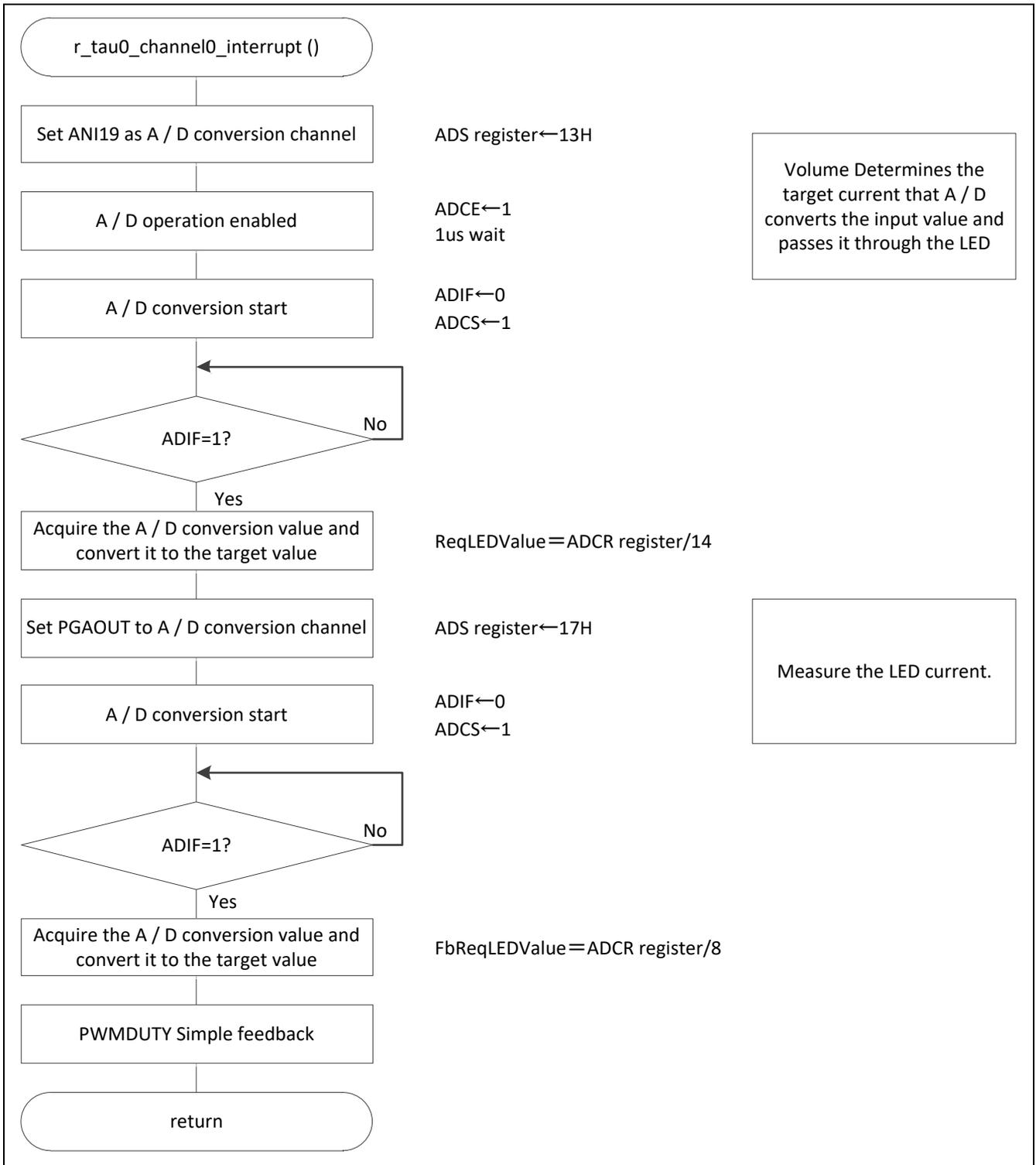
Figure 5.27 Timer Array Unit Interrupt Operation
