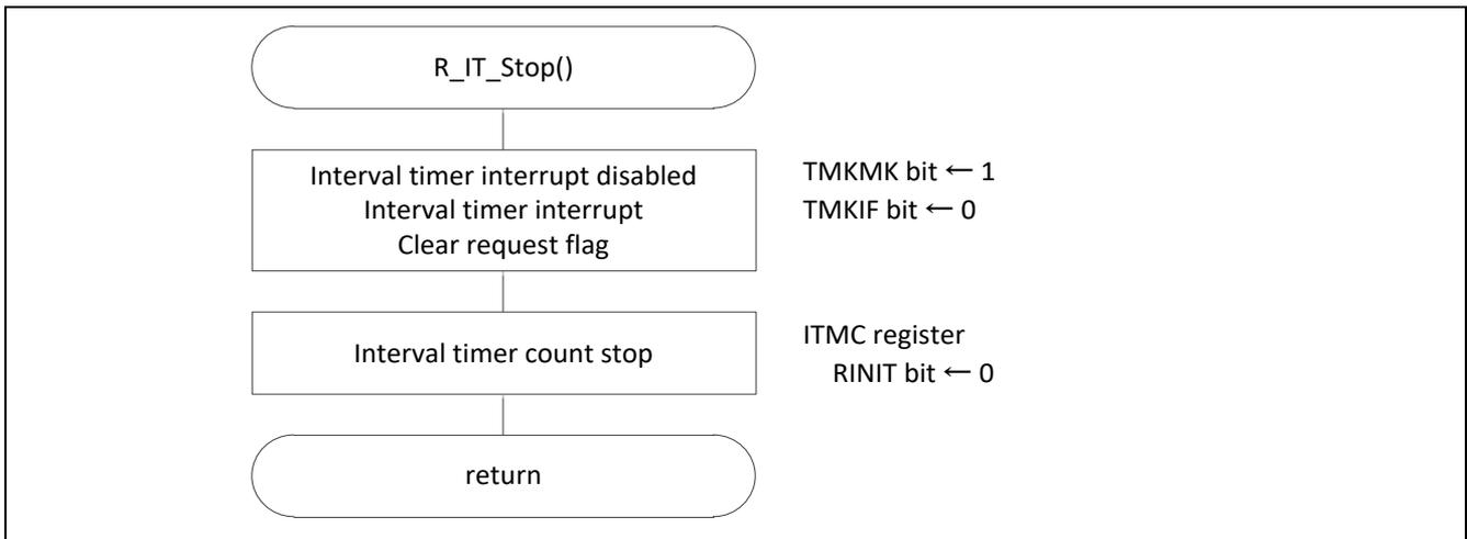
Figure 5.26 Stopping Interval Timer Operation
