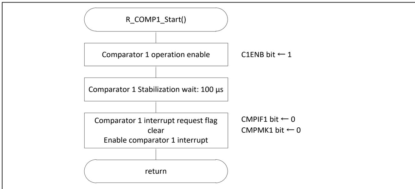
Figure 5.18 Starting Comparator 1 Operation
