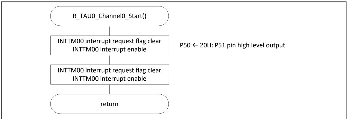
Figure 5.22 Starting Timer Array Unit Operation
