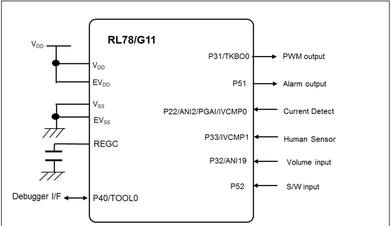
Figure 4.1 Hardware Configuration
