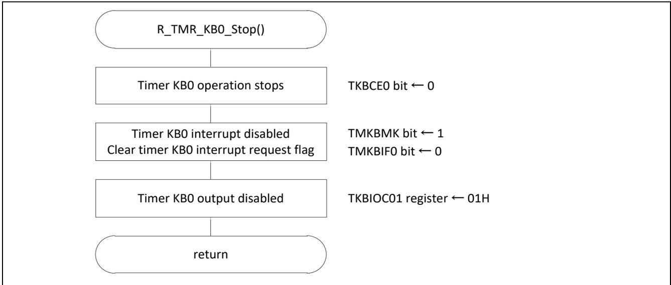
Figure 5.25 Stopping Timer KB0 Operation
