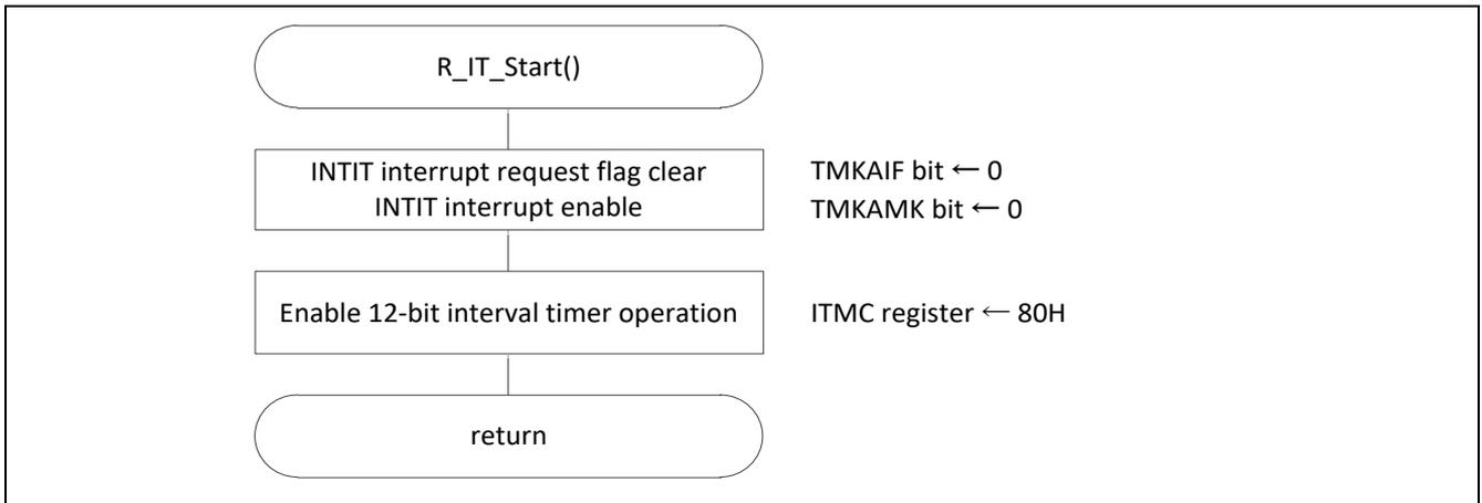
Figure 5.21 Starting Interval Timer Operation
