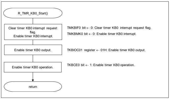
Figure 5.16 Timer KB0 Operation Starting Function
