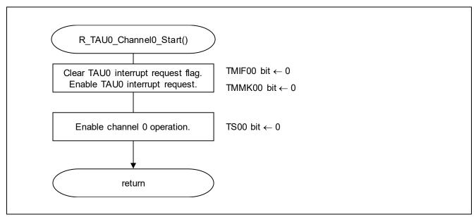
Figure 5.15 TAU0 Operation Starting Function
