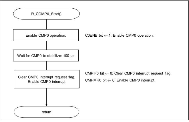
Figure 5.13 Comparator Operation Starting Function
