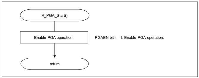
Figure 5.14 PGA Operation Starting Function
