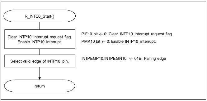
Figure 5.17 External Interrupt Operation Starting Function
