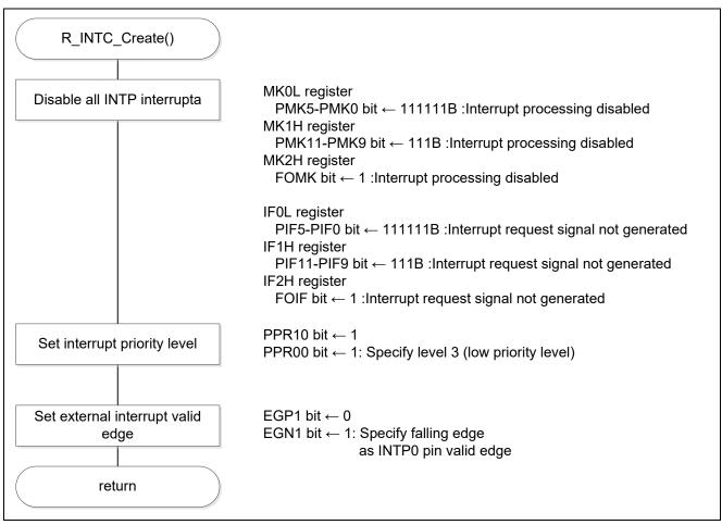
Figure 5.6 External Interrupt Setting
