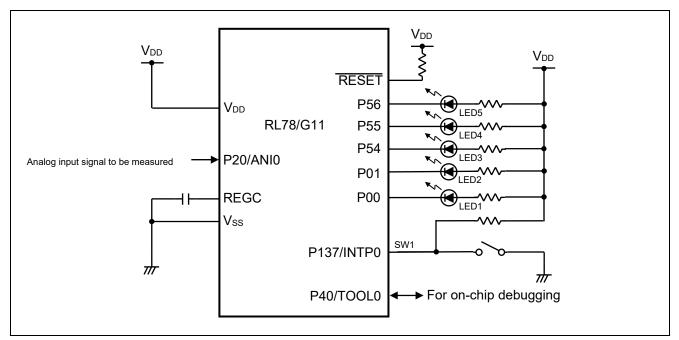
Figure 4.1 Hardware Configuration
