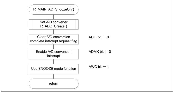
Figure 5.28 A/D Converter Setting
