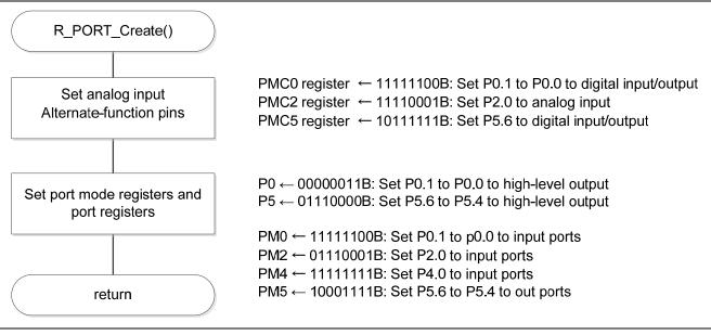
Figure 5.4 Input/Output Port Settings
