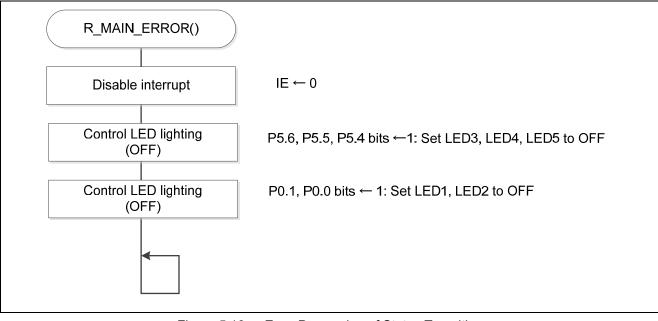
Figure 5.16 Error Processing of Status Transition
