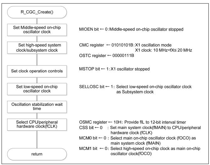
Figure 5.5 Clock Generator Setting
