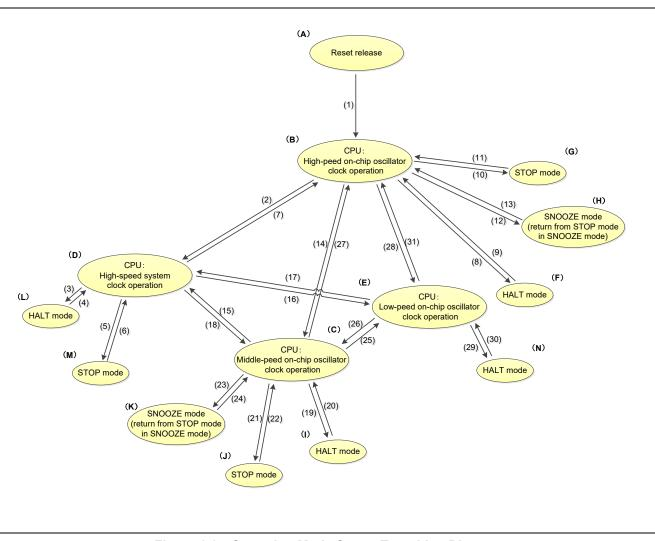
Figure 1.1 Operating Mode Status Transition Diagram
