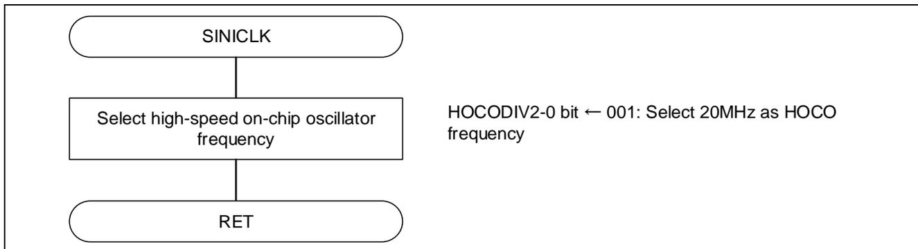
**Figure 5.5 Clock Oscillation Circuit Setting**
