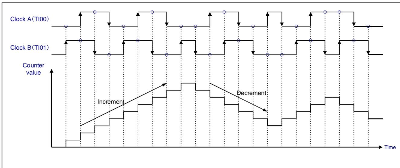
Figure 5.1 Phase Difference Detection Example
