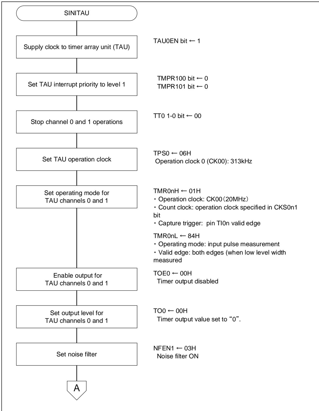
Figure 5.6 Timer Array Unit Setting (1/2)
