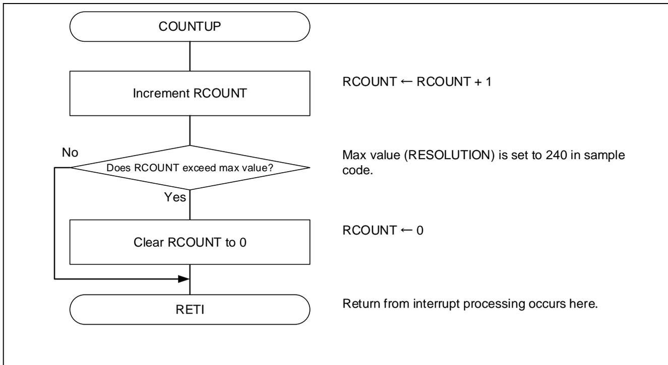
Figure 5.11 Interrupt Processing (count-up)
