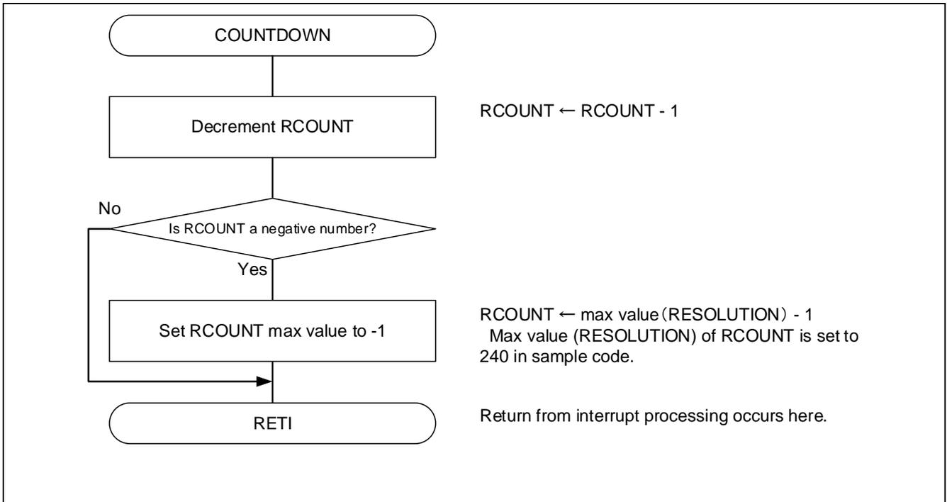
Figure 5.12 Interrupt Processing (count-down)
