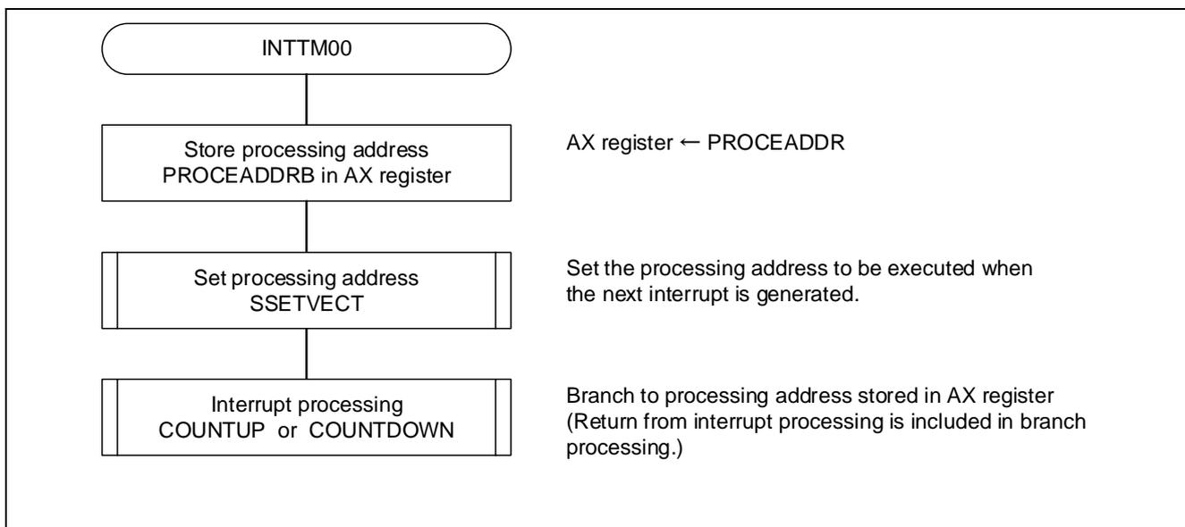
Figure 5.9 INTTM00 Interrupt Processing
