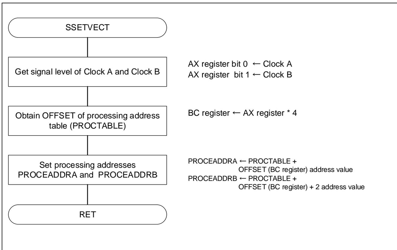
Figure 5.8 Interrupt Processing Address Setting
