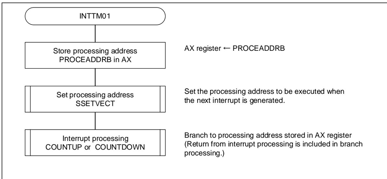
Figure 5.10 INTTM01 Interrupt Processing
