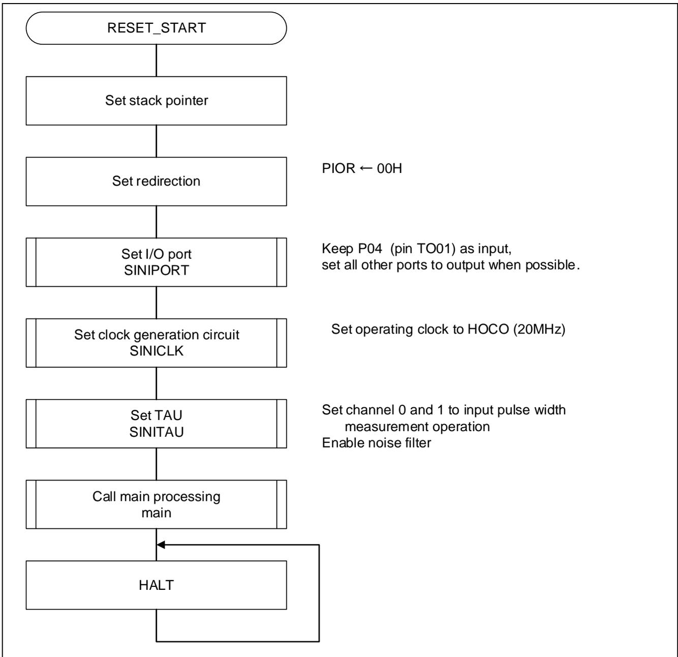
Figure 5.3 CPU Initialization Function
