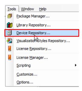
In the dialog box, click on the "Install" button to produce the dialog box where you are to enter the name of the provided GSDML file. Specify "GSDML-V2.31-Renesas-Template-20160520.xml". The result of installation will be indicated under the file name. An icon " \*\* appears in the case of normal installation, as is shown within the blue rectangle in the figure below.
