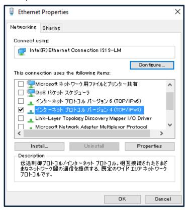
Select the radio button "Use the following IP Address" and set IP and subnet mask.
