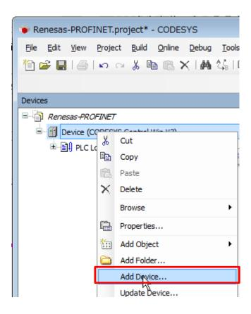
The "Add Device" dialog box opens. Select "Ethernet" under "Fieldbusses", "Profinet IO", then "Ethernet Adapter" and click on the "Add Device" button.
