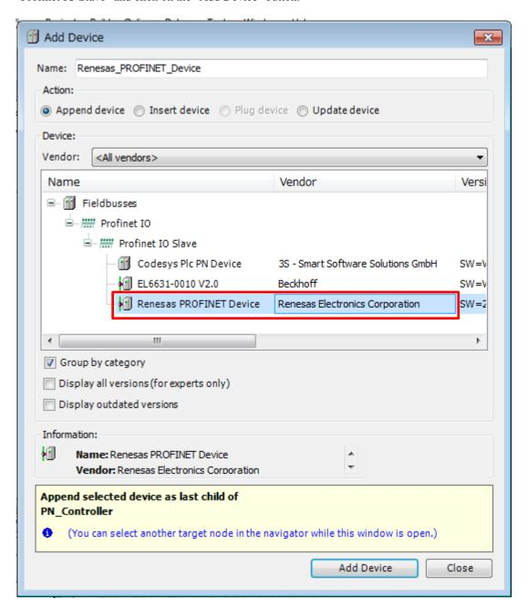
You can see that "Renesas\_PROFINET\_Device" has been added under "PN-Controller" in the "Device" tree.
