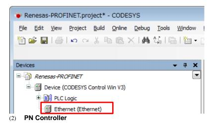
Right-click on "Ethernet(Ethernet)" in the "Device" tree and select "Add Device".
