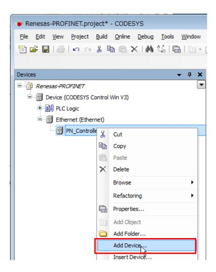
The "Add Device" dialog box opens. Select "Renesas\_PROFINET\_Device" under "Fieldbusses", "Profinet IO", then "Profinet IO Slave" and click on the "Add Device" button.
