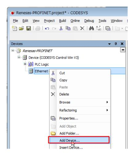
The "Add Device" dialog box opens. Select "PN-Controller" under "Fieldbusses", "Profinet IO", then "Profinet IO Master" and click on the "Add Device" button.
