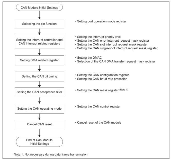
Figure 4.2.1 CAN Module Initial Setting
