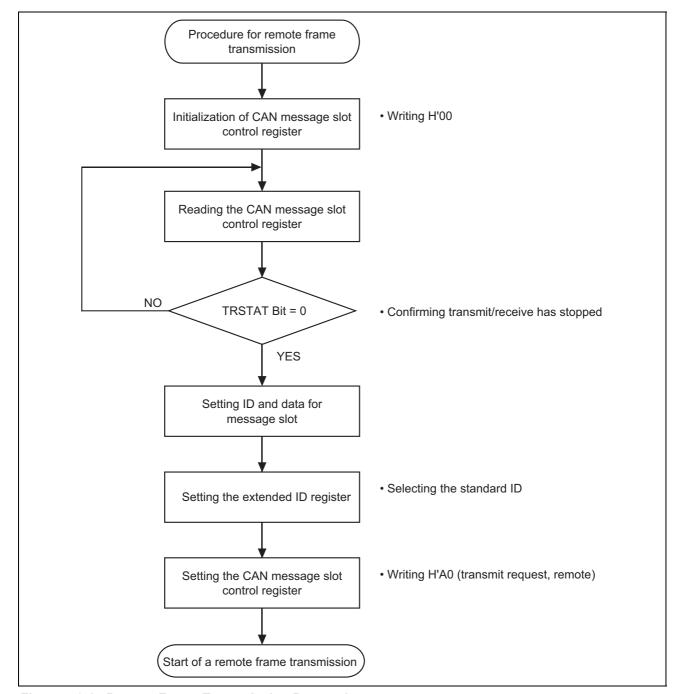
Figure 4.3.1 Remote Frame Transmission Processing
