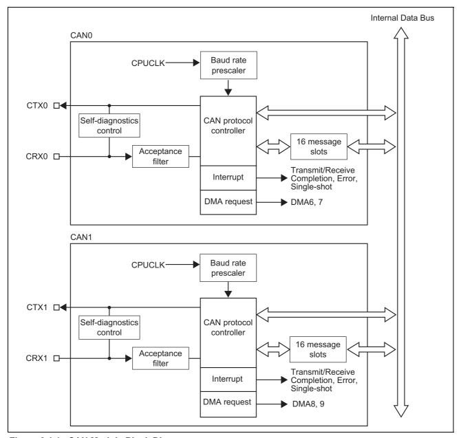
Figure 3.1.1 CAN Module Block Diagram
