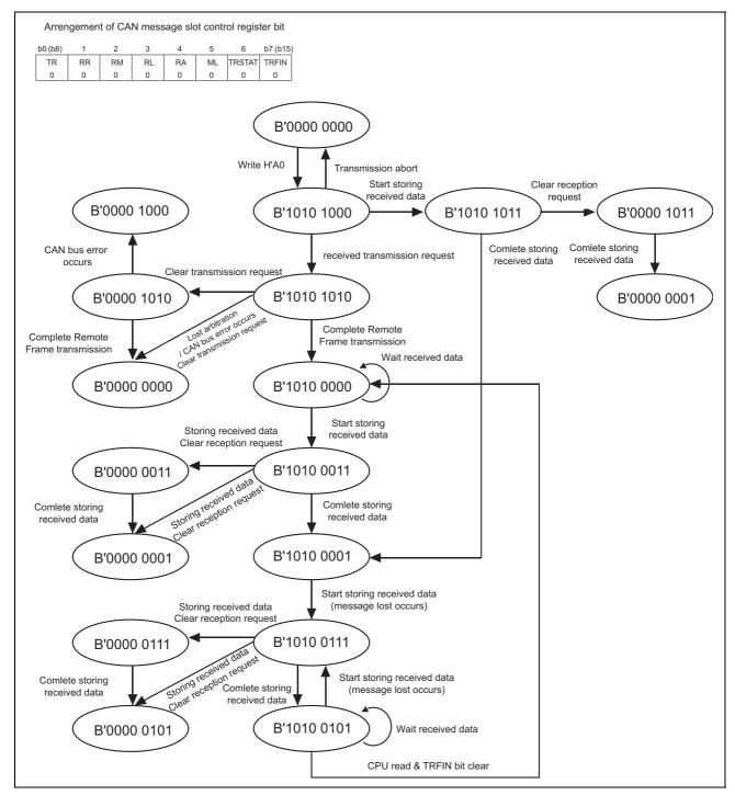
Figure 4.4.1 The State of CAN Message Slot Control Registers during Remote Frame Transmission
