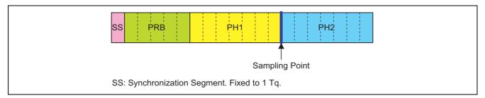
Figure 4.5.1 Bit Timing
