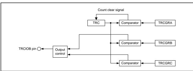
Figure 3.1 Block Diagram
