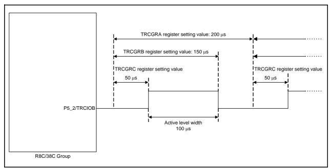
Figure 3.2 Timing Diagram
