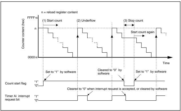
Figure 1. Operation timing of timer mode
