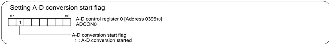
Repeatedly carries out A-D conversion on pins selected through the A-D sweep pin select bit. **Start A-D conversion**
