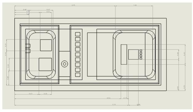
Figure 3. Optical Element Locations within the Package
