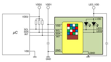
Figure 1. Application Circuit
