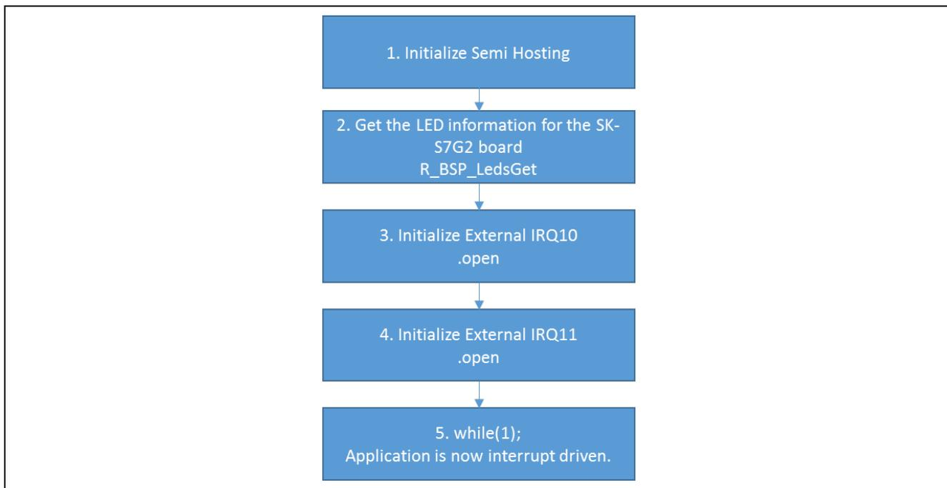
**Figure 4 External IRQ HAL Module Application Project Flow Diagram**
