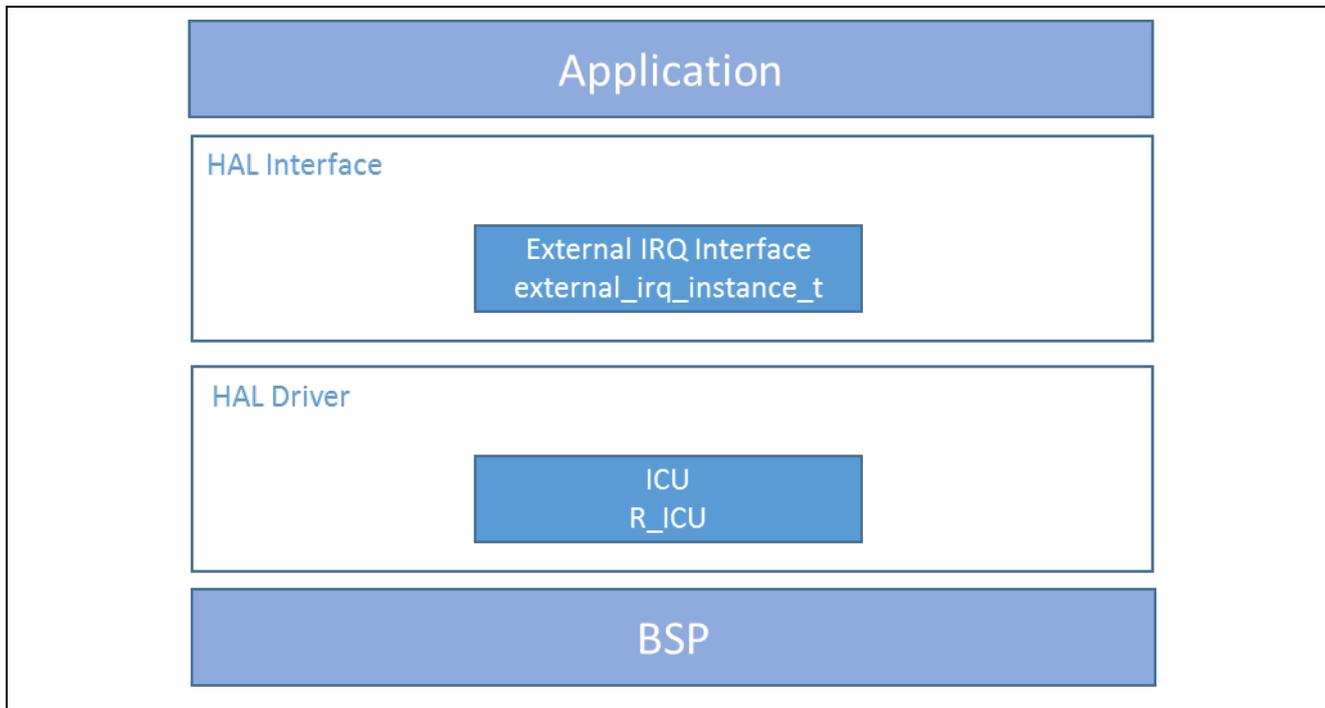
Figure 1 External IRQ HAL Module Block Diagram
