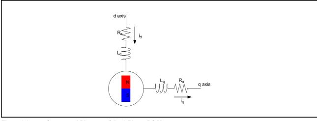
Figure 3.2 Conceptual Diagram of the 2-Phase DC Motor
