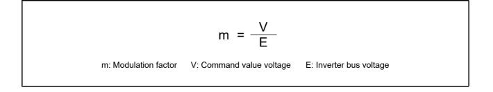
Desired control is performed by reflecting this modulation factor in the register that determines the PWM duty.
