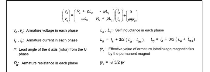
It can be considered here that the alternating current that was flowing through the quiescent 3-phase stator appears as the direct current in the 2-phase stator that is rotating in synchronization with the permanent magnet (rotor).
