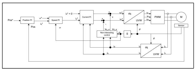
Figure 3.3 Control Flow of Vector Control (Position Control)
