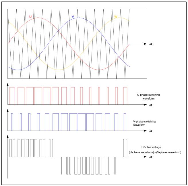
Figure 3.7 Conceptual Diagram of the Triangular Wave Comparison Method
