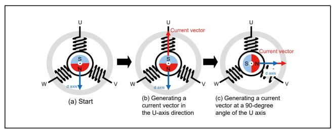
Figure 3.4 Determining the Position of the Permanent Magnet
