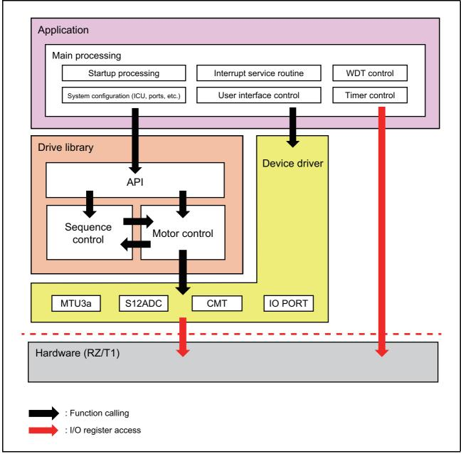
Figure 2.2 Module Configuration of the Sample Program
