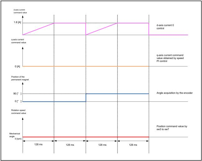
Figure 3.5 Motor Start Control
