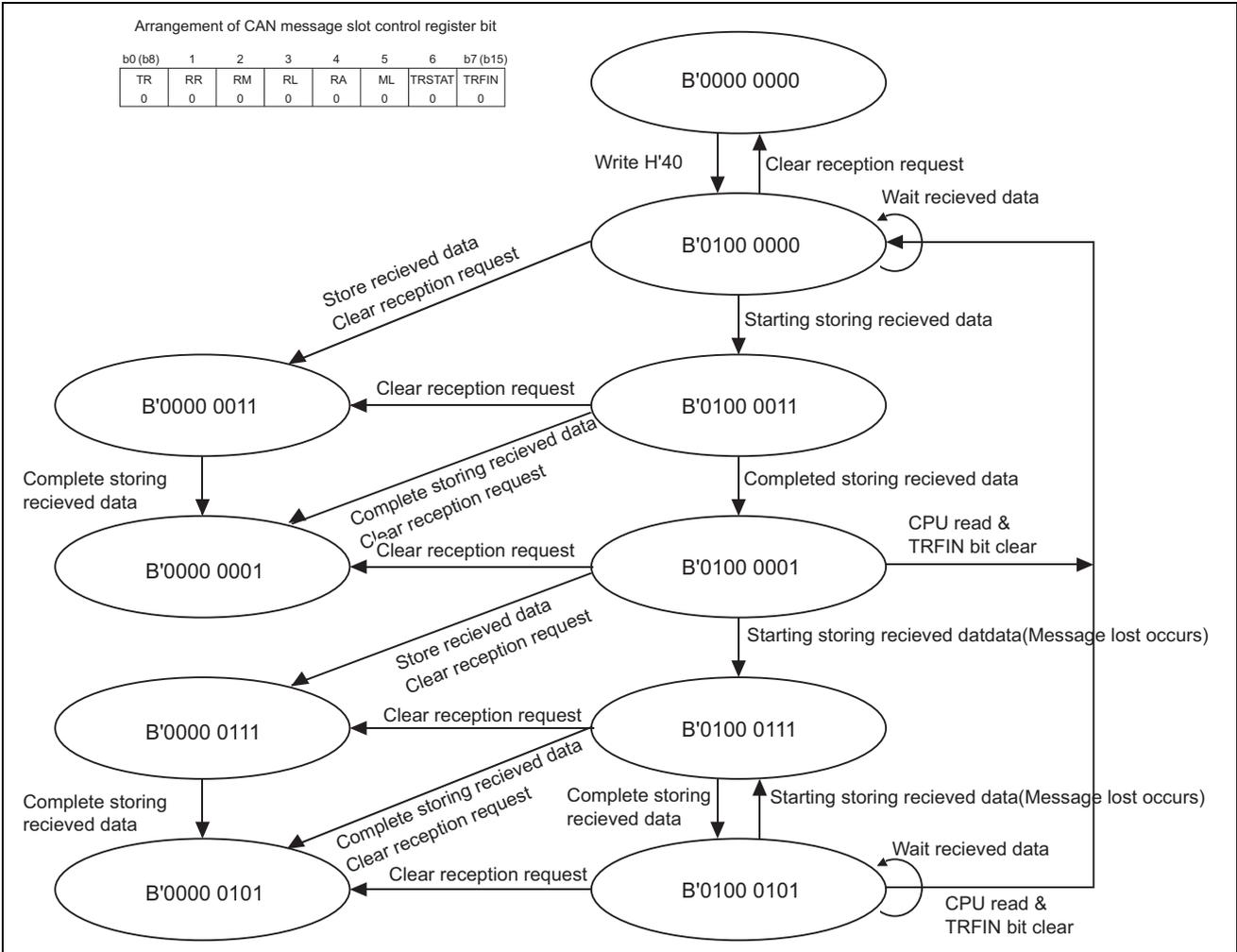
Figure 4.4.1 The State of CAN Message Slot Control Registers during Data Frame Reception
