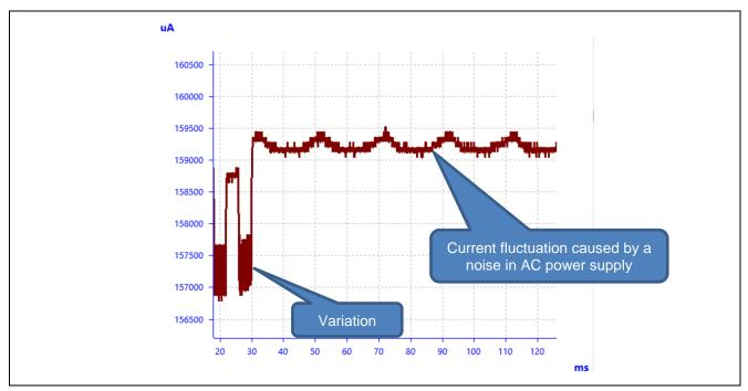
Figure 5-5 Characteristics of Measurement Result of Current Consumption
