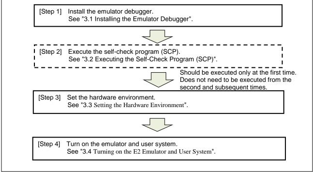
Figure 3-1 Setup Procedure
