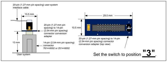
Figure 3-4 Connecting the User-System Interface Cable to the 14-Pin Connector
