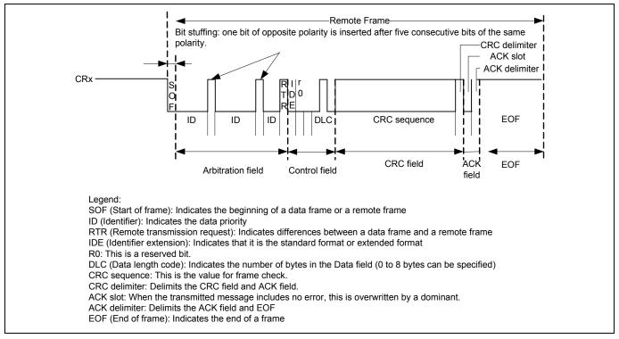
**Figure 5 CAN Reception Waveform**
