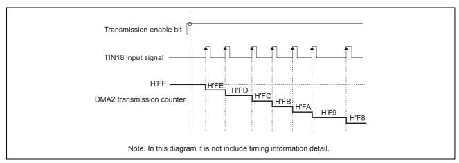
Figure 3.4.1 Timing Diagram for combination sample of input pin and DMAC
