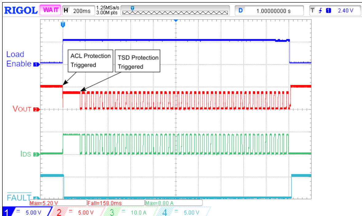
Figure 17: Two SLG59M1714Vs Operating in Parallel: ACL with thermal protection operation; V_{DD} = 5\text{ V} , V_{IN} = 5\text{ V} , I_{ACL} = 8\text{ A} , R_{SET\_U1} = 20\text{ k}\Omega , R_{SET\_U2} = 20\text{ k}\Omega , R_{LOAD} = 0.6\ \Omega , C_{LOAD} = 10\ \mu\text{F} , ON = HIGH
